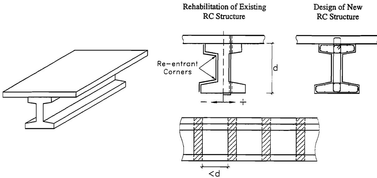
Figure 3: Design detailing for Shear Strengthening of I-Beams
