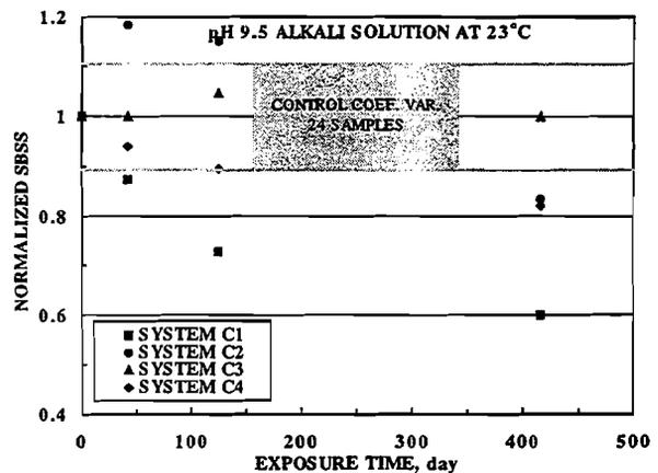
Fig. 4--Normalized short beam shear strength for systems C1, C2, C3, and C4 as functions of exposure time in pH 9.5 alkali solution at  $23^\circ\text{C}$  ( $73^\circ\text{F}$ ).
