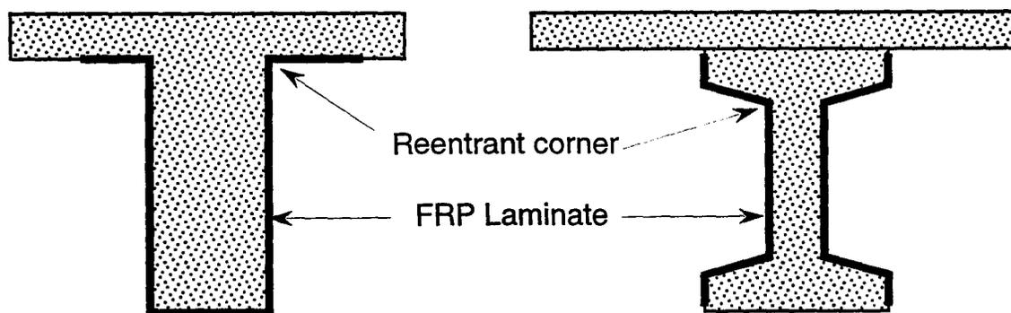
Fig. 2—External shear strengthening of T- and I-beams
