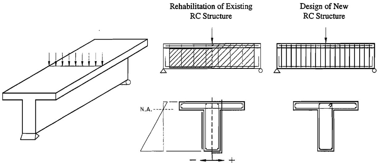
Figure 2: Design detailing for Shear Strengthening of T-Beams
