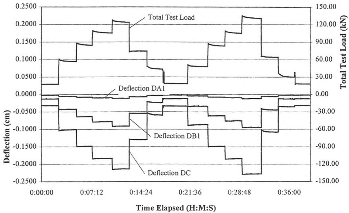
**Figure 6: Sample load and deflection history data for two load cycles**
