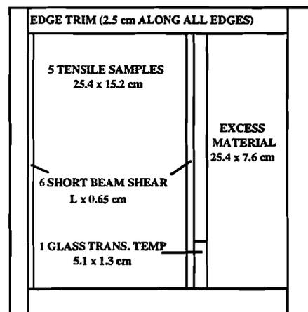
Fig. 1-- Lay-out for cutting samples from a 30 cm x 30 cm composite durability panel
