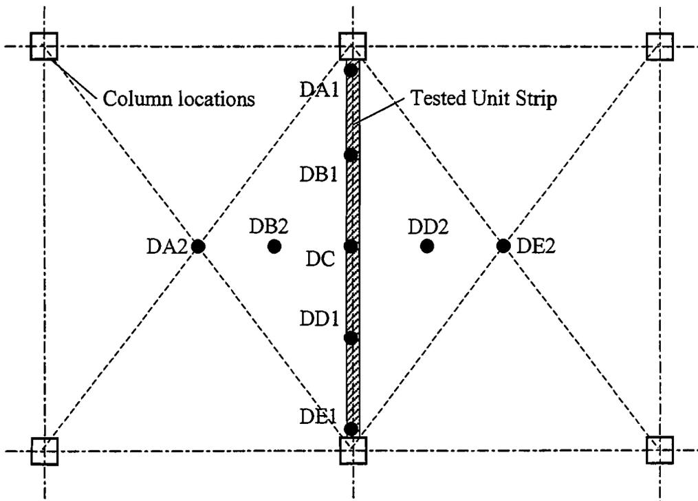
**Figure 4: Typical location of instruments to measure deflections**
