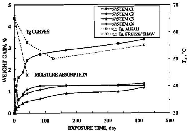
Fig. 5--Moisture absorption and glass transition temperature for systems C1, C2, C3, and C4 as functions of exposure time in pH 9.5 alkali solution at 23 °C (73 °F).
