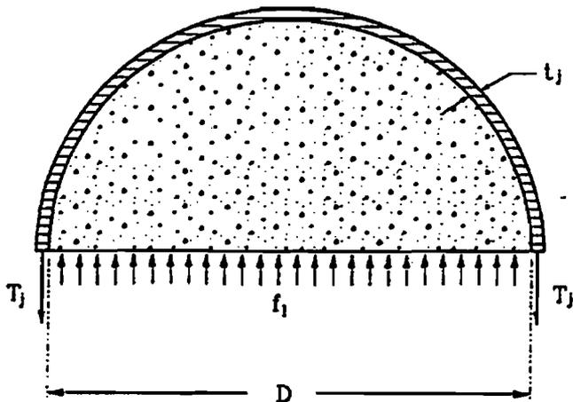
FIG. 12 Confinement of Circular Column by Passive Jacket
