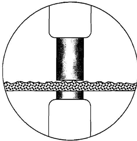
Figure 3: Illustration of Thickness Measurement Error with Cored Casing Sample.
