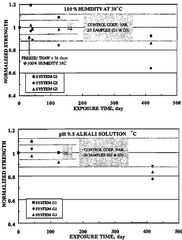
Fig. 2--Normalized tensile strength for systems G1, G2, and G3 as functions of exposure time in 100 % humidity at 38 °C (100 °F) or pH 9.5 alkali solution at 23 °C (73 °F).
