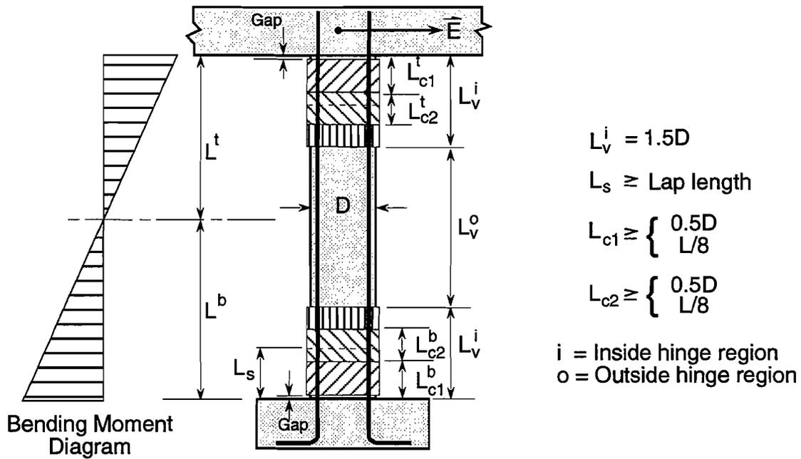
**FIG. 6. Carbon Jacket Regions for Bridge Columns Retrofit, Double Bending**
