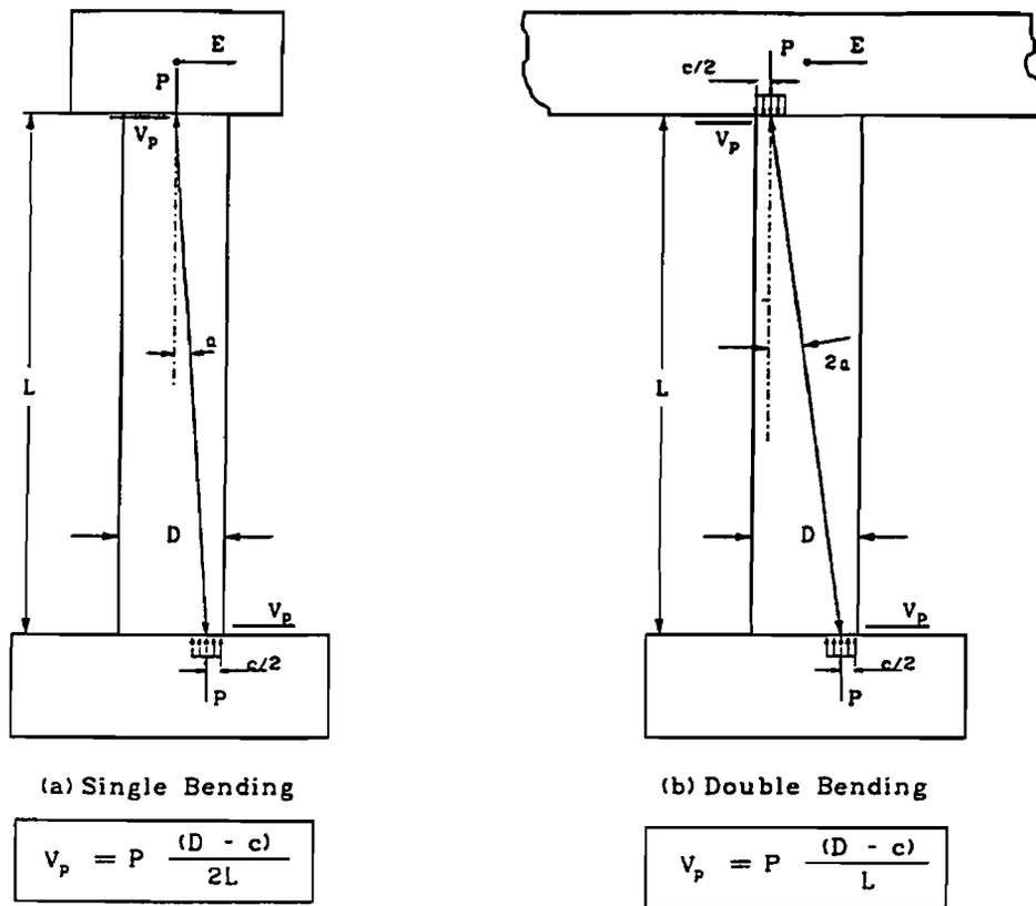
FIG. 9. Axial Force Shear Contribution
