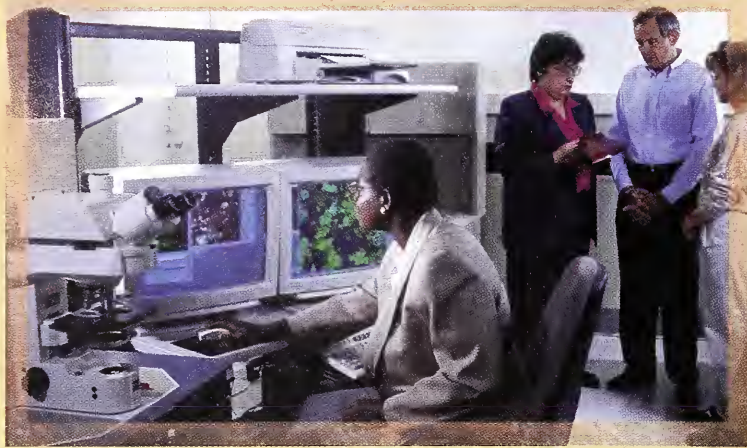
F. Hunt inspects a scanning electron microscope (SEM) image of the microstructure of a metallic paint used in automobile coatings. M. McKnight (BFRL), T. Vorburger (MEL), and M. Nadal (PL) discuss a piece of an automobile from which the SEM sample was taken. The project combines optical and microstructural measurements as part of a multi-laboratory effort to develop measurement sciences for optical reflectance and scattering. (1)
