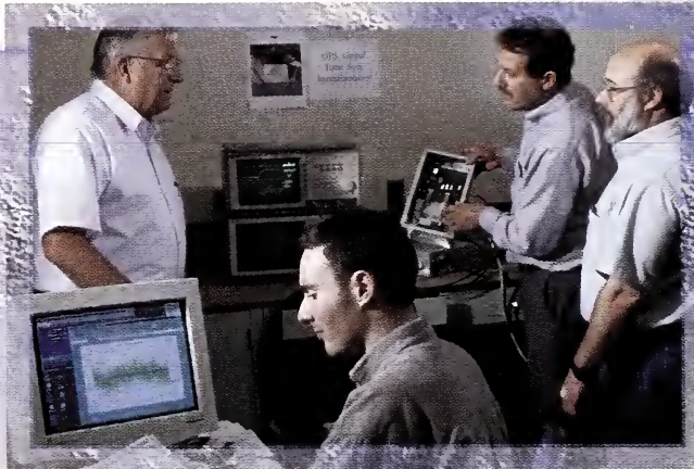
B. Hershman adjusts a sensor connection on the NIST GPS time synchronization printed circuit board as directed by A. Mink, R. Carpenter adjusts the oscilloscope tracing the GPS time synchronization pulse and the NIST "trained" time synchronization pulse, and M. Courson plots the time synchronization stability of the NIST GPS "trained" oscillator feeding the NIST MultiKron board which is plugged into a local computer. (25)
