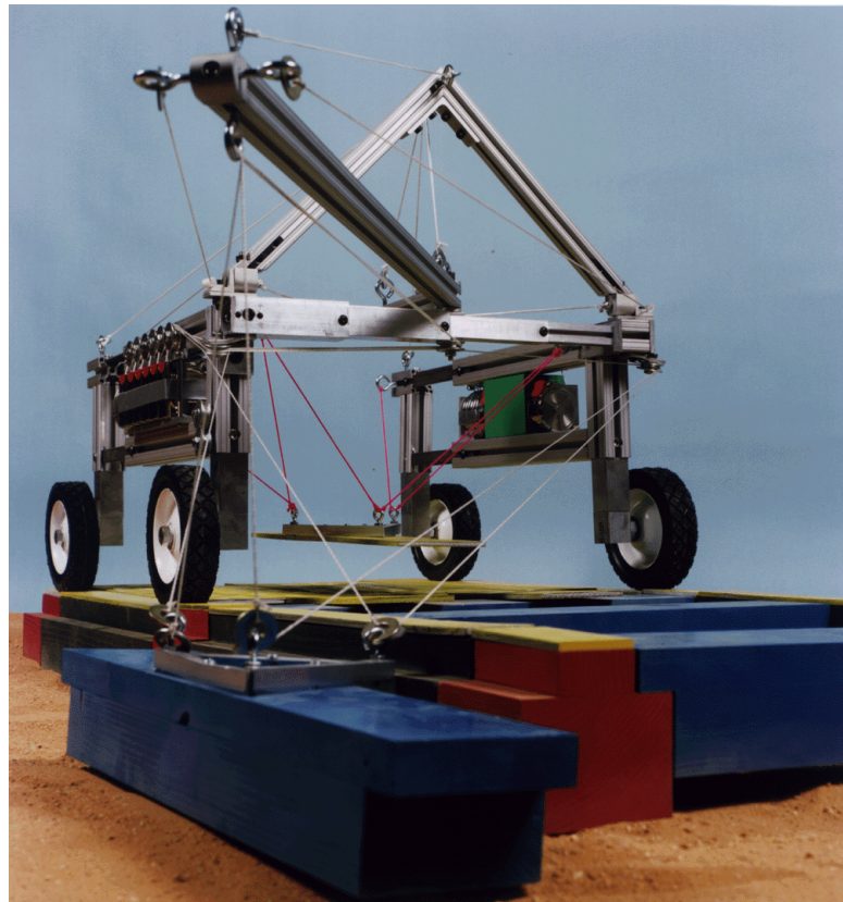
FIGURE 17. ATEC - Cantilevered Material Handler
