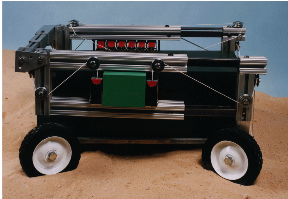
1/12th Scale Model of the ATEC - Container Mobilizer
