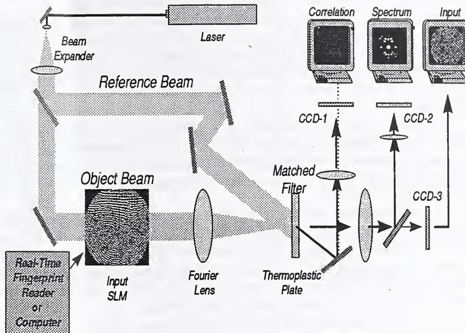
Figure 1: Diagram of the optical pattern recognition system
