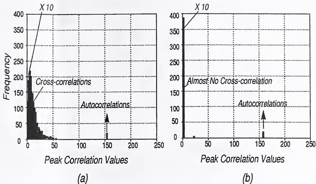
Figure 2: Histograms of peak correlations for gray (a) and binary (b) fingerprint images.
