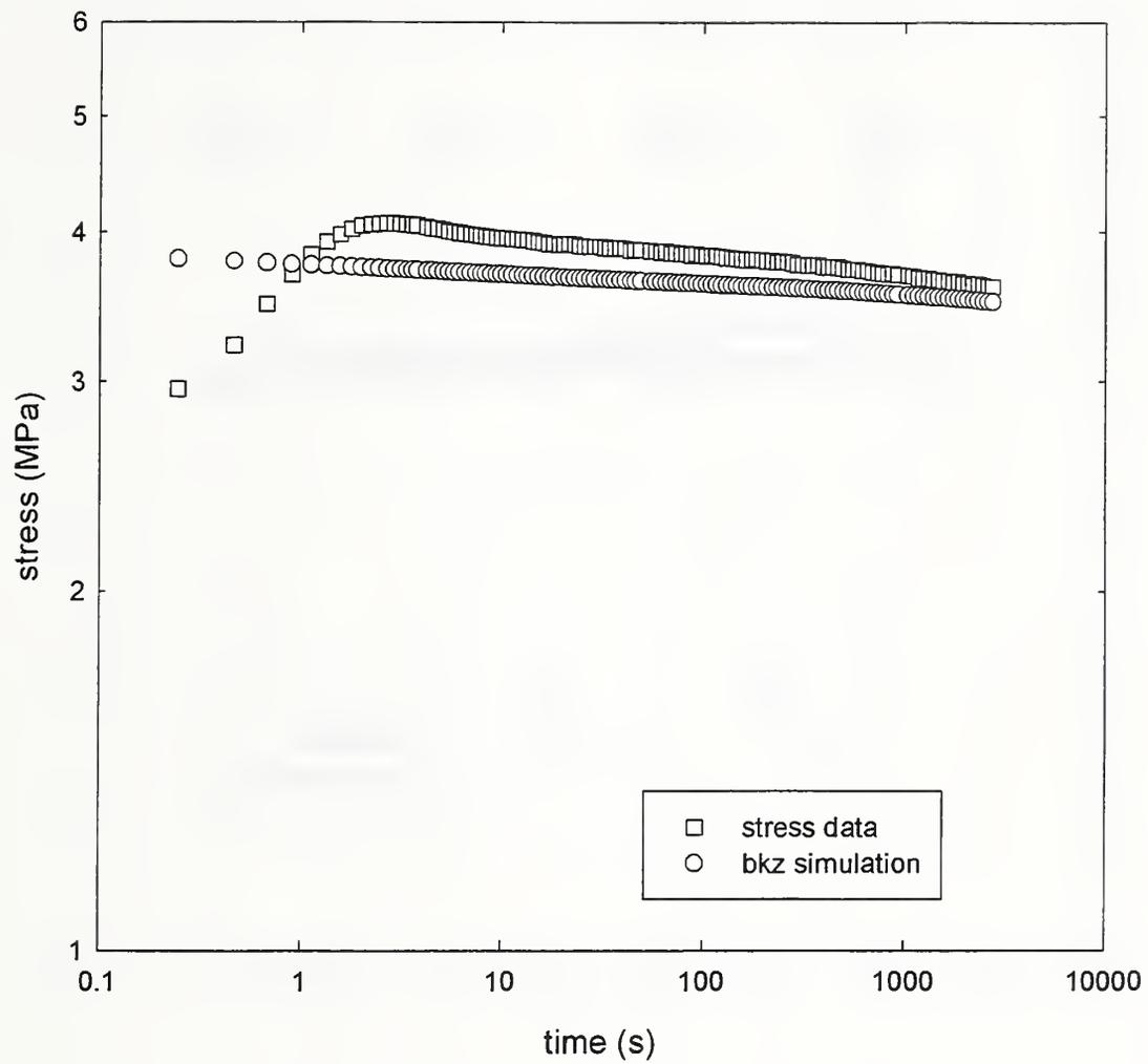
Figure 10: Log(stress) vs Log(time) curve for a multiple step-up stress relaxation experiment.
