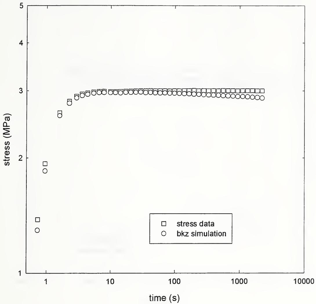
Figure 16: Log(stress) vs Log(time) curve for a multiple step-up creep experiment.
