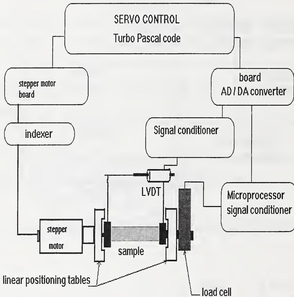
Figure 2. Schematic of Control System for Stepper Motor. (See text.)
