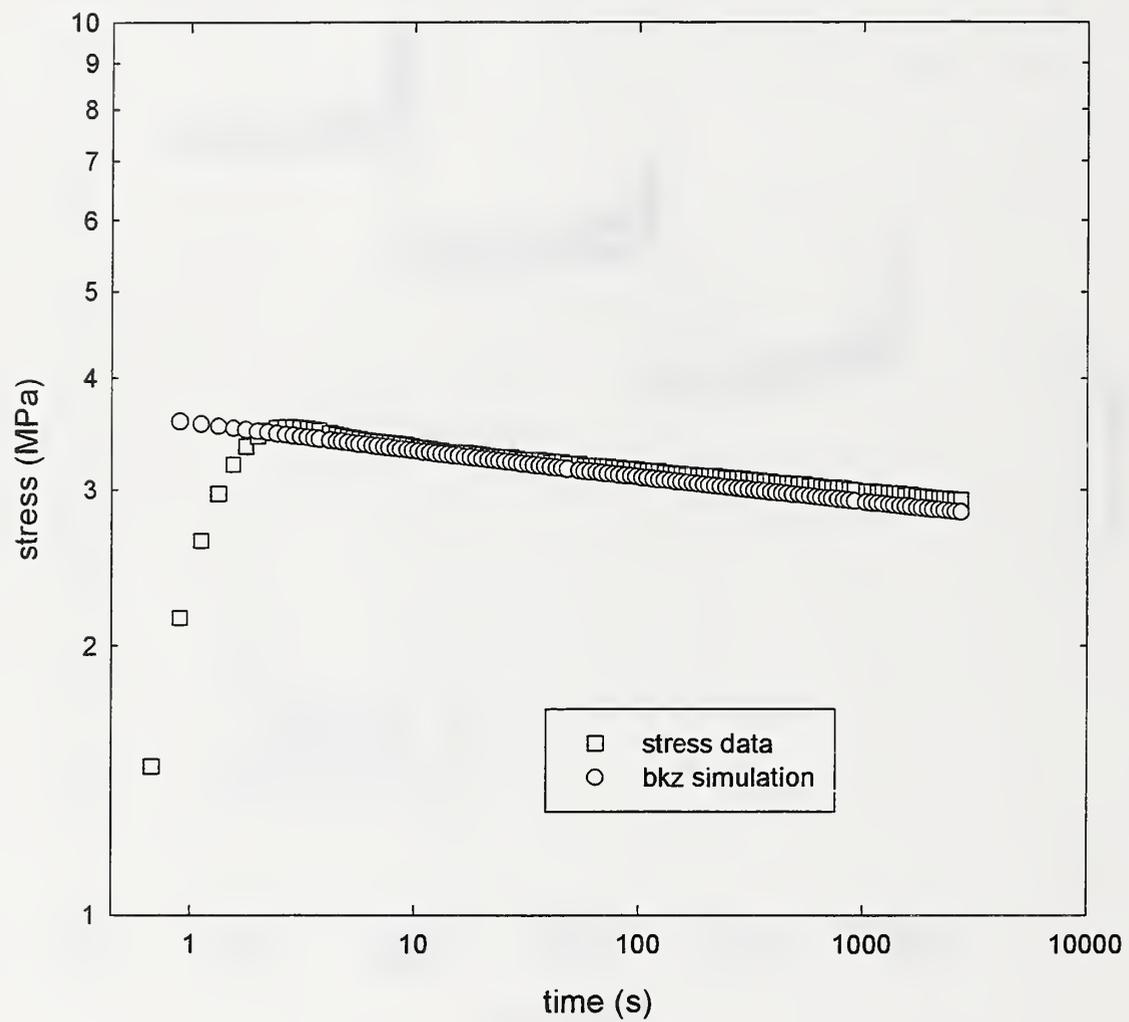
Figure 9: Log(stress) vs Log(time) curve for a multiple step stress relaxation experiment.
