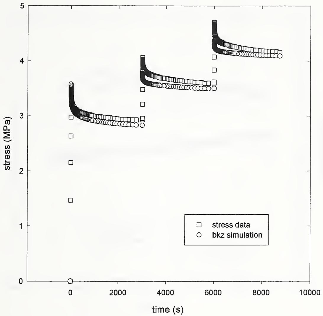
Figure 8: Stress versus time curve for a multiple step-up stress relaxation experiment  $T=50^{\circ}\text{C}$ .
