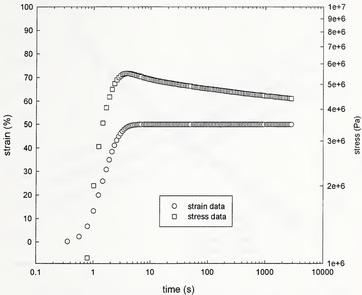
Figure 3a: Typical strain (left) and stress (right) versus time curves for a single step stress relaxation test on a polyurethane elastomer.
