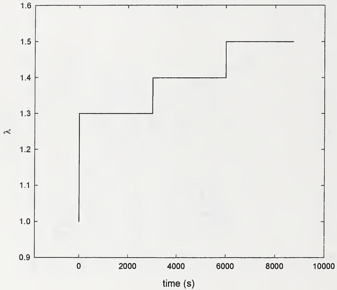
Figure 7: Strain versus time curve for a multiple step-up stress relaxation experiment.  $T=50^{\circ}\text{C}$ .
