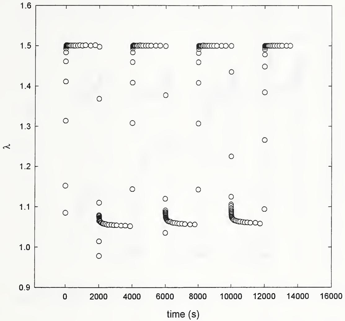
Figure 12: Strain versus time curve for a multiple stress relaxation cycle history.  $T=10^{\circ}\text{C}$ .
