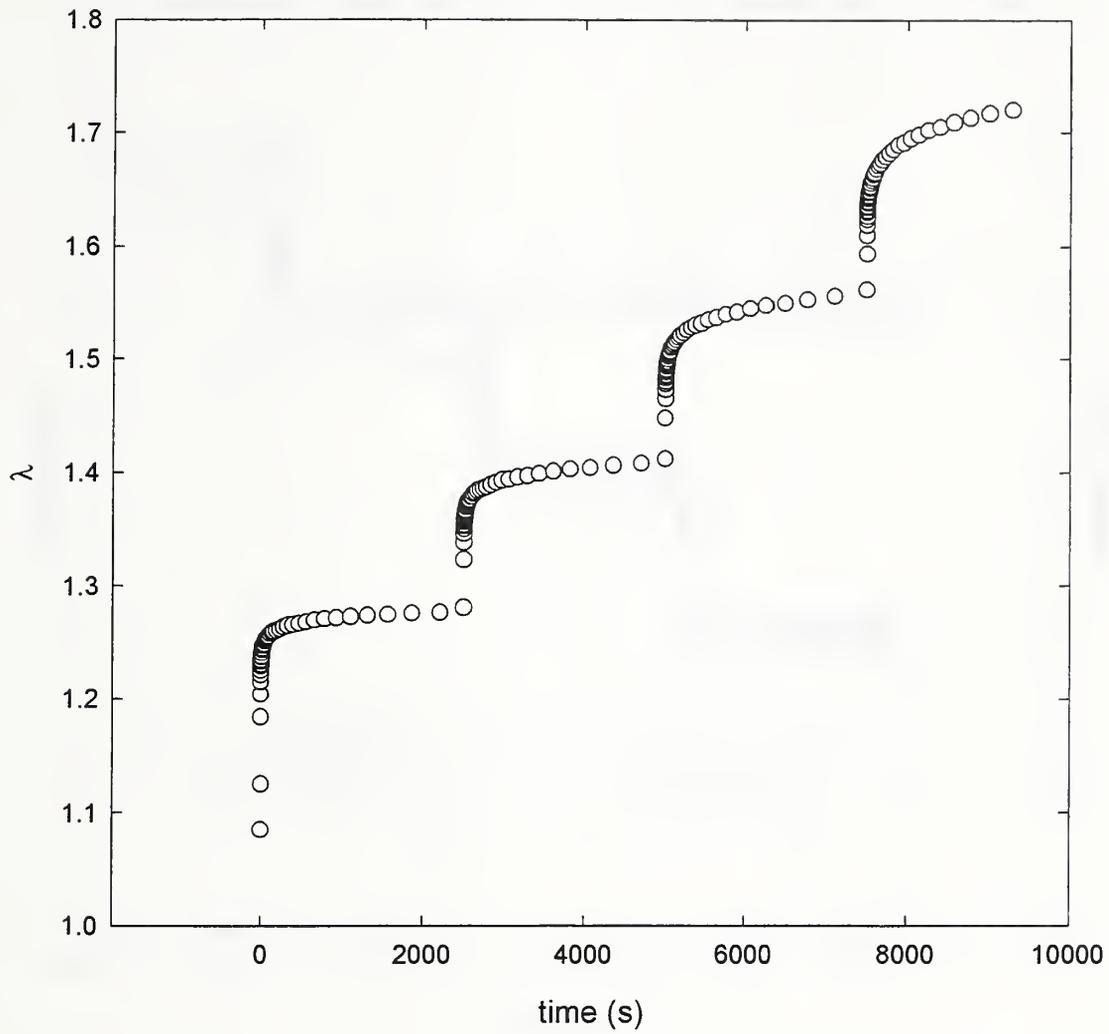
Figure 14: Strain versus time curve for a multiple step-up creep experiment.  $T=10^{\circ}\text{C}$ .
