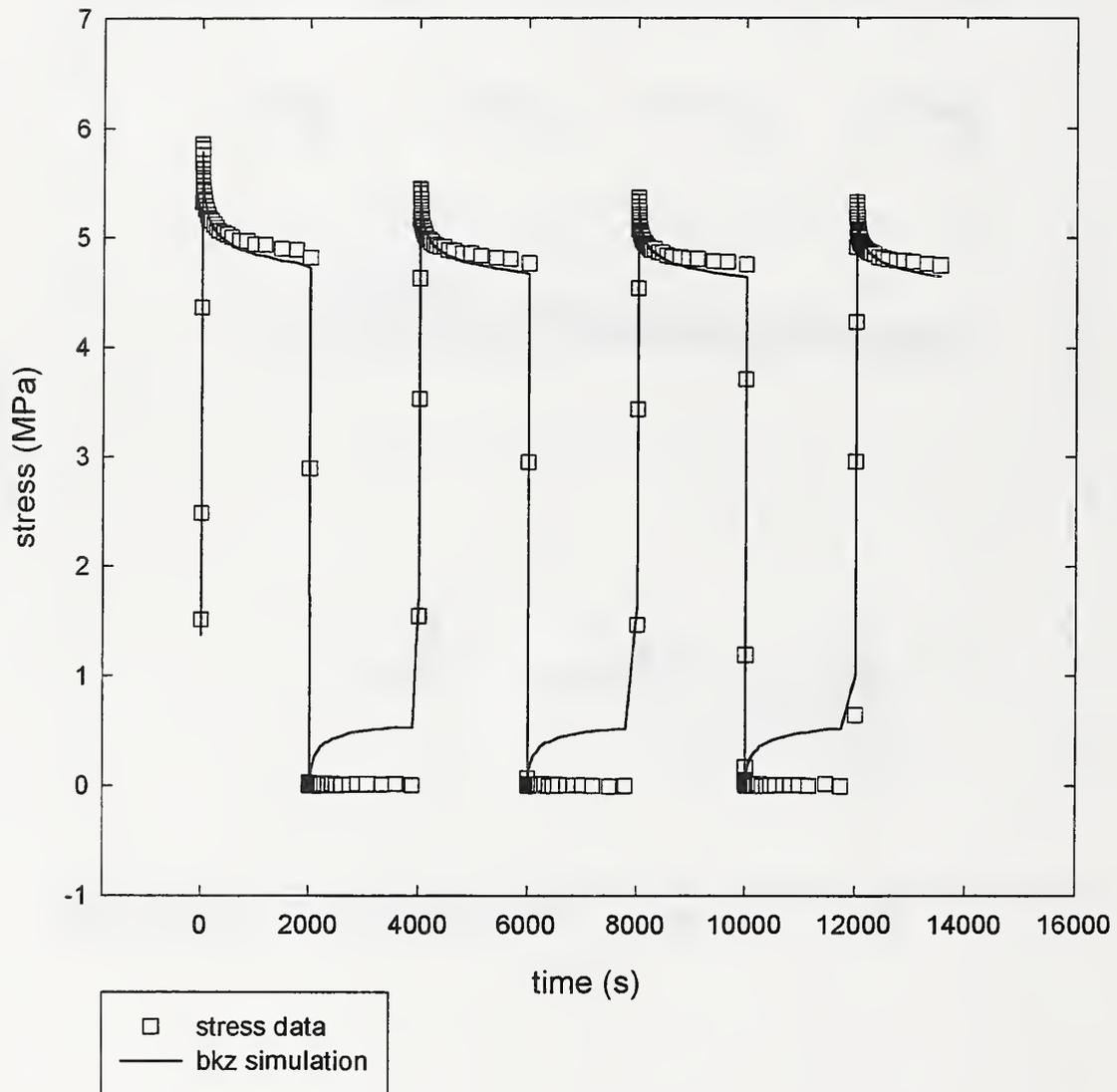
Figure 13: Stress versus time curve for the material response to multiple stress relaxation cycles.
