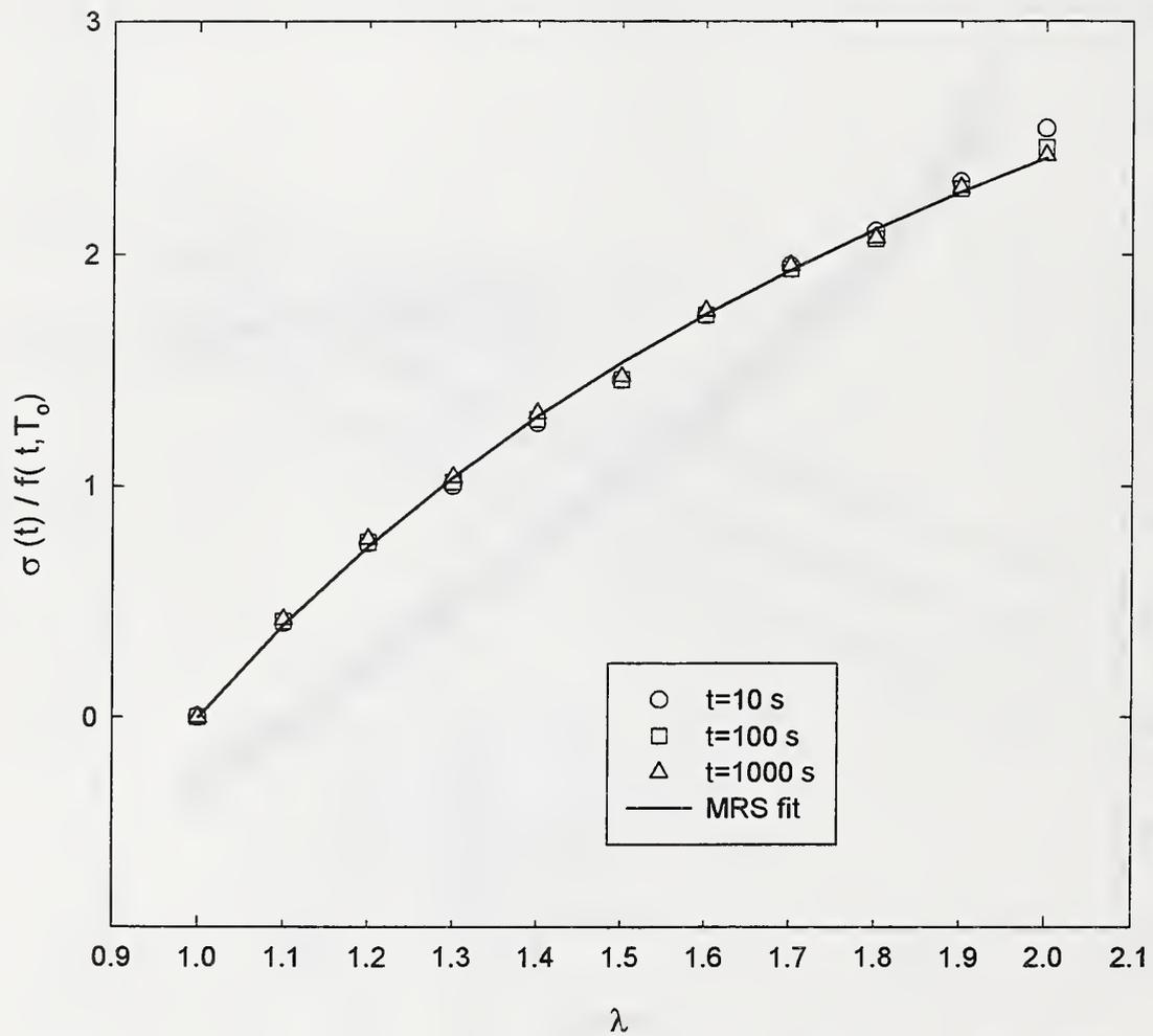
Figure 5: Comparison of normalized stress function vs deformation in tension with curve fit response given for the MRS equation.  $T_0=10^\circ\text{C}$ .
