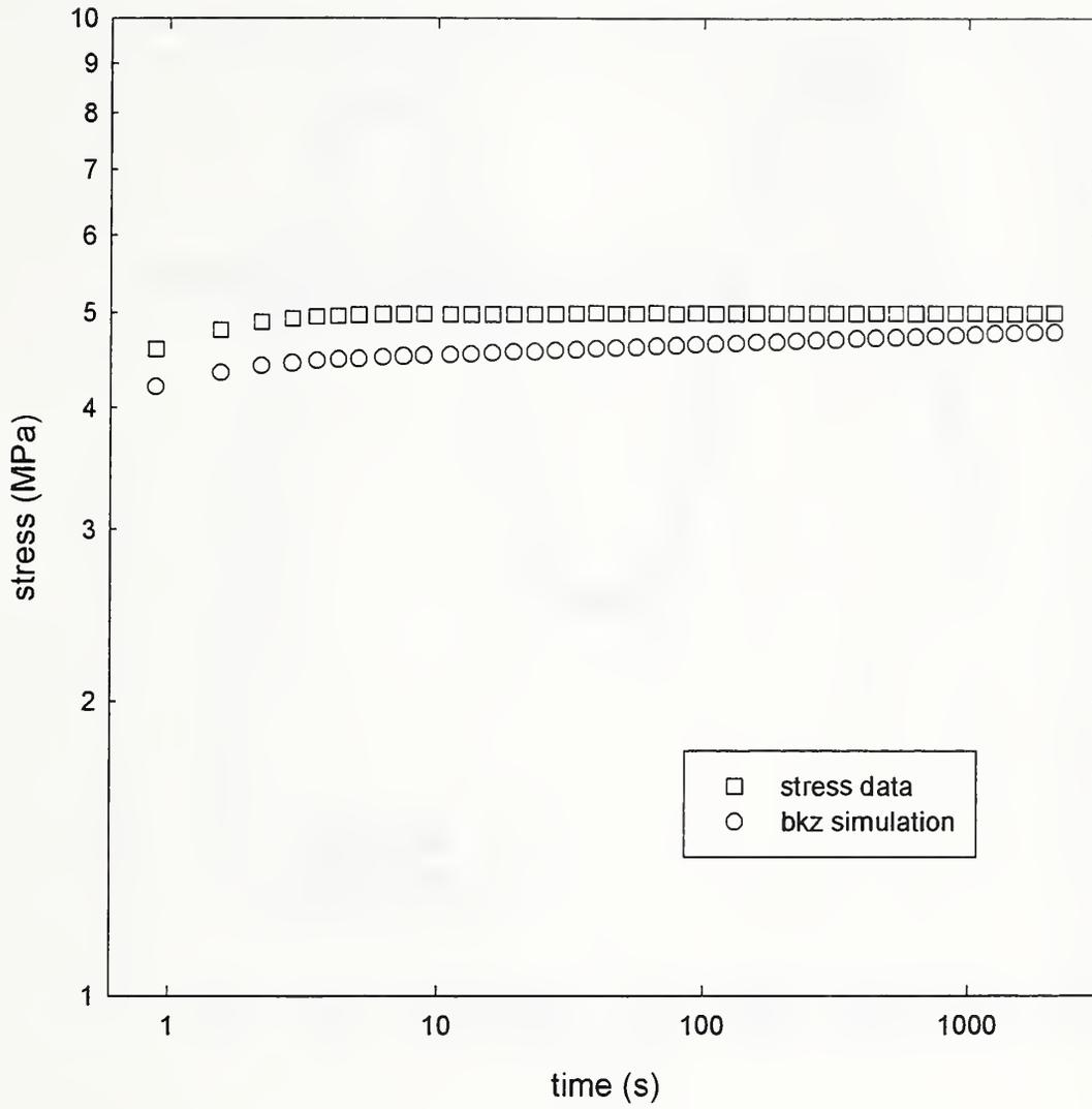
Figure 18: Log(stress) vs Log(time) curve for a multiple step-up creep experiment.
