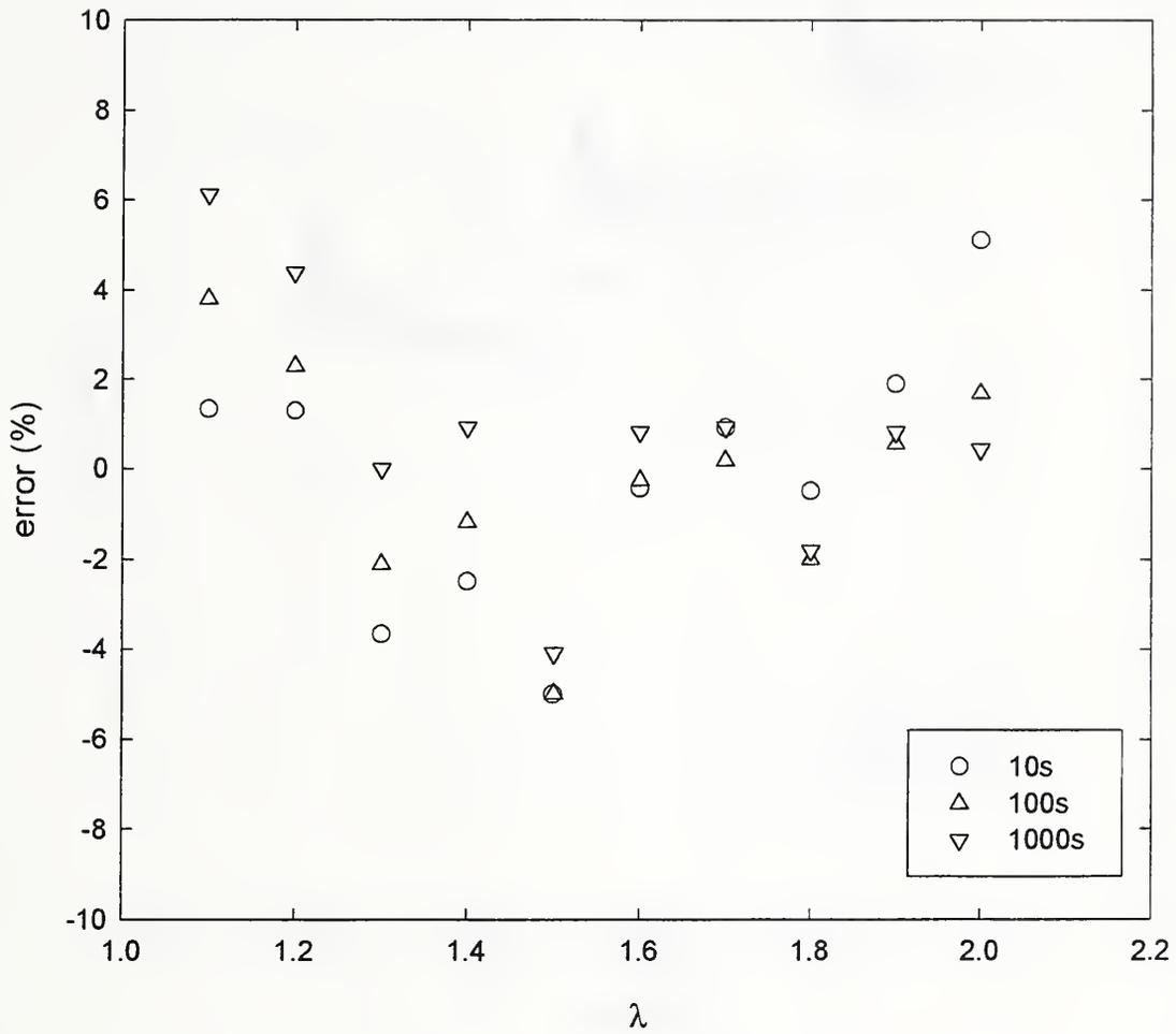
Figure 6: Residuals between normalized stress function (see text) and the MRS curve fit. Data are from Figure 5.
