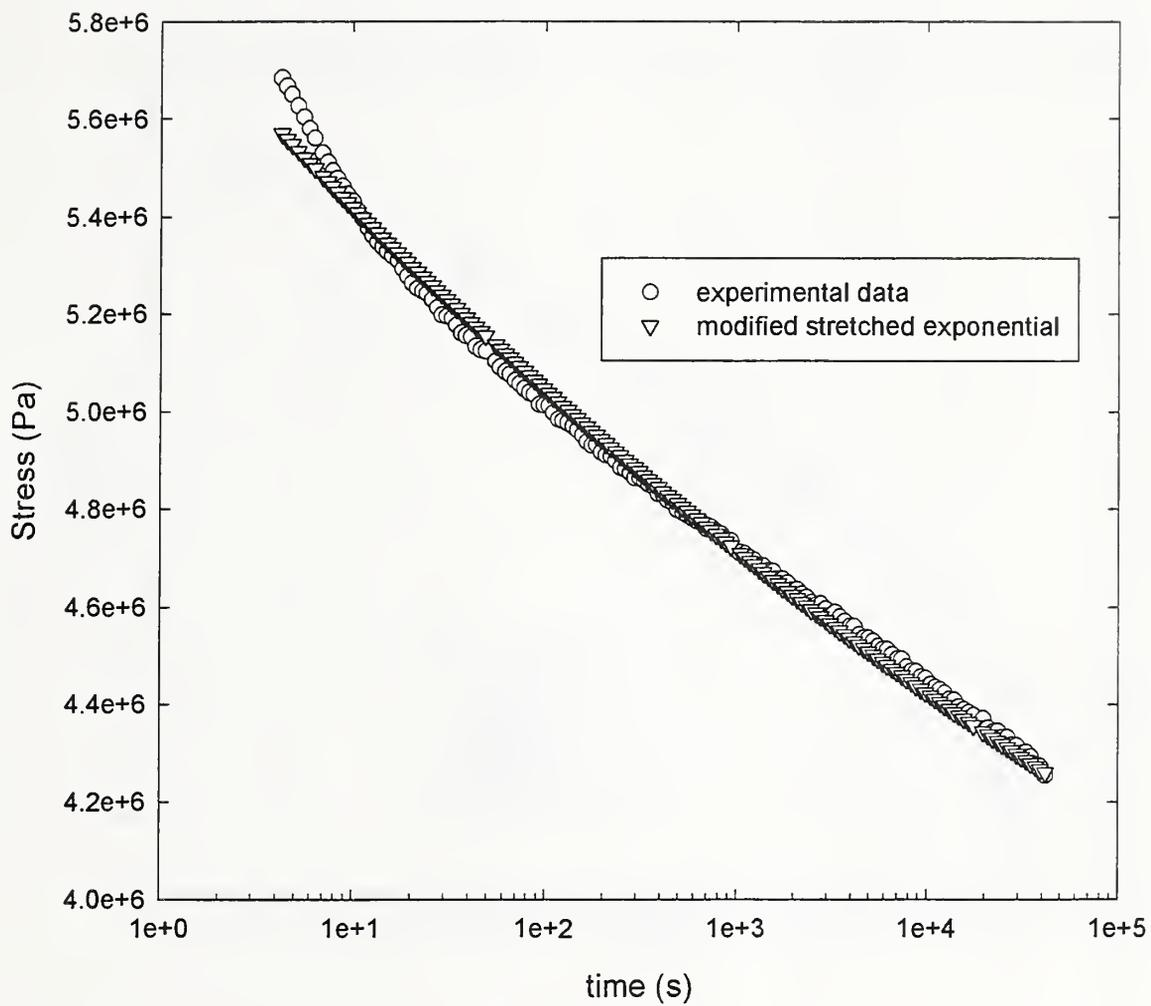
Figure 4: Stress versus Log(time) in stress relaxation test at  $\lambda=1.5$  and  $T=10^\circ\text{C}$ . The modified stretched exponential is given by Eq. (19).
