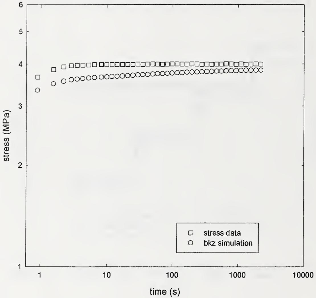
Figure 17: Log(stress) vs Log(time) curve for a multiple step-up creep experiment.
