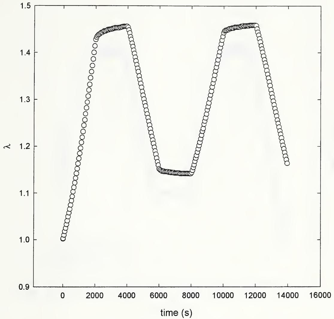
Figure 20: strain versus time vurve for a material response to a trapezoidal-shaped stress history.
