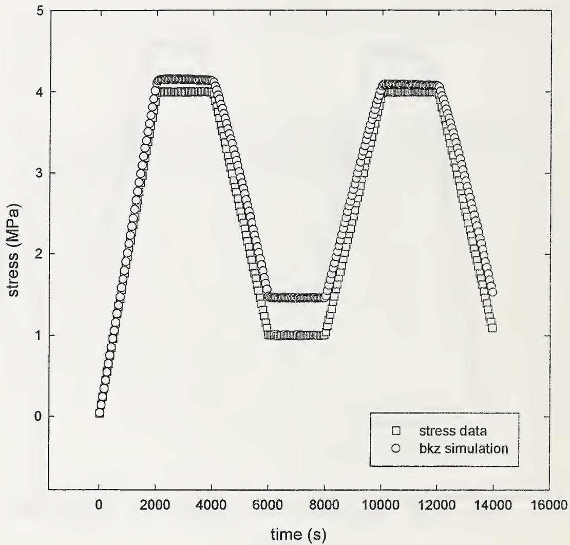
Figure 21: stress versus time curve for a material response to a trapezoidal-shaped stress history.
