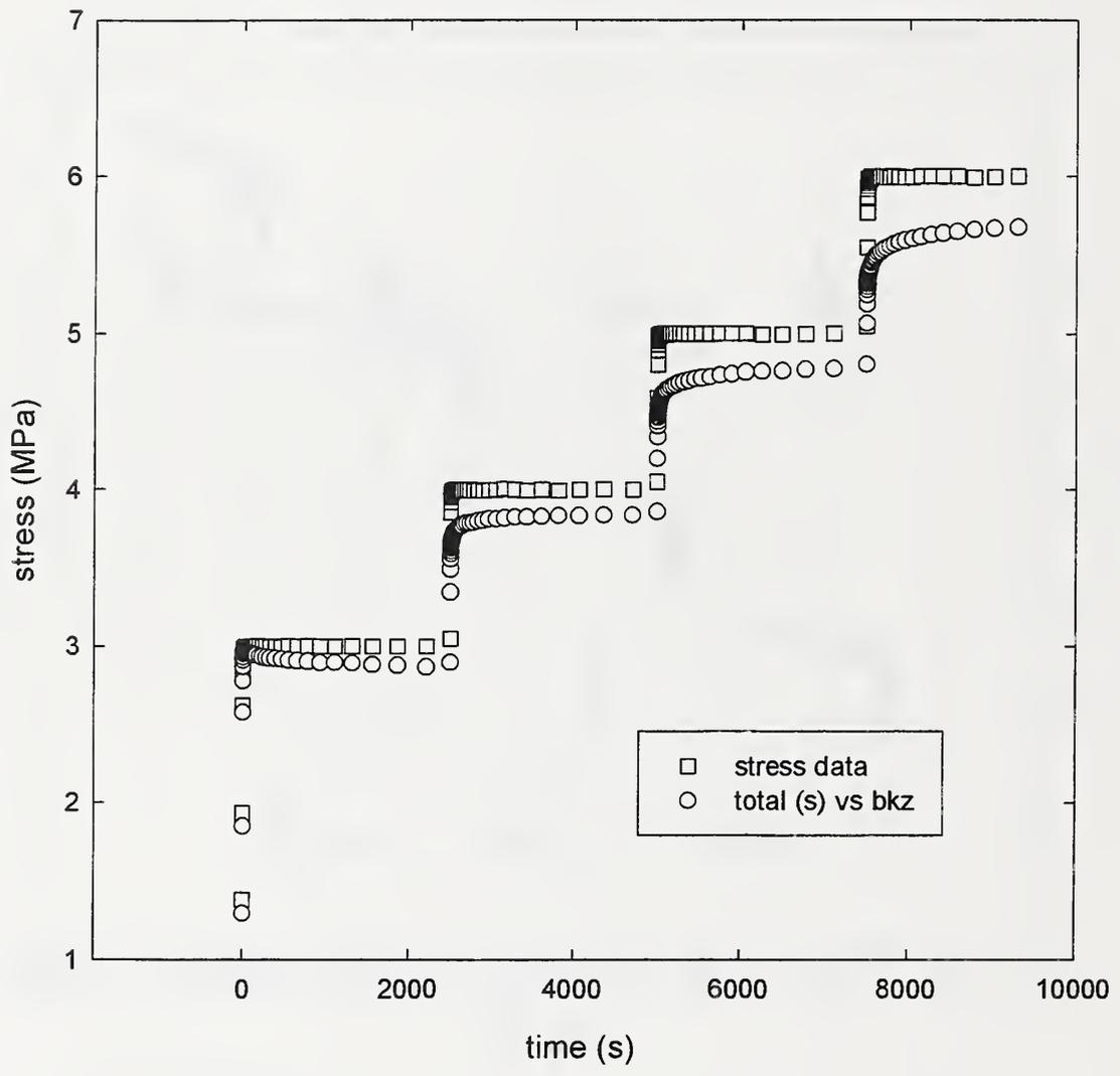
Figure 15: Stress versus time curve for a multiple step-up creep experiment T=10°C.
