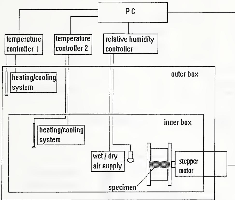
Figure 1. Schematic of Environmental Testing Chamber (See text).
