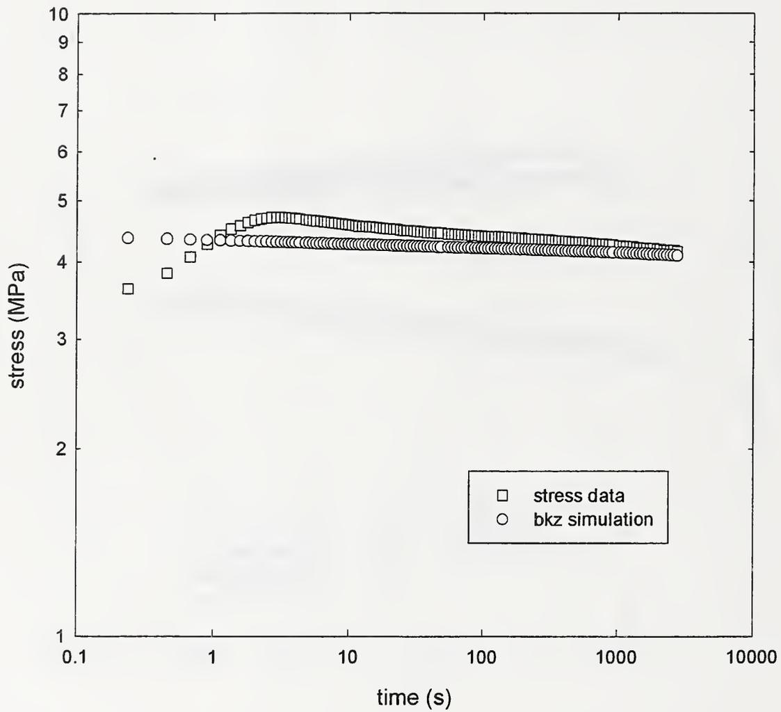
Figure 11: Log(stress) vs Log(time) curve for a multiple step-up stress relaxation experiment.
