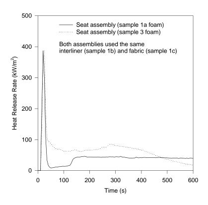
Figure 5-5. Comparison of Cone Calorimeter HRR - Two Seat Assemblies with Sample 1c Fabric
