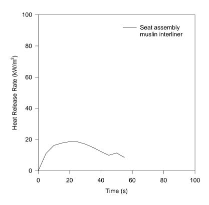
Figure 5-4. Cone Calorimeter HRR-Cotton Muslin Interliner (Sample 1b)
