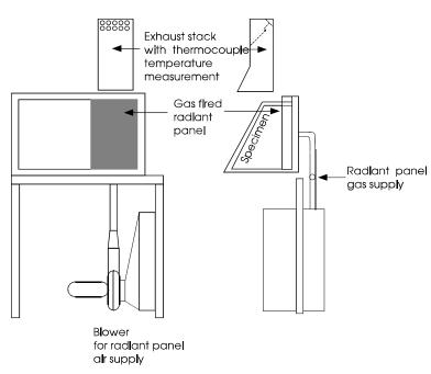
Figure B-1. ASTM E 162 Test Apparatus
