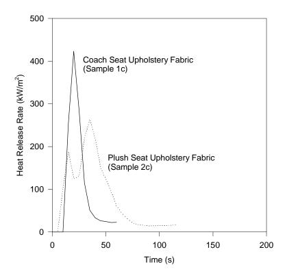
Figure 5-3. Comparison of Cone Calorimeter HRR for Two Upholstery Fabrics
