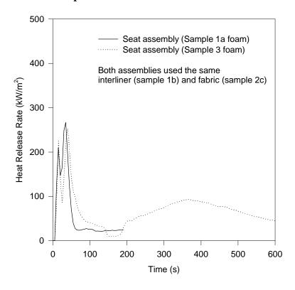
Figure 5-6. Comparison of Cone Calorimeter HRR - Two Seat Assemblies Sample 2c Fabric
