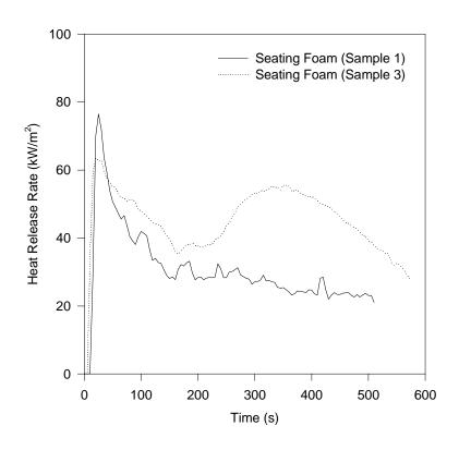
Figure 5-2. Comparison of Cone Calorimeter HRR for Two Foam Samples
