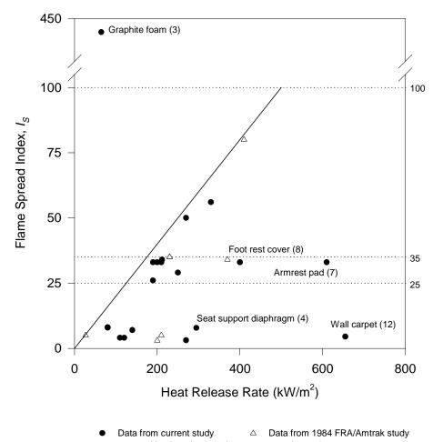
Numbers in parentheses are sample numbers Figure 6-1. Comparison of  $I_s$  as Measured According to ASTM E 162 / D 3675 and
