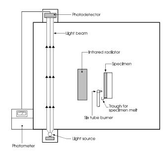
Figure B-2. ASTM E 662 Test Apparatus
