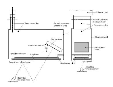
Figure B-3. ASTM E 648 Test Apparatus
