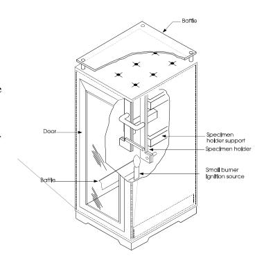
Figure B-4. FAR 25.853 (a) Test Apparatus
