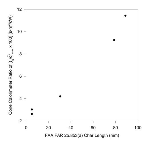
Figure 6-2. Comparison of Char Length as Measured According to FAR 25.853 (a) to the Ratio of Time to Ignition and Peak HRR as Measured in the Cone Calorimeter
