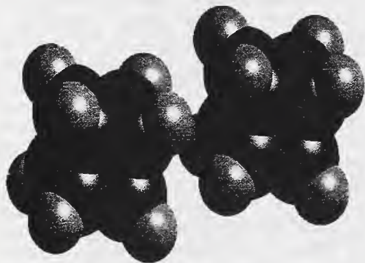
Fig. 1. Relative orientation of two nearest neighbor cubane molecules along one of the cell axes in the orientationally ordered phase. The darker spheres represent the carbon atoms and the lighter spheres represent the hydrogen atoms. The spheres have been arbitrarily expanded to a diameter corresponding to 0.7 times the Van der Waals radius for each atom.
