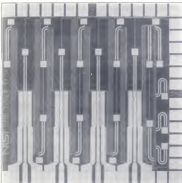
Stable 1-Volt programmable voltage standard. This 1 cm by 1 cm chip is a fully functional 1 V programmable standard. It contains 32,768 Nb-PdAu-Nb Josephson junctions. Each junction is 2 \mu\text{m} in diameter. The chip is biased with a continuous 16 GHz microwave frequency.
