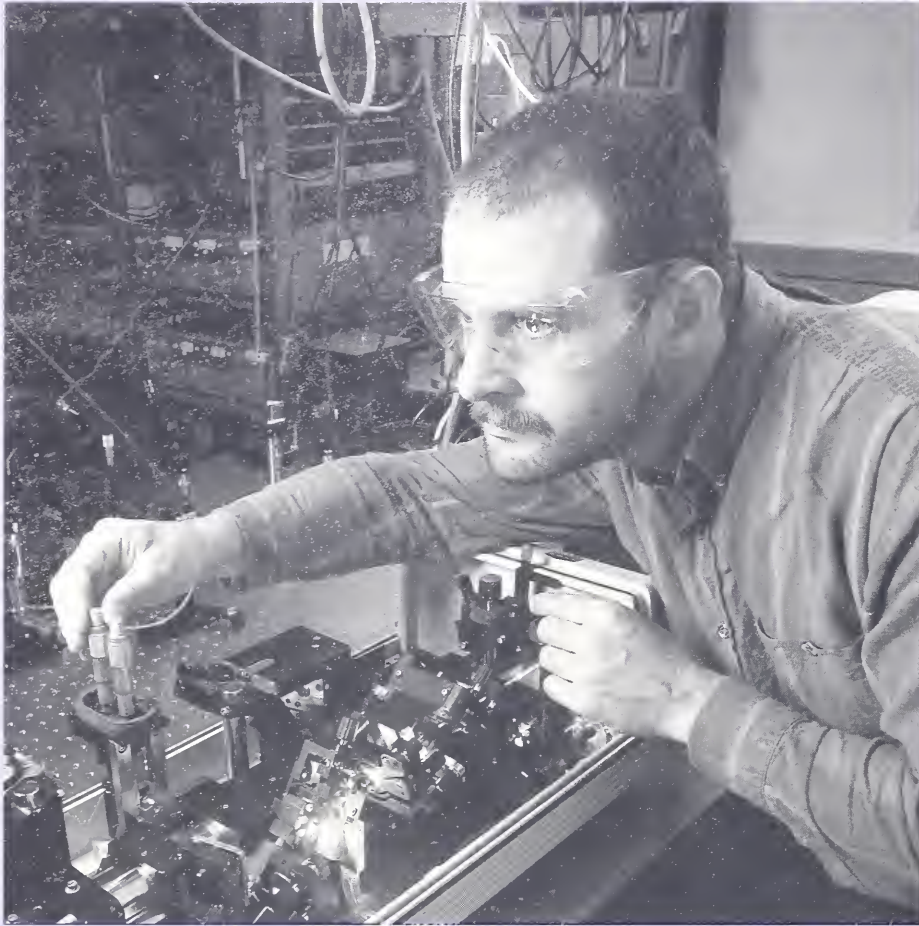
T. J. Silva – Measurement of second-harmonic magneto-optic Kerr effect (SHMOKE) in thin films.
