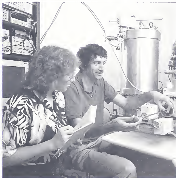
(Front to back) L. L. Dulcie, J. M. Martinis – Loading samples into a scanning electron microscope to test the performance of their microcalorimeter in x-ray microanalysis.
