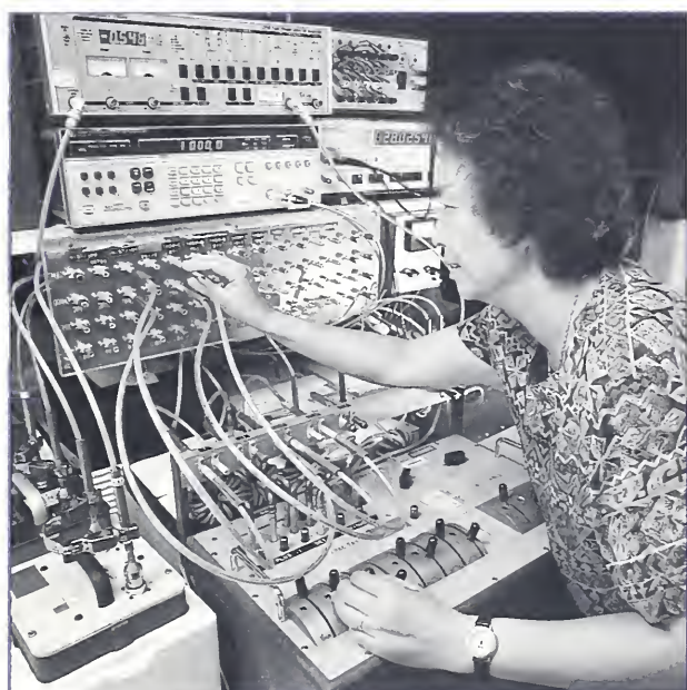
Y. M. Chang – Balancing the Type-2 bridge. Adjustment of the internal capacitance and conductance standards are necessary to obtain a null balance, which determines the value of the capacitor under test.
