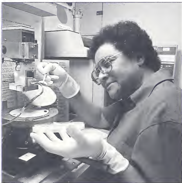
D. R. Ricks – Mounting a silicon wafer on the resistivity instrument stage prior to taking measurements for SRM certification.
