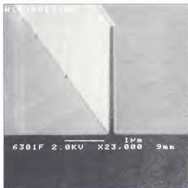
Cross section of a critical dimension artifact.
