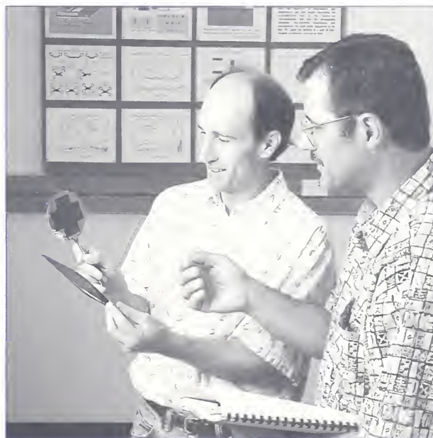
(Left to right) D. F. Williams, R. M. Judish. Examining multiconductor transmission lines fabricated on a silicon substrate.
