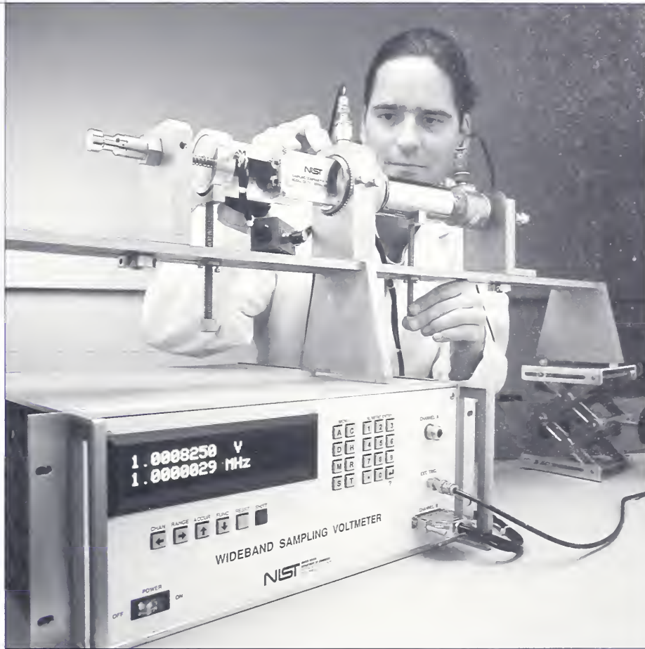
B. C. Waltrip – Measurement of voltmeter gain flatness. Adjusting a test jig used to compare the wideband sampling voltmeter with a calibrated thermal voltage converter.
