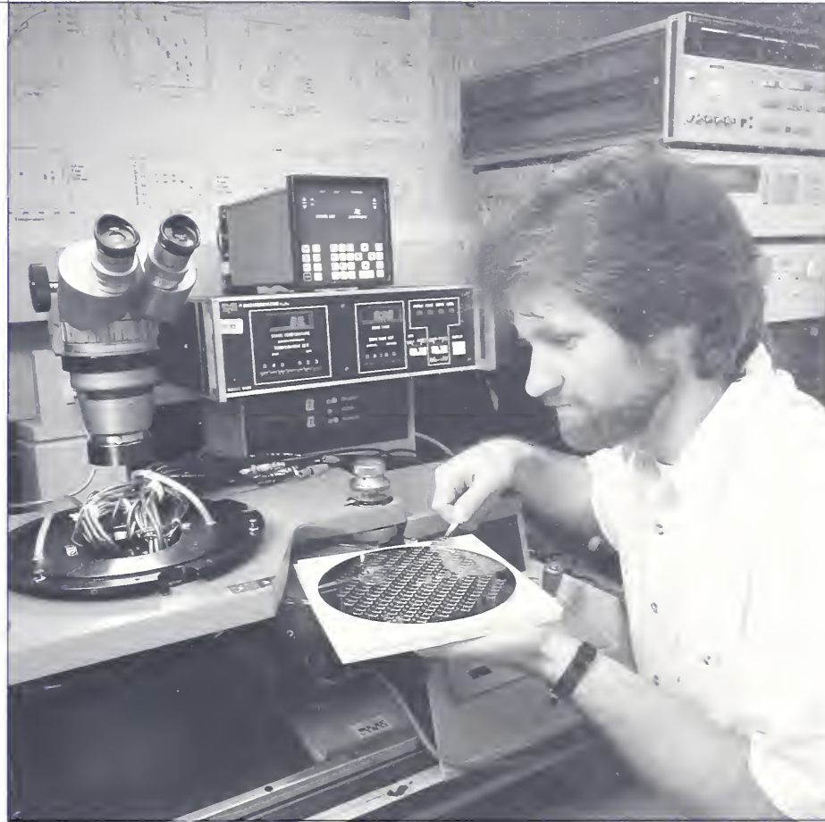
J. S. Suehle – Test wafer being loaded on wafer prober for long-term dielectric testing.
