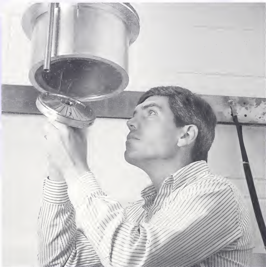
S. L. Bray – Mounting an aluminum-composite ring in superconducting magnet for cryogenic fatigue testing.
