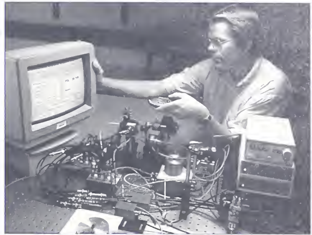
R. M. Craig – Variable retardance, fixed states system for measuring polarization-dependent loss. Measurement parameters are entered through a visual interface with a handheld remote.
