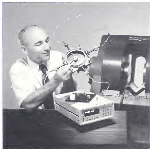
R. G. Geyer – Describing use of low-loss dielectric ring resonators.
