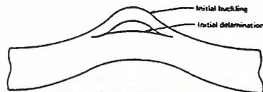
Figure 3-9. Initial Buckling of the Delamination Followed by Global Buckling (Failure Mode 4)
