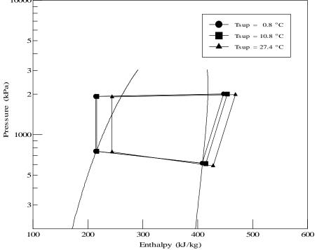
Figure 16. Pressure-Enthalpy Diagram for R-22 Diagram for R-22 During the Cooling Test at Different Superheats at the LLSL-HX Outlet (1800 Compressor RPM)
