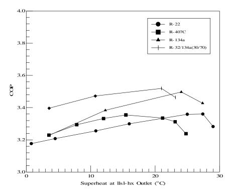
Figure 14. COP During the Cooling Test (System with LLSL-HX, 1800 Compressor RPM)
