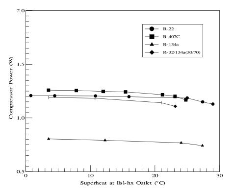
Figure 13. Compressor Power During the Cooling Test (System with LLSL-HX, 1800 Compressor RPM)
