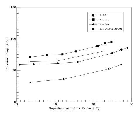
Figure 18. Refrigerant Pressure Drop in the Counter-Flow Evaporator During the Cooling Test (System with LLSL-HX, 1800 Compressor RPM)
