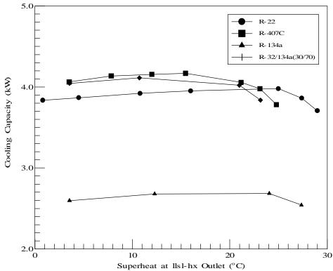
Figure 12. Capacity During the Cooling Test (System with LLSL-HX, 1800 Compressor RPM)
