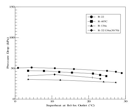
Figure 17. Refrigerant Pressure Drop in the Cross-Flow Condenser During the Cooling Test (System with LLSL-HX, 1800 Compressor RPM)
