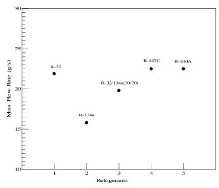
Figure 4. Refrigerant Mass Flow Rate in the Basic System During the Cooling Test (1800 Compressor RPM)
