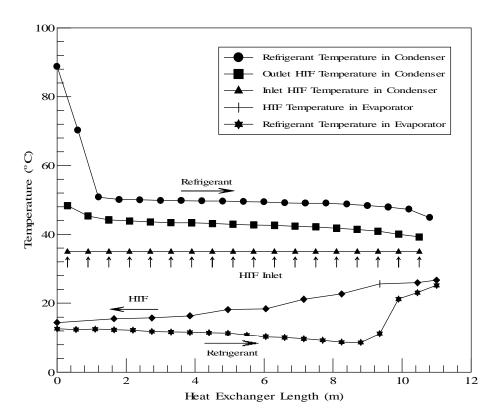
Figure 7. Temperature Distribution of R-22 in Cross-Flow Condenser and Counter-Flow Evaporator During the Cooling Test (Basic System, 1800 Compressor RPM)
