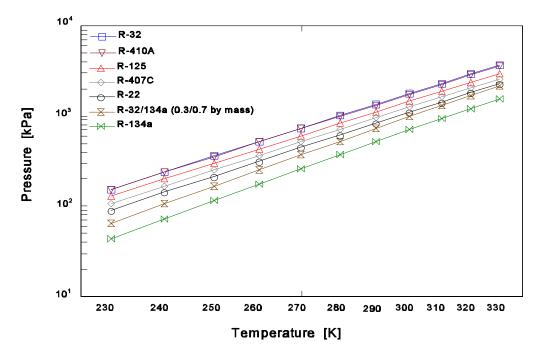
Figure 2. Dew Point Vapor Pressures for Refrigerants Studied
