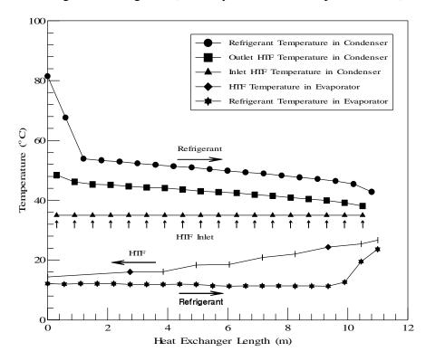
Figure 8. Temperature Distribution of R-407C in Cross-Flow Condenser and Counter-Flow Evaporator During the Cooling Test (Basic System, 1800 Compressor RPM)
