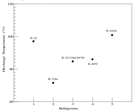
Figure 6. Compressor Discharge Temperature for the Basic System During the Cooling Test (1800 Compressor RPM)
