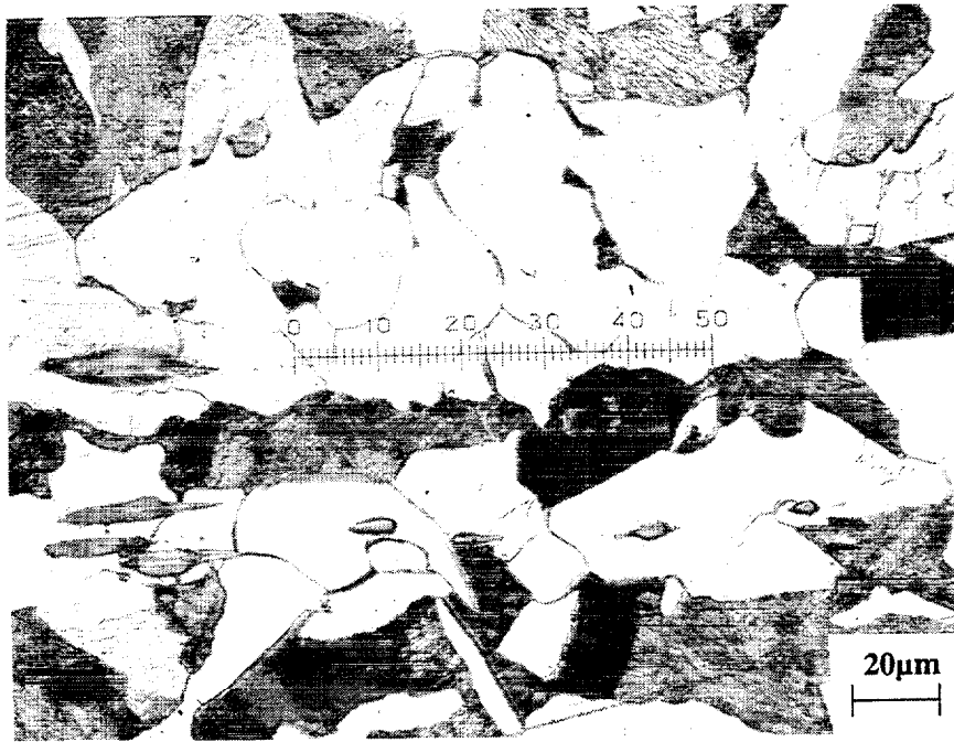
Sample A254 - Column Flange Magnification: 500X Etchant: 2% Nital
