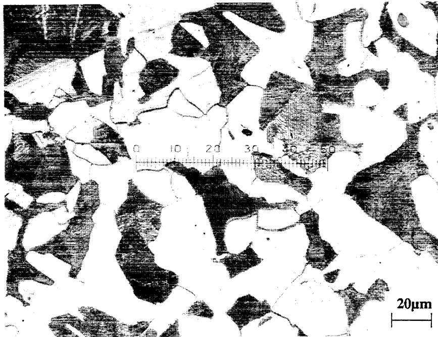
Sample A165 - Column Flange Magnification: 500X Etchant: 2% Nital
