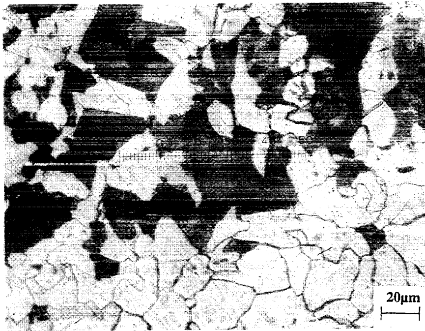
Sample E549 - Column Flange Magnification: 500X Etchant: 2% Nital
