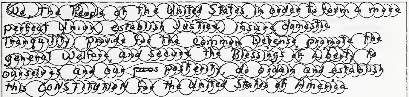
Figure 5. Traces of the bubbles used to sort the connected components into lines.
