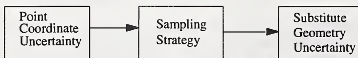
Figure 2. Schematic of the various factors affecting the CMM measurement of a small ring gauge.
