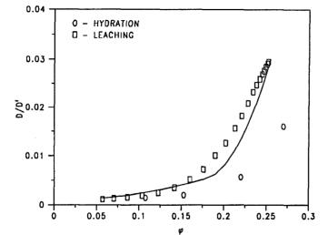
Figure 2: Formation factor,  $D/D^f$ , due to hydration (circles) and to leaching (squares) for w/c=0.35 (after [14]). The solid line represents the approximation used by 4SIGHT for the leaching formation factor.
