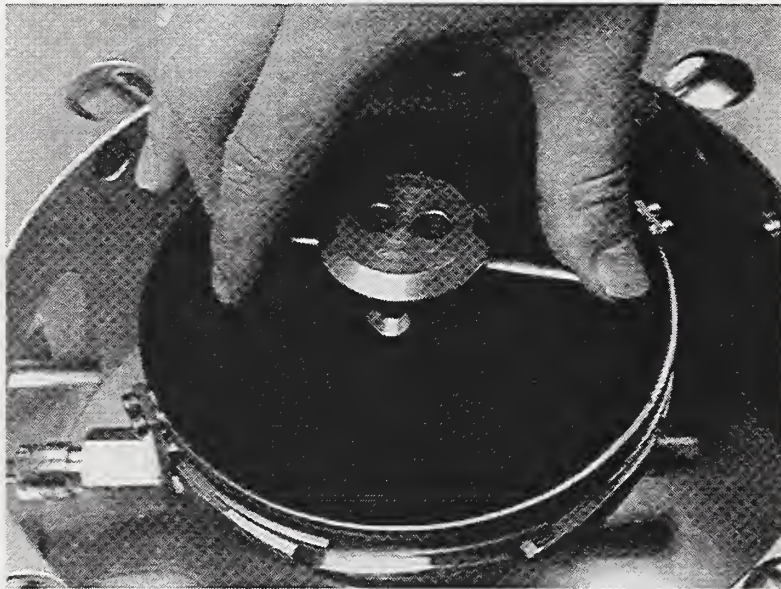
Figure 17. Fastening the automatic pneumatic ITA to the CMM
