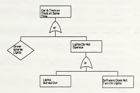
Figure 3-6 System Fault Tree.
