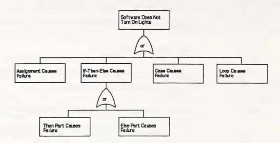
Figure 3-7 Software Fault Tree.
