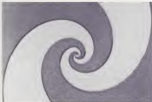
DETAIL OF MICROMETER-SIZED IR ANTENNA
