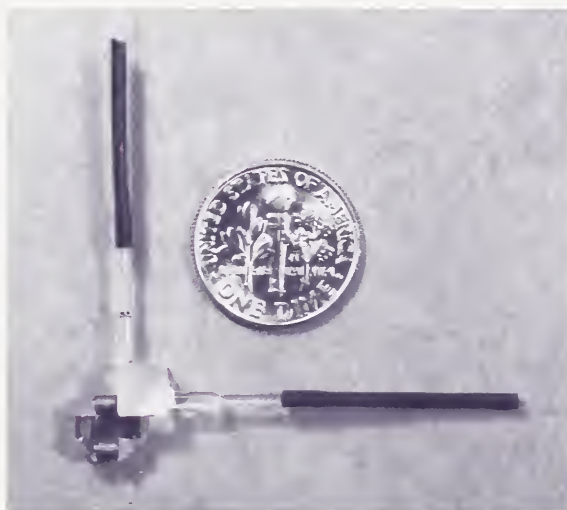
OPTICAL-FIBER CURRENT SENSOR
