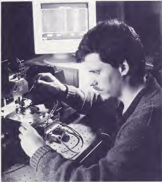
ADJUSTING SENSITIVITY FOR SCM FOR 2-D DOPANT PROFILING
