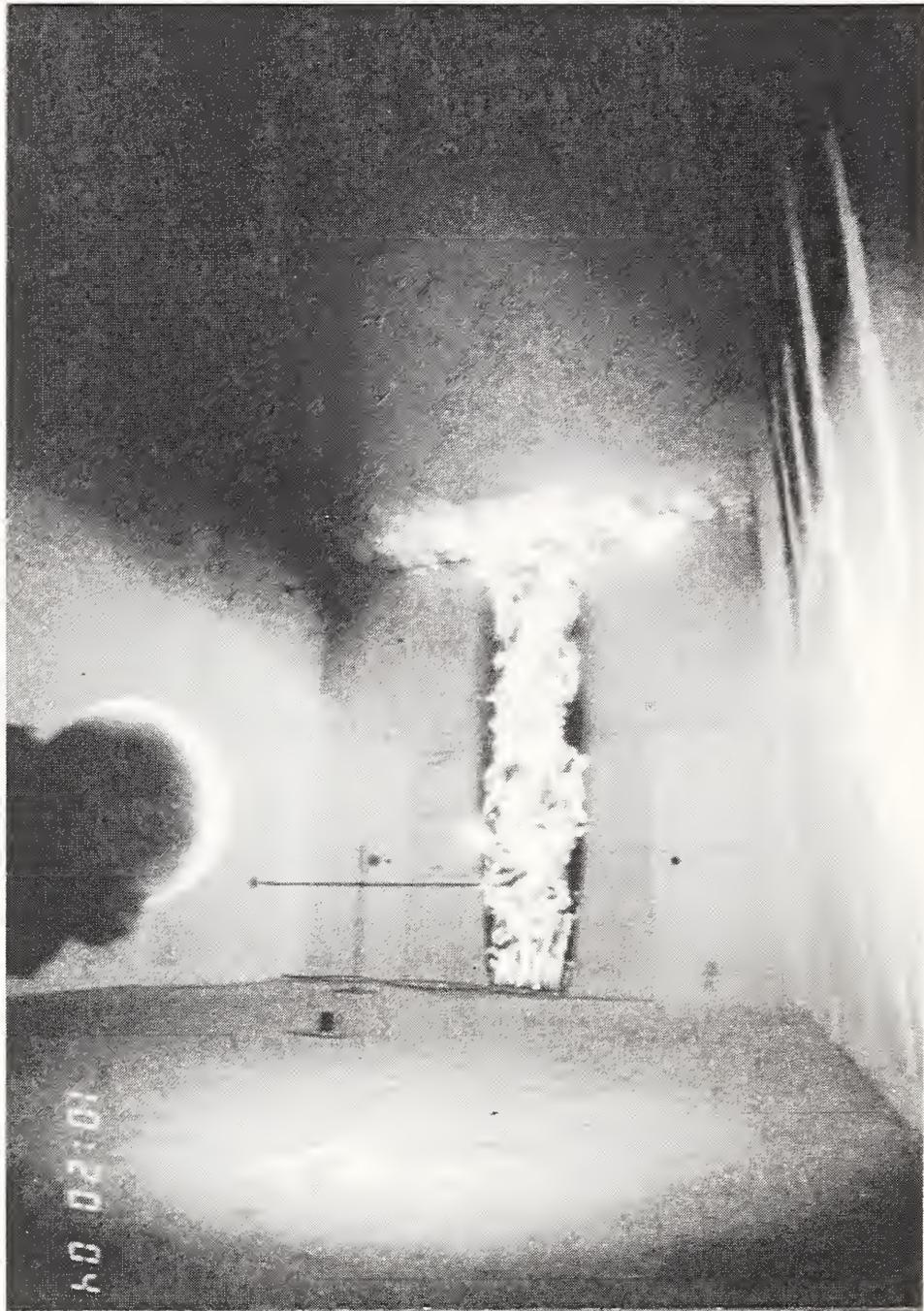
Figure 6. Photograph of a wall fire with the flame impinging on the ceiling. From an experiment carried out at CFR/NBS by B. Lee in 1986. Photo courtesy of R. Peacock.
