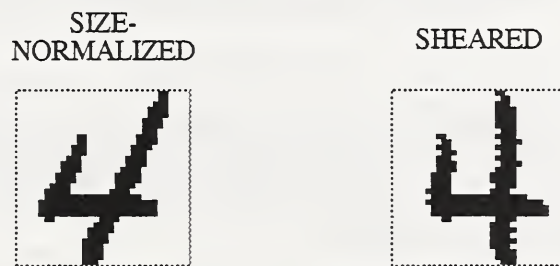
Figure 24. Slant removed from a character image via shearing.
