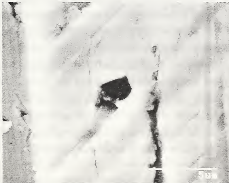
Fig. 16. SEM micrograph of Al 2 O 3 particle embedded in 52100 steel disk.
