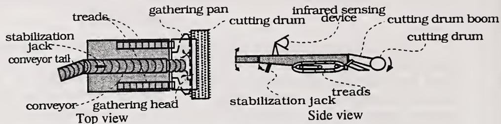
Figure 1: A continuous mining machine and appendages
