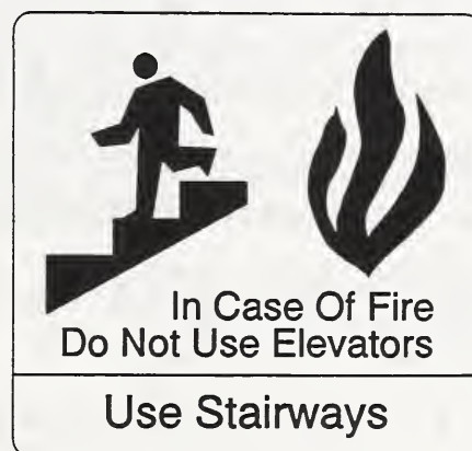
Figure 1. Typical sign currently used to indicate that elevators should not to be used during fires
