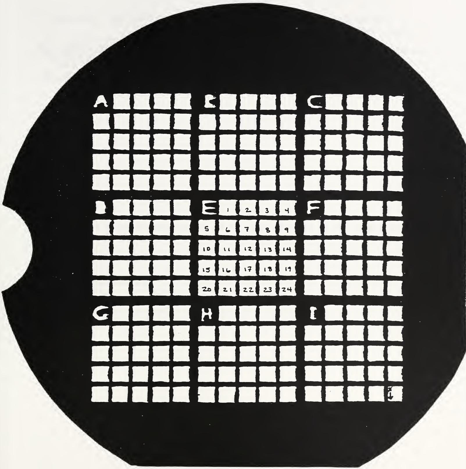
Figure 1. Indexed Electron Microscope Grid. Grids in block "E" show how the grid squares are numbered. Grid square I-24 shows initial start point and scan direction for structure counting.
