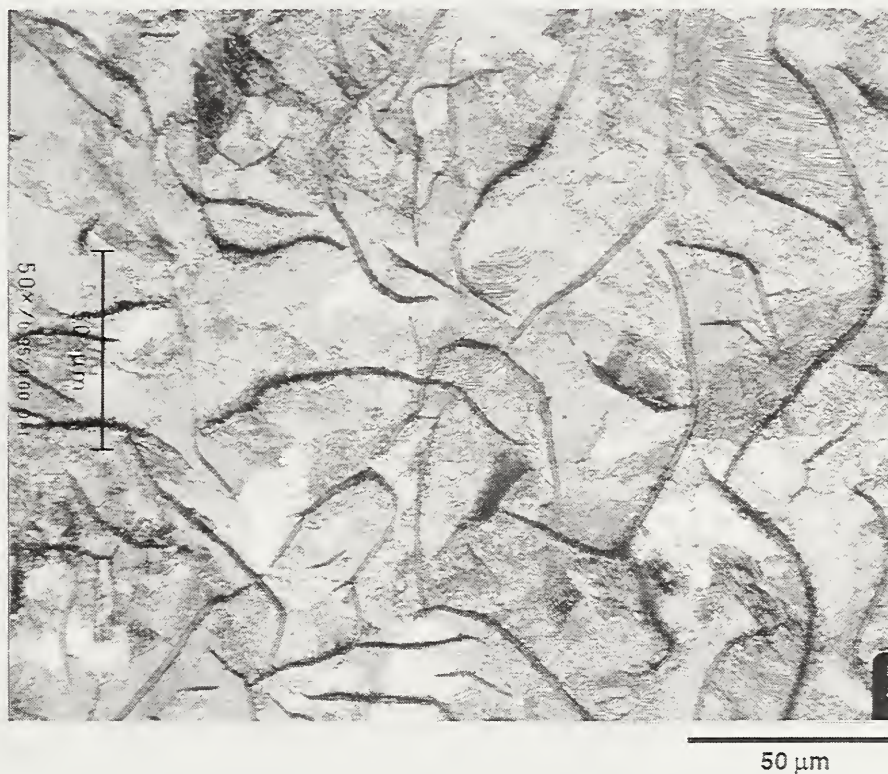
Figure 4 Optical micrograph showing the graphite flakes in a pearlite matrix microstructure of a failed cast iron coupling taken from the Filene Center . Etchant: 2% nital
