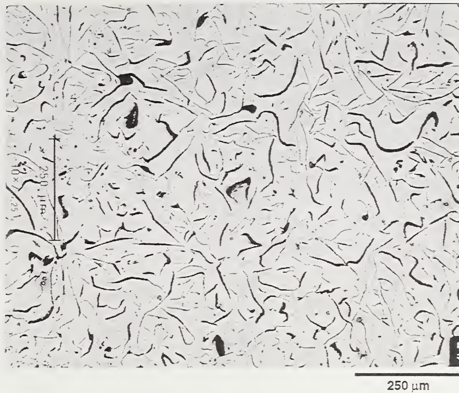
Figure 3 Optical micrograph in the "as polished" condition showing the microstructure of a failed cast iron coupling taken from the Filene Center.
