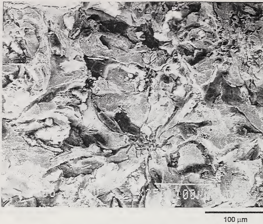
Figure 5 Low magnification scanning electron micrograph showing brittle cracking along the graphite matrix interfaces on a fracture surface taken from a failed cast iron coupling at the Filene Center.
