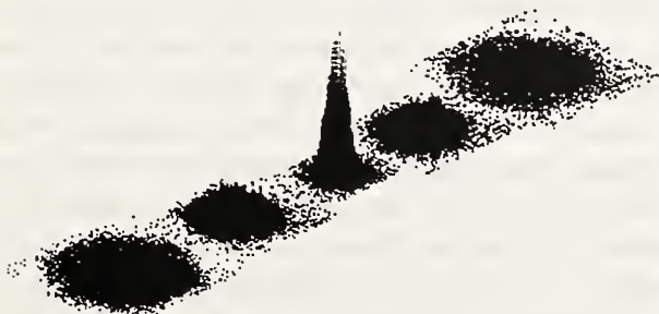
Figure 2. Intensity distribution of images at different distances around the focus.
