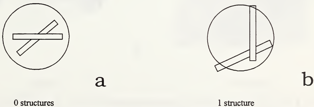
FIG. X1.2 Interconnecting fibrils (item 5.1.2): a) the largest dimension of the particle is less than 0.5 \mu\text{m} and therefore the particle is not counted as a structure; b) the largest dimension of the interconnecting fibrils is greater than 0.5 \mu\text{m} and therefore the particle counts as one structure.
