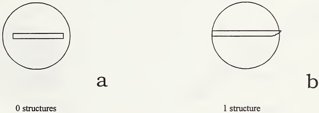
FIG X1.1 Single fibrils (item 5.1.1): a) the fibril is less than 0.5 \mu\text{m} in length and therefore is not counted as a structure; b) the fibril has an irregular termination - the longest dimension parallel to the fibril axis is greater than 0.5 \mu\text{m} and therefore the fibril counts as one structure (item 3.1.2).
