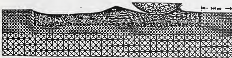
(e) t = 19.0 \mu\text{s} , depth = 32 \mu\text{m} , distance = 1584 \mu\text{m} , average velocity = 227 \text{ m/s}
