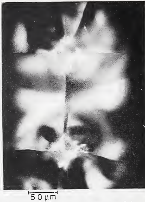
Figure 1. Optical reflection micrograph of a glass slide showing a Vickers indent pair and associated vertical and lateral cracks.
