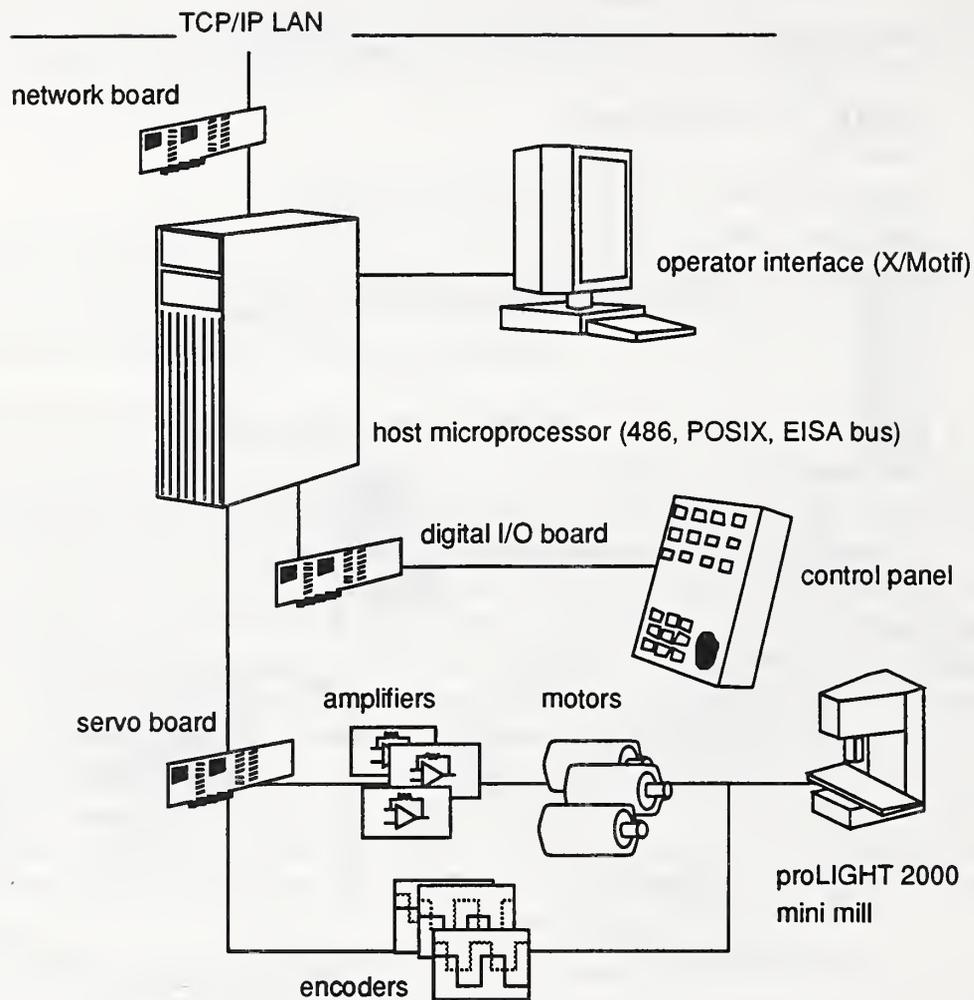
Figure 3. Laboratory Development Controller.
