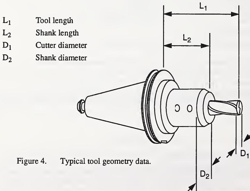
Figure 4. Typical tool geometry data.
