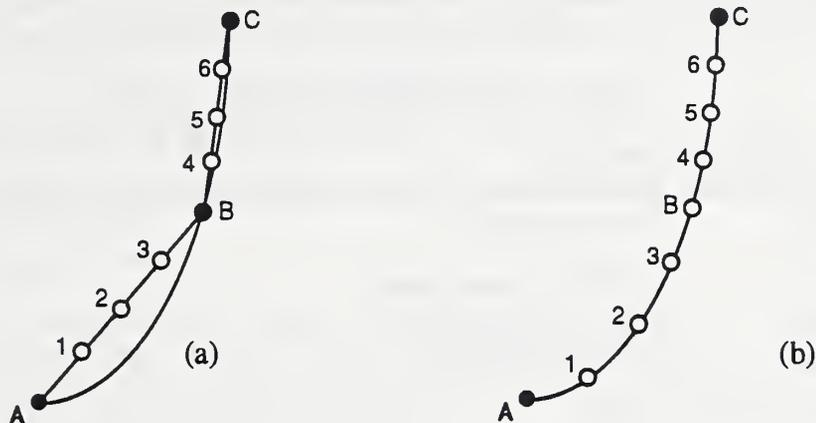
Figure 5. (a). Approximation of curve with line segments. Numbered points are generated by interpolation during machining.
