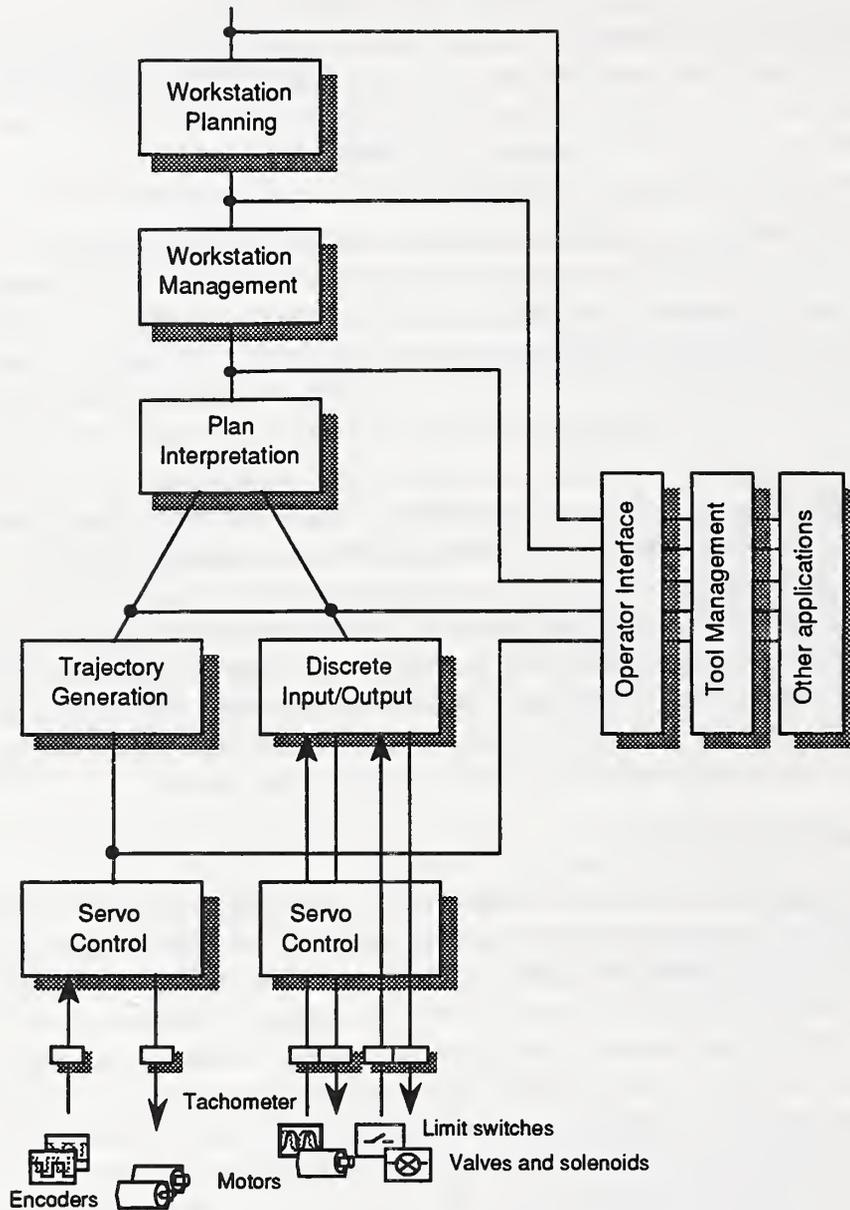
Figure 1. The Enhanced Machine Controller architecture.
