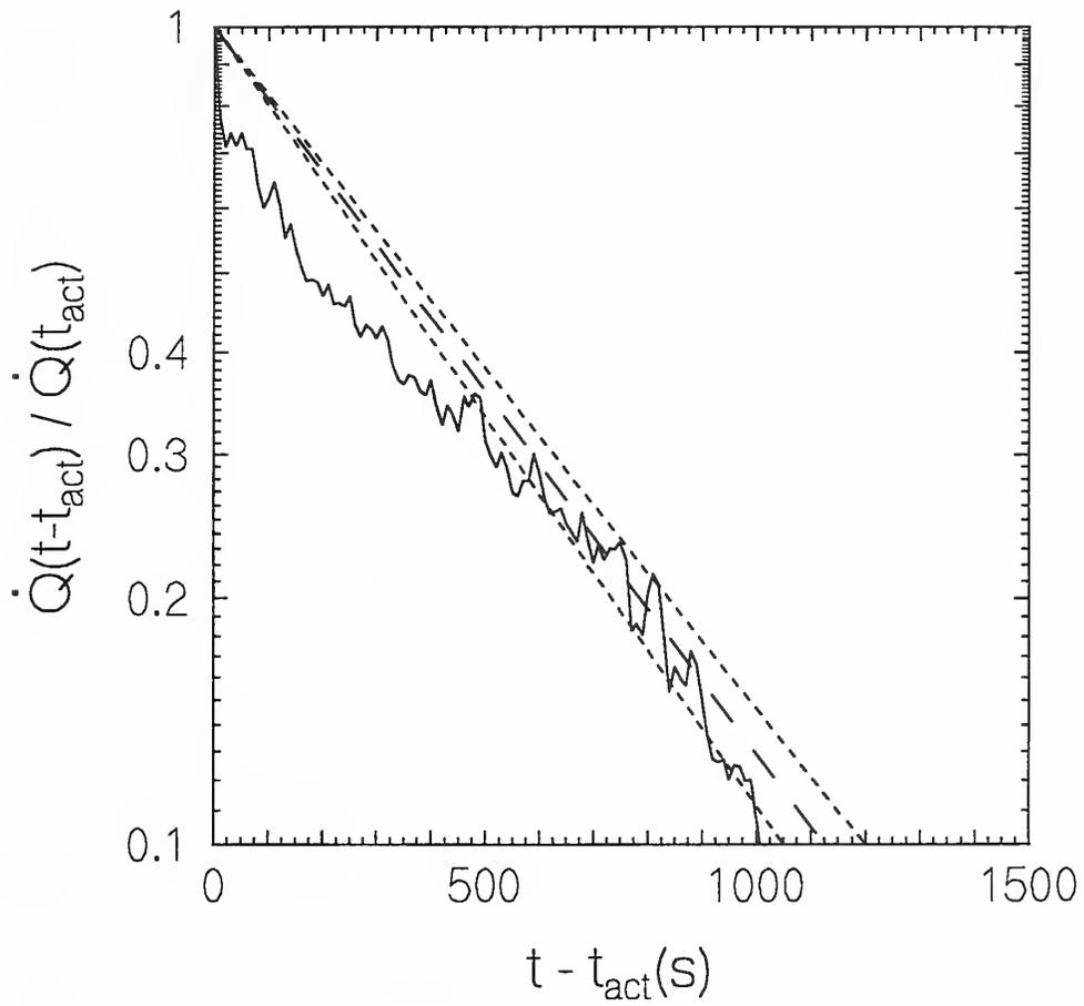
Figure 5. Time constant for 610 mm wood crib fire suppression at 0.066 mm/s sprinkler spray density
