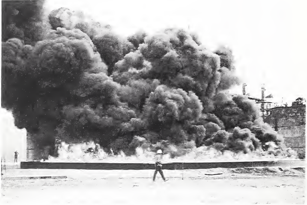
Figure 1. 15.2 m square mesoscale crude oil burn
