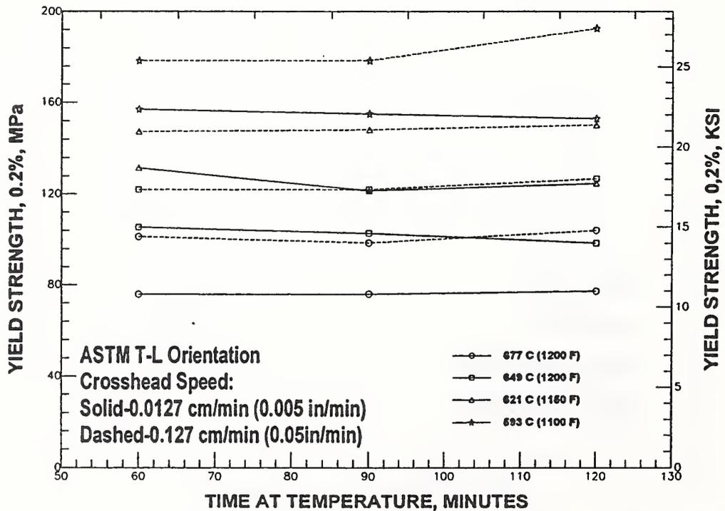
Figure 21. Effects of crosshead speed, temperature, and time on the YS. Specimens were taken from the ASTM T-L direction in the plate.
