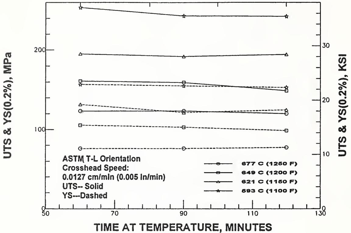
Figure 16. UTS and YS results for specimens tested at a crosshead speed of 0.0127 cm/minute and taken from the ASTM T-L direction in the plate.
