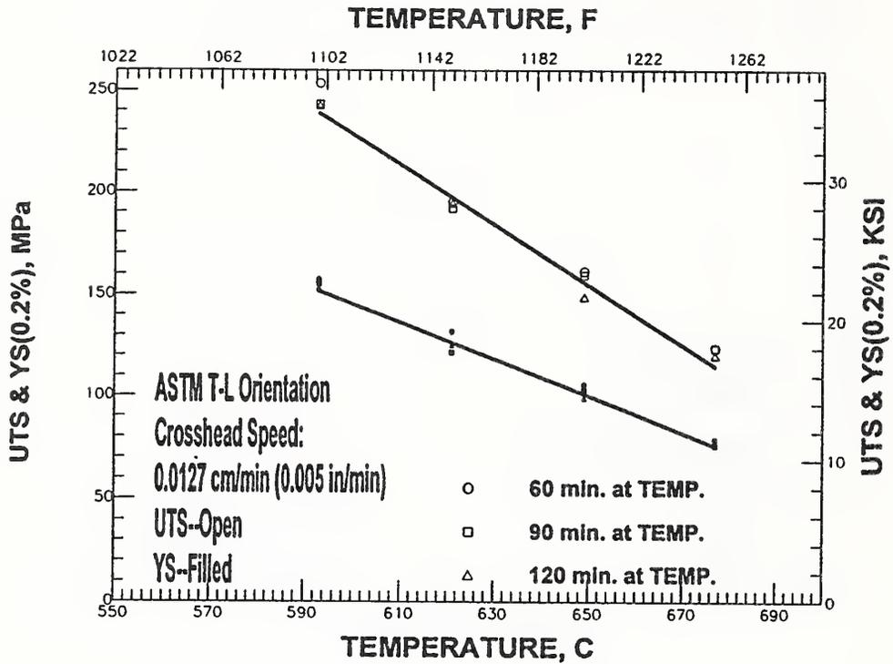
Figure 24. UTS and YS as a function of temperature. Specimens were taken from the ASTM T-L direction in the plate and tested at a crosshead speed of 0.0127 cm/minute.
