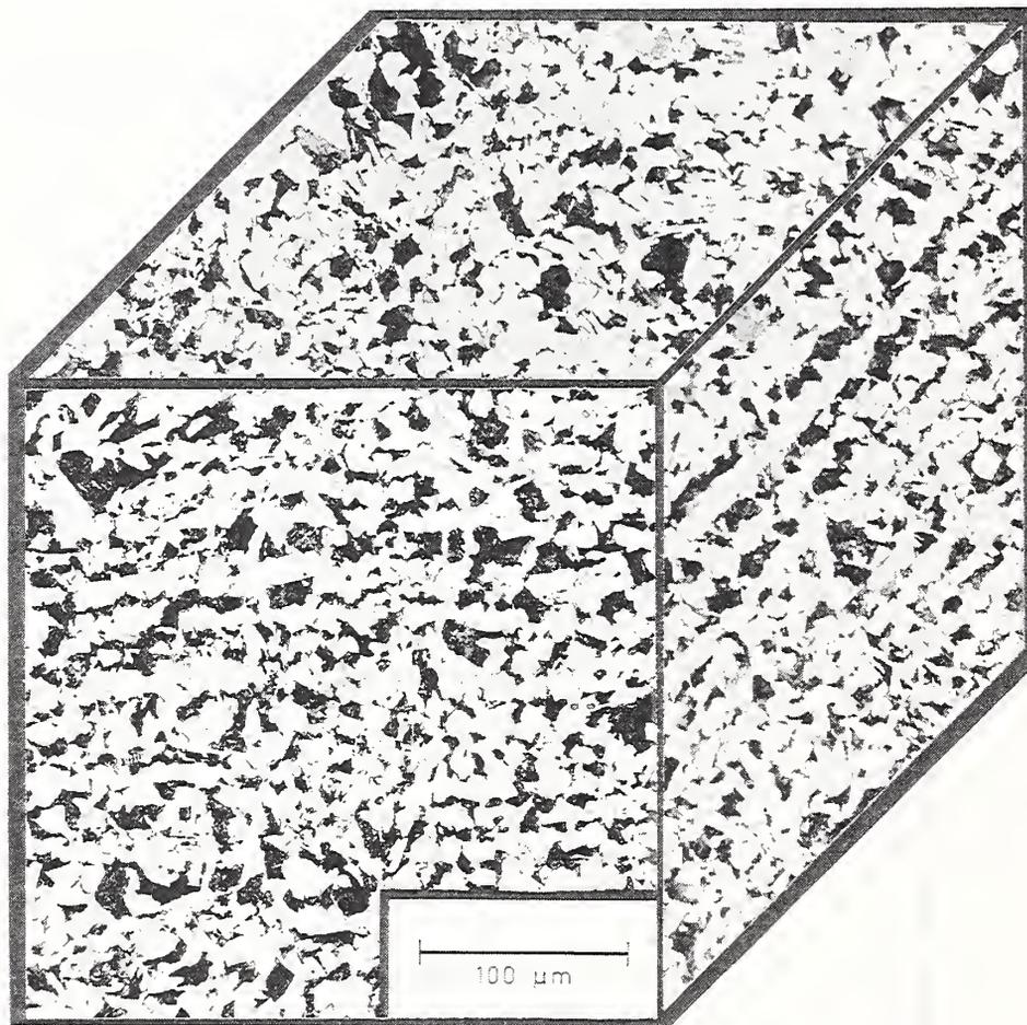
Figure 2. Photomicrographs of the as-received normalized AAR TC128 grade B steel in three orthogonal directions in the etched condition. Etch: 1% Nital
