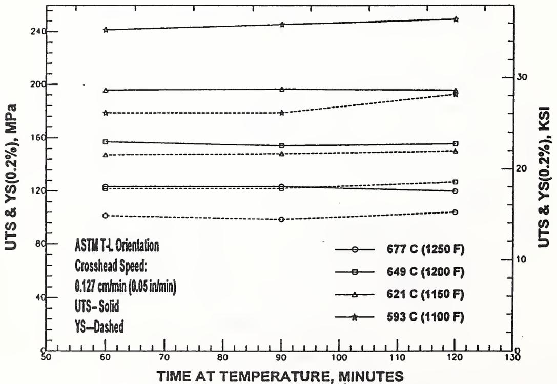
Figure 17. UTS and YS results for specimens tested at a crosshead speed of 0.127 cm/minute and taken from the ASTM T-L direction in the plate.
