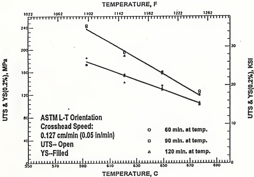
Figure 23. UTS and YS as a function of temperature. Specimens were taken from the ASTM L-T direction in the plate and tested at a crosshead speed of 0.127 cm/minute.
