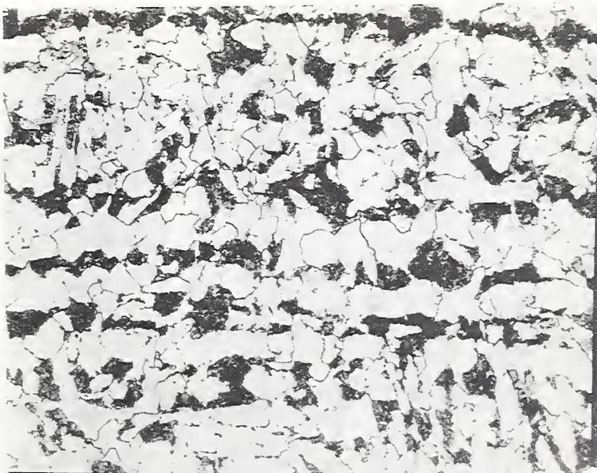
Figure 3. Photomicrographs of the as-received normalized and stress relieved AAR TC128 grade B taken at two different locations. Etch: 1% Nital Mag. X500.
