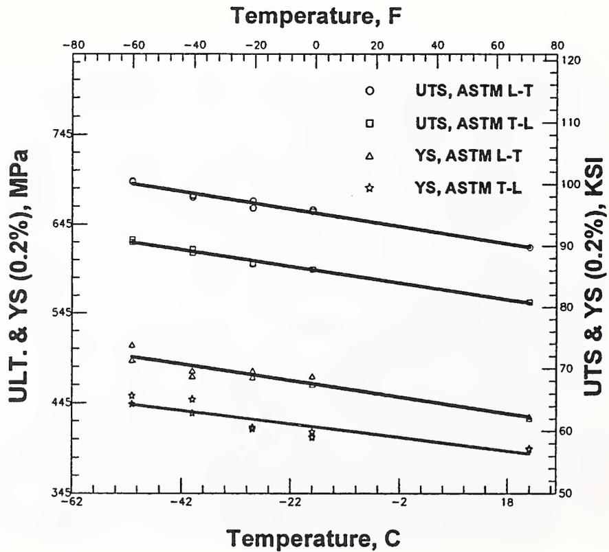
Figure 13. UTS and YS results for normalized and stress relieved AAR TC128 grade B tensile specimens tested at room temperature to -51 C.
