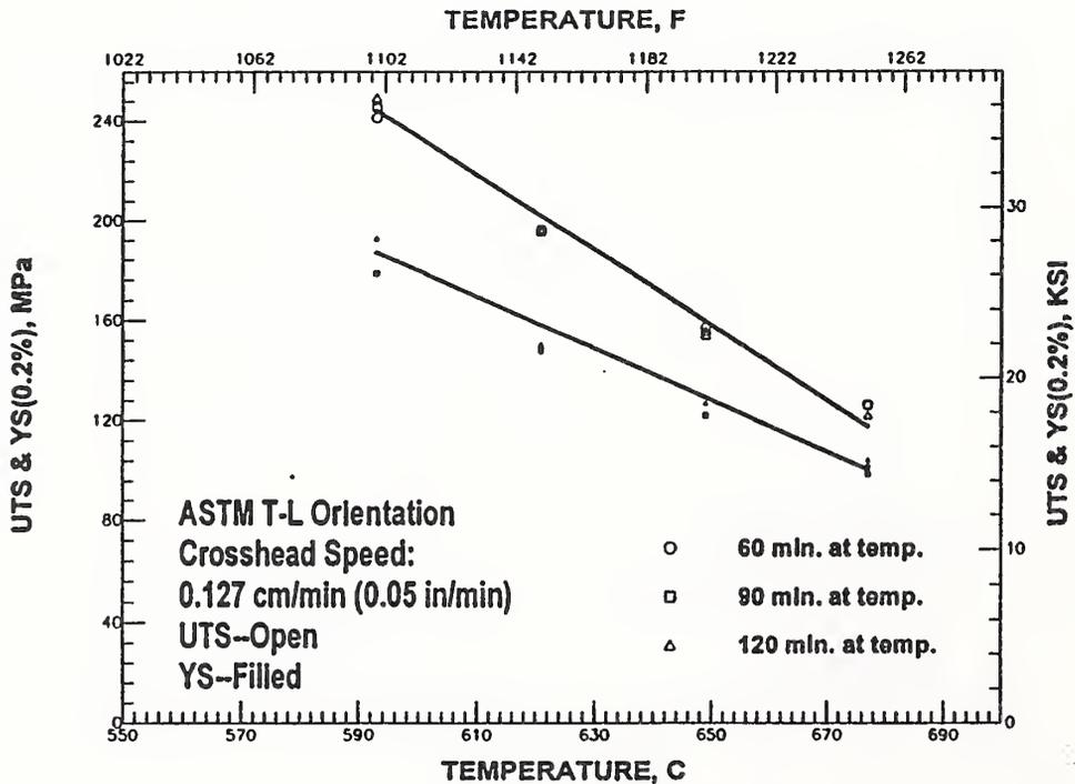
Figure 25. UTS and YS as a function of temperature. Specimens were taken from the ASTM T-L direction in the plate and tested at a crosshead speed of 0.127 cm/minute.
