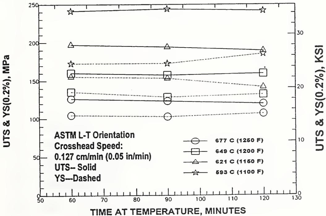
Figure 15. UTS and YS results for specimens tested at a crosshead speed of 0.127 cm/minute and taken from the ASTM L-T direction in the plate.
