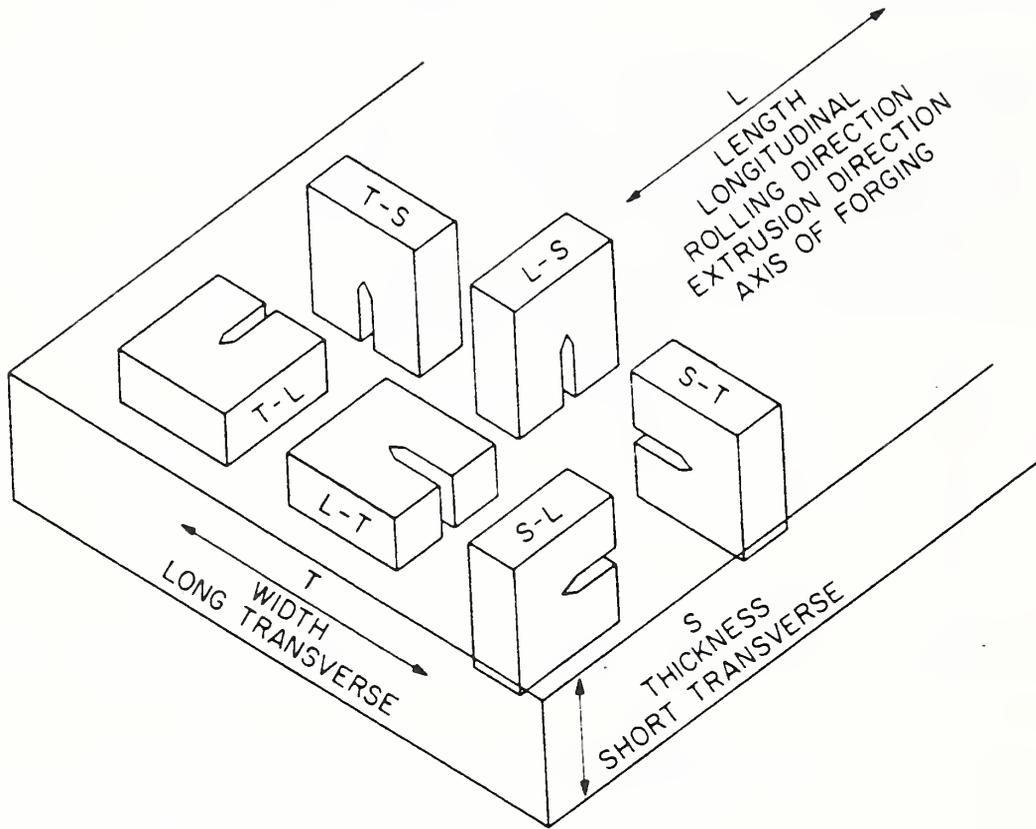
**Crack Plane Orientation Code for Rectangular Sections**
