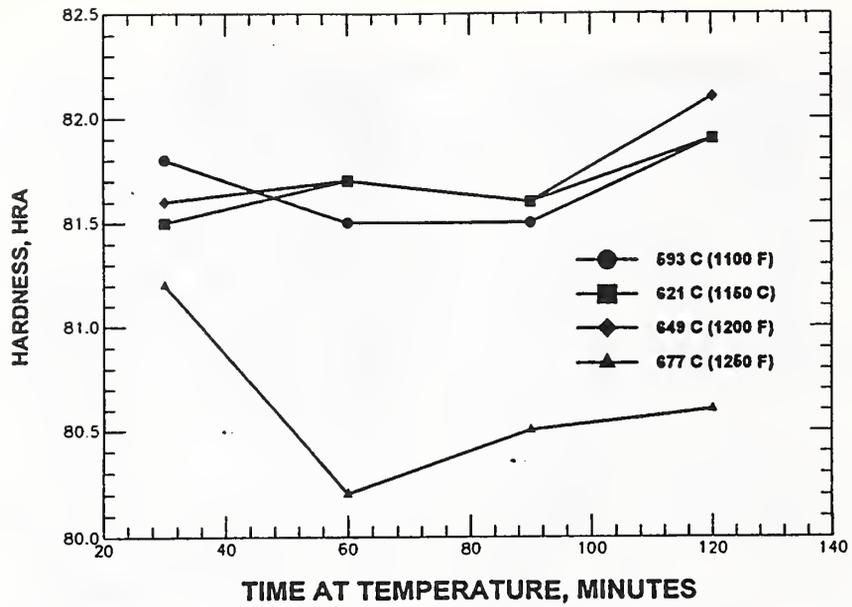
Figure 12. Average hardness (Rockwell A) versus time at 593 C, 621 C, 649 C, and 677 C for normalized and stress relieved AAR TC128 grade B steel specimens.
