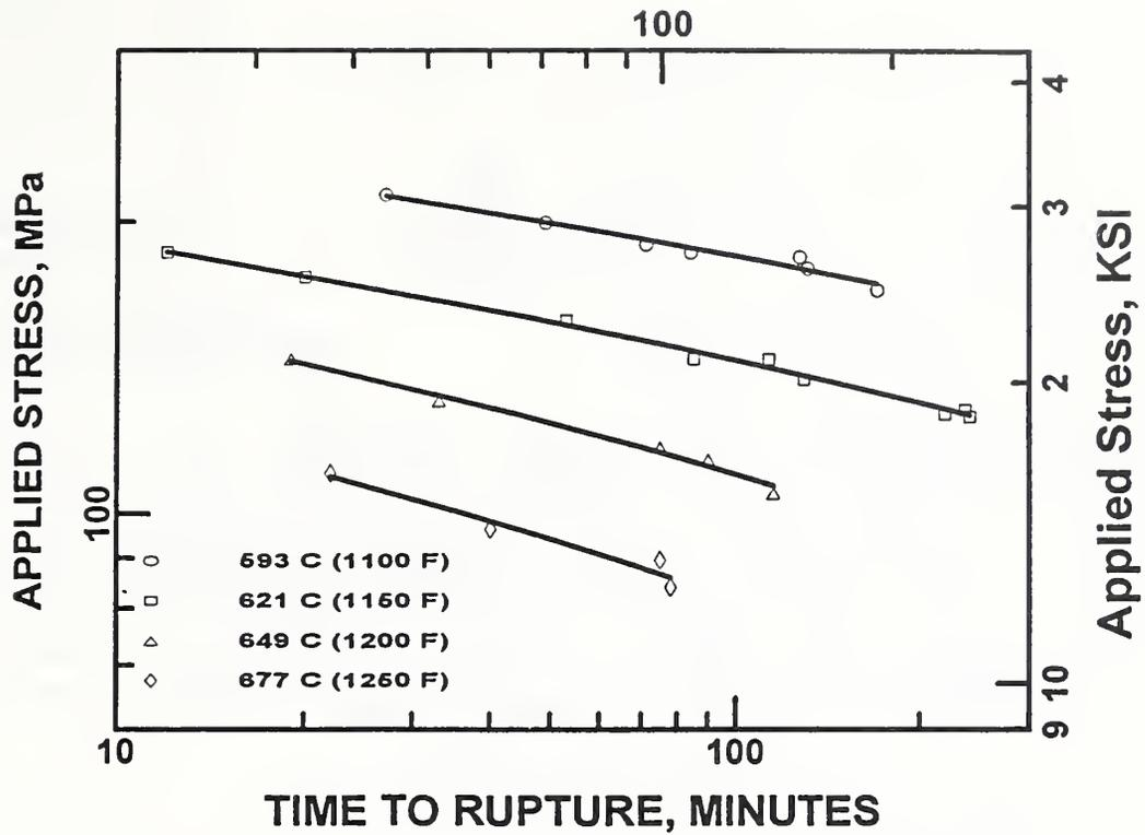
Figure 26. Applied stress versus time to rupture as a function of temperature.
