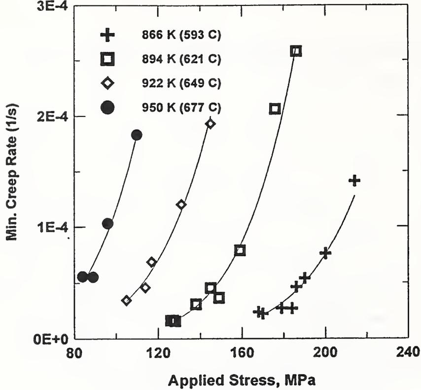
Figure 28. Minimum creep rate versus the applied stress as a function of temperature.
