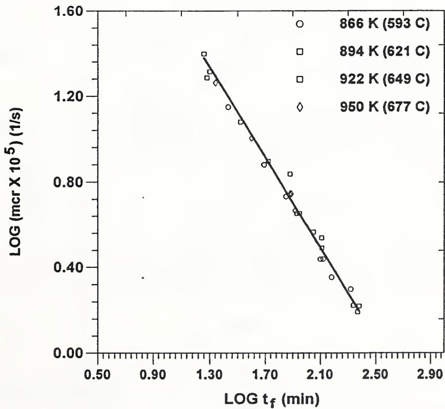
Figure 27. Log of the minimum creep rate versus the log of the time to failure.
