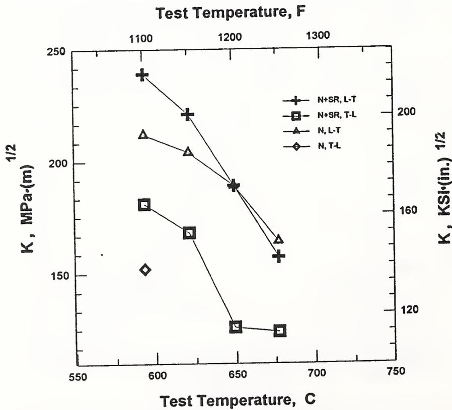
Figure 29. Fracture toughness versus test temperature. Both the ASTM T-L and L-T directions are shown in the figure.
