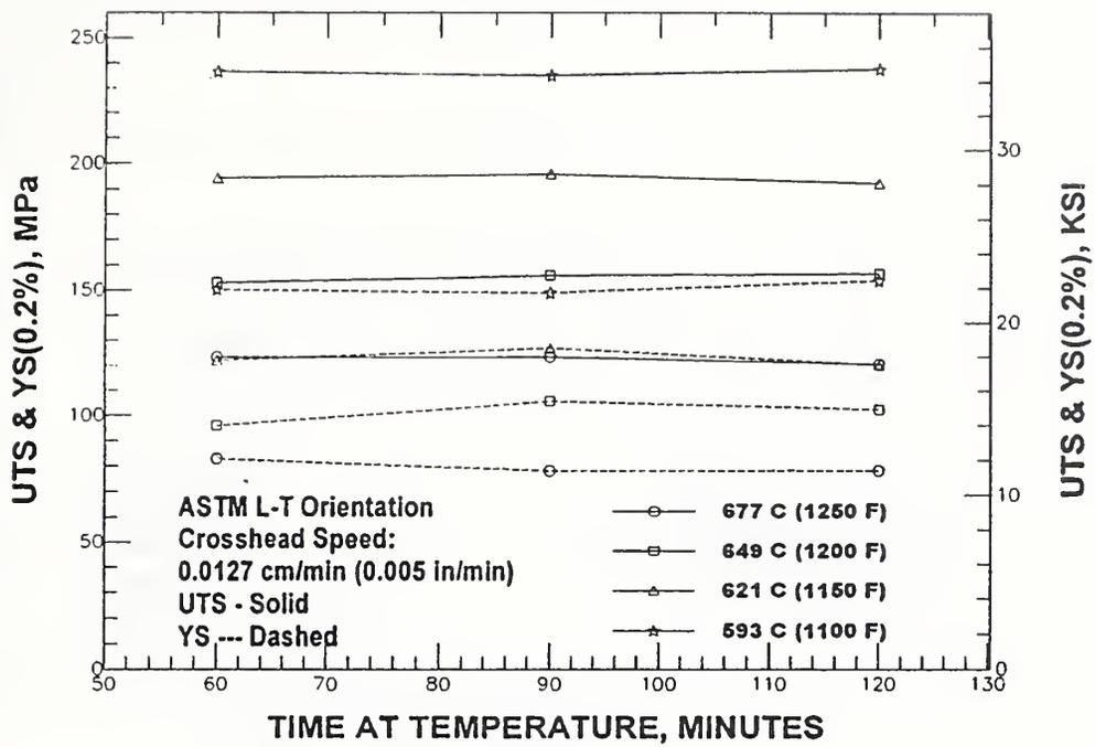
Figure 14. UTS and YS results for specimens tested at a crosshead speed of 0.0127 cm/minute and taken from the ASTM L-T direction in the plate.
