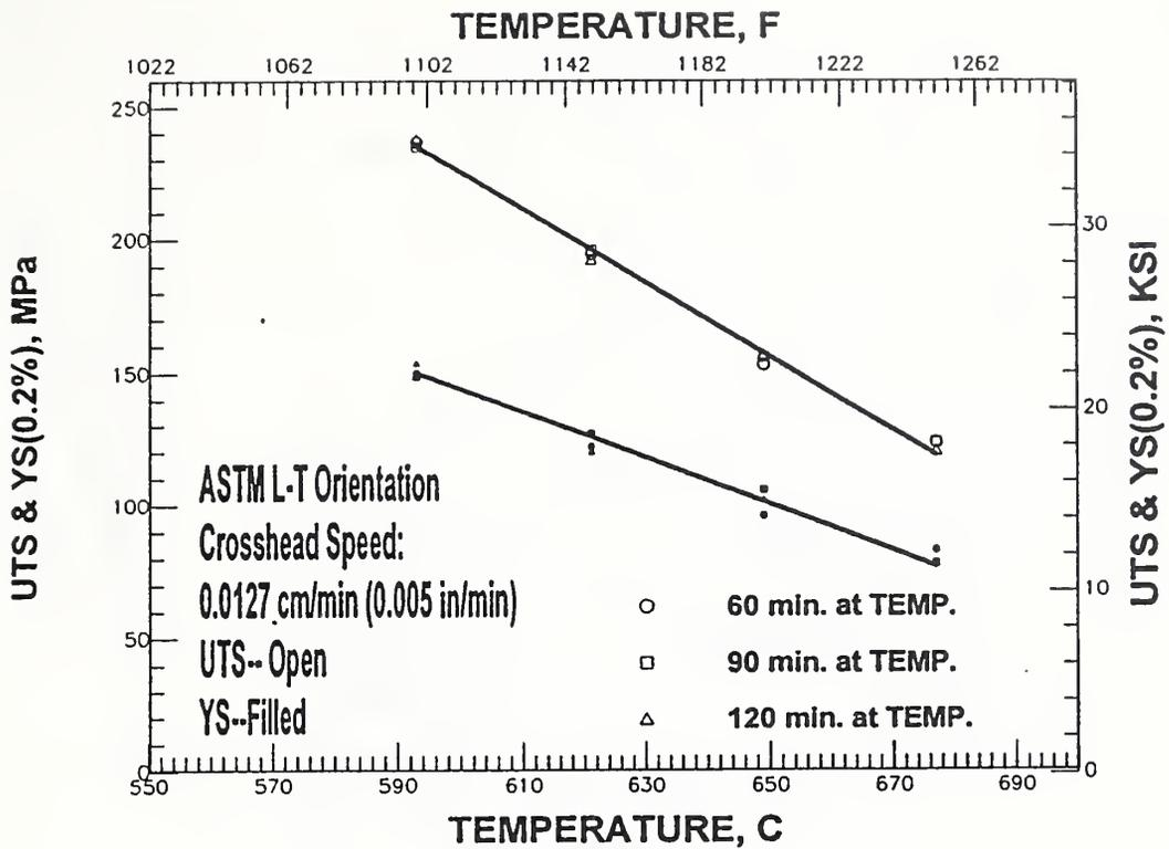
Figure 22. UTS and YS as a function of temperature. Specimens were taken from the ASTM L-T direction in the plate and tested at a crosshead speed of 0.0127 cm/minute.
