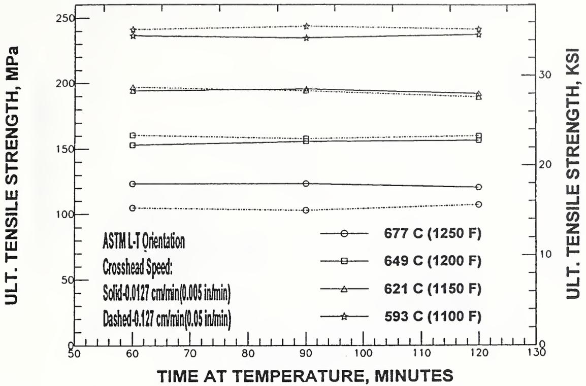
Figure 18. Affects of crosshead speed, temperature, and time on the UTS. Specimens were taken from the ASTM L-T direction in the plate.
