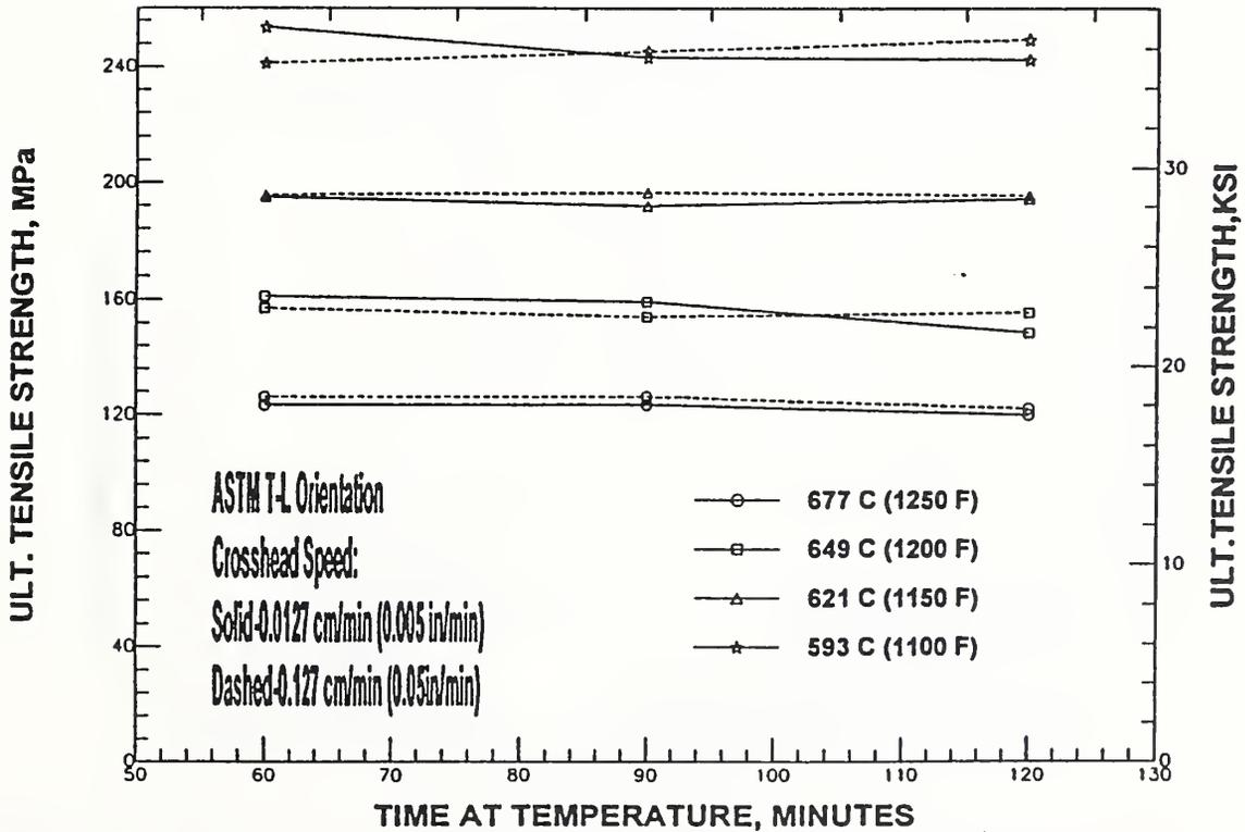
Figure 19. Affects of crosshead speed, temperature, and time on the UTS. Specimens were taken from the ASTM T-L direction in the plate.
