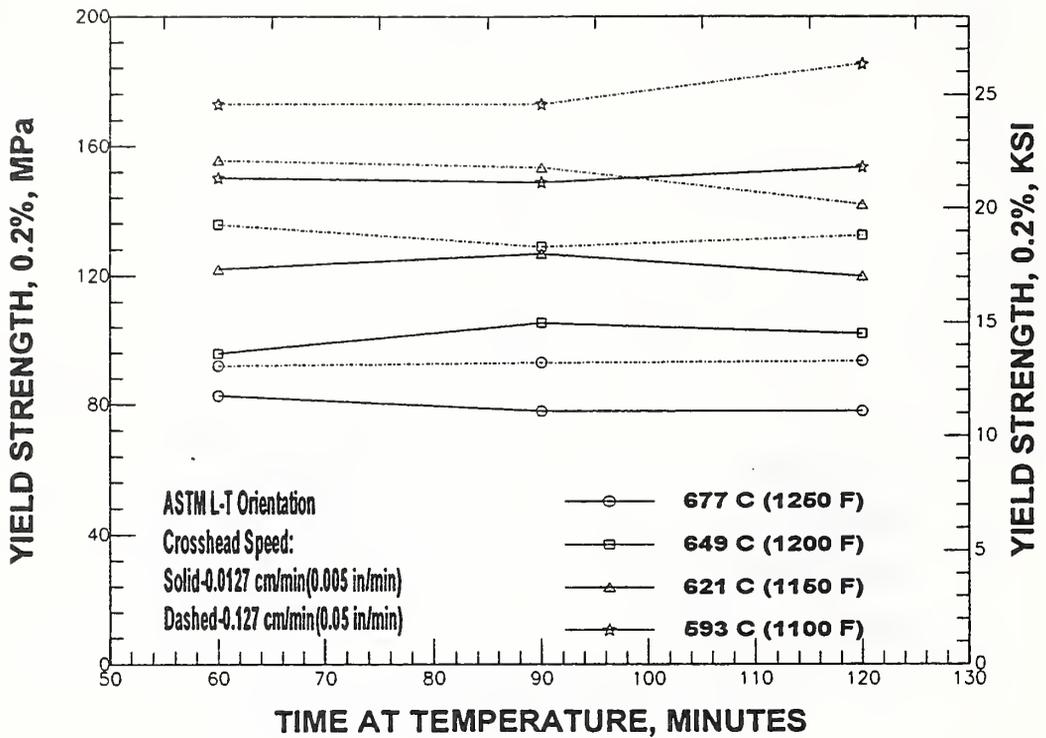
Figure 20. Affects of crosshead speed, temperature, and time on the YS. Specimens were taken from the ASTM L-T direction in the plate.
