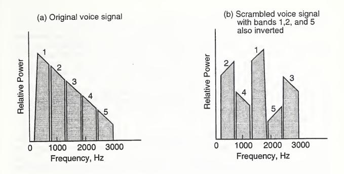
Figure 2. Scrambling by bandsplitting combined with inversion.
