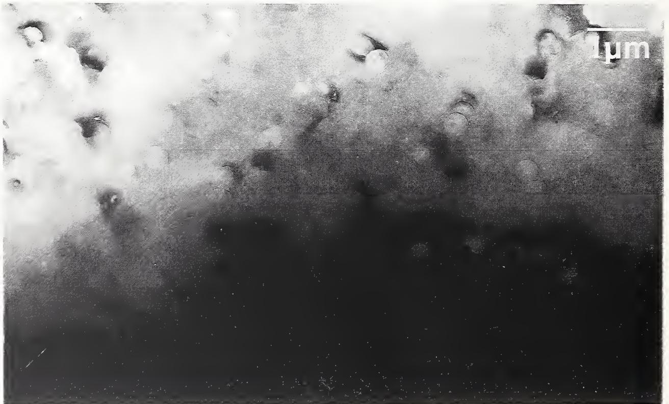
Figure 7c. (top) Type 3 texture on an MCE replica.
