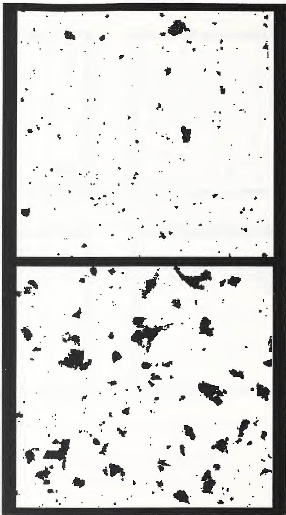
Figure 15 a-d. Particle loadings on grid squares (interior of grid squares is  $\sim 90 \mu\text{m}$  in width); (a) (top) particles comprise 3 percent of grid square area, (b) (bottom) particles comprise 10 percent of grid square area (continued next page).
