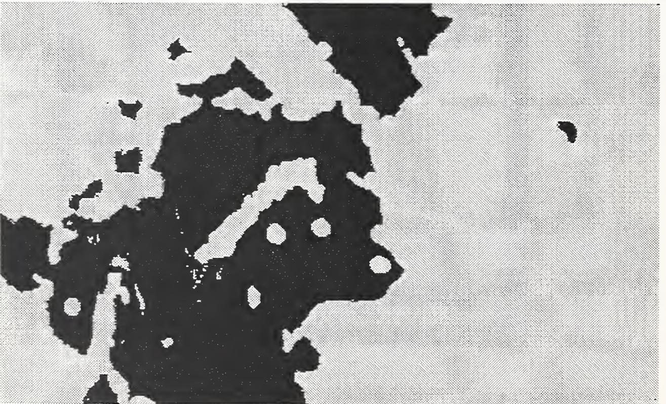
Figure 16. Image of overlapping replica on a PC filter replica (top). The overlapping replica covers 32 percent of the total image (black areas in bottom image).
