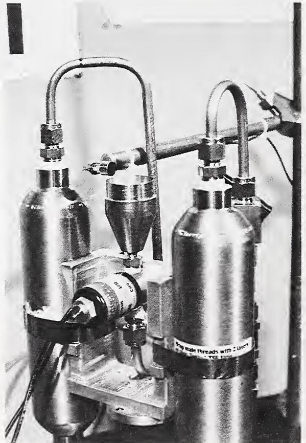
Fig. 3.7: (RIGHT) Close-up side view of solenoid-based RCS unit with acoustic sensor ready for pulse width resolution tests.
