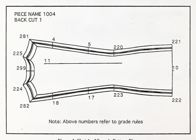
Figure 1: Sketch of Sample Pattern Piece
