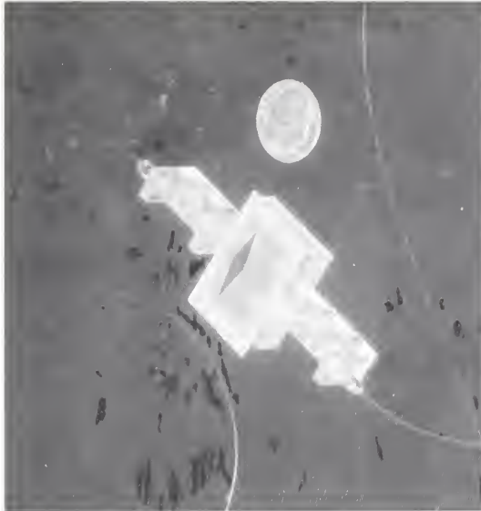
Integrated resistively tapered dipole and electrooptic modulator
