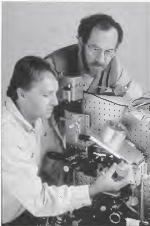
Norman Fontaine and Matt Young demonstrate the refracted ray scanning system for index of refraction profiling of optical waveguides.
