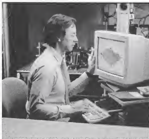
Nonlinear optical measurement system for nondestructive mapping of composition, strain, refractive index, and thickness in materials including lithium niobate and gallium nitride.
