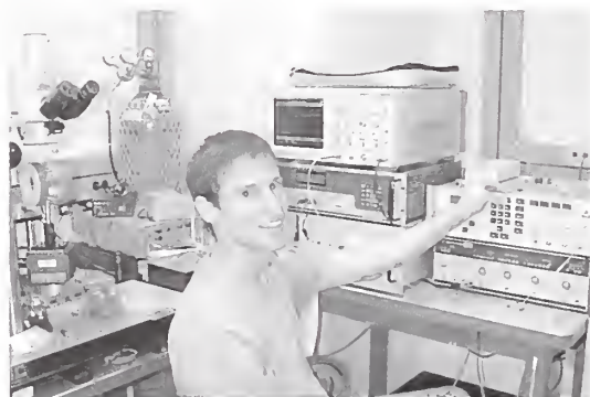
Unique high voltage, fast risetime pulse generators used in the project's magnetic switching studies are designed and built by electrical engineer Tony Kos. He also designs interfaces for computer control and data acquisition for the project's experiments.
