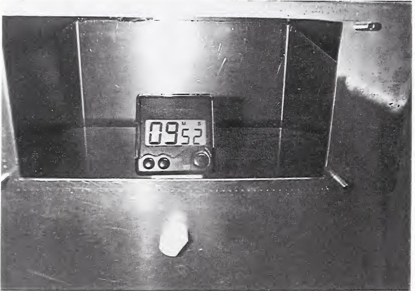
Figure 9. Closeup photograph of an electronic timer in a TEM cell.
