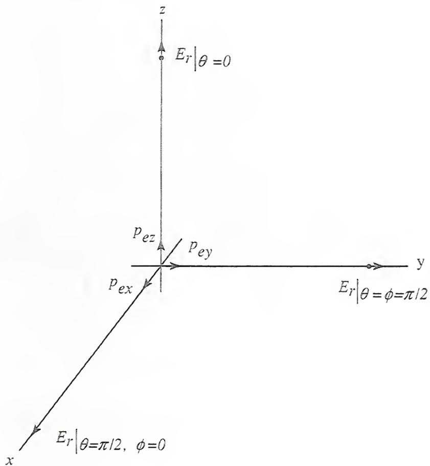
Figure 10. Geometry for electric dipoles at the origin and radial electric fields on the axes.
