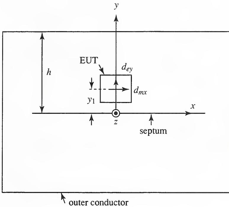
Figure 2. Cross-sectional view of an EUT with electric and magnetic dipole moments located above the septum in a TEM cell.
