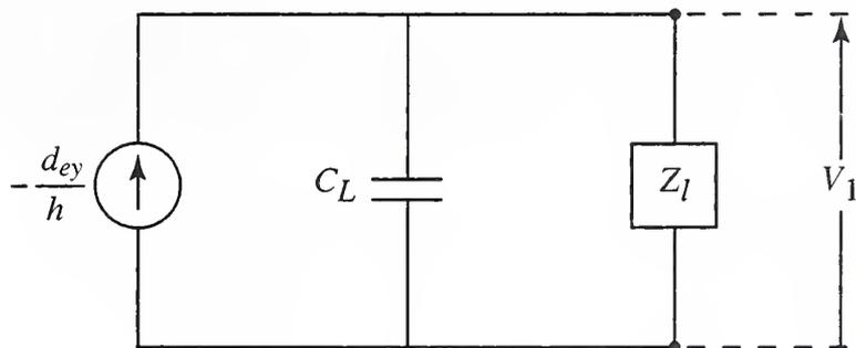
Figure 5. Equivalent circuit for an electric dipole source in an open-circuited TEM cell.
