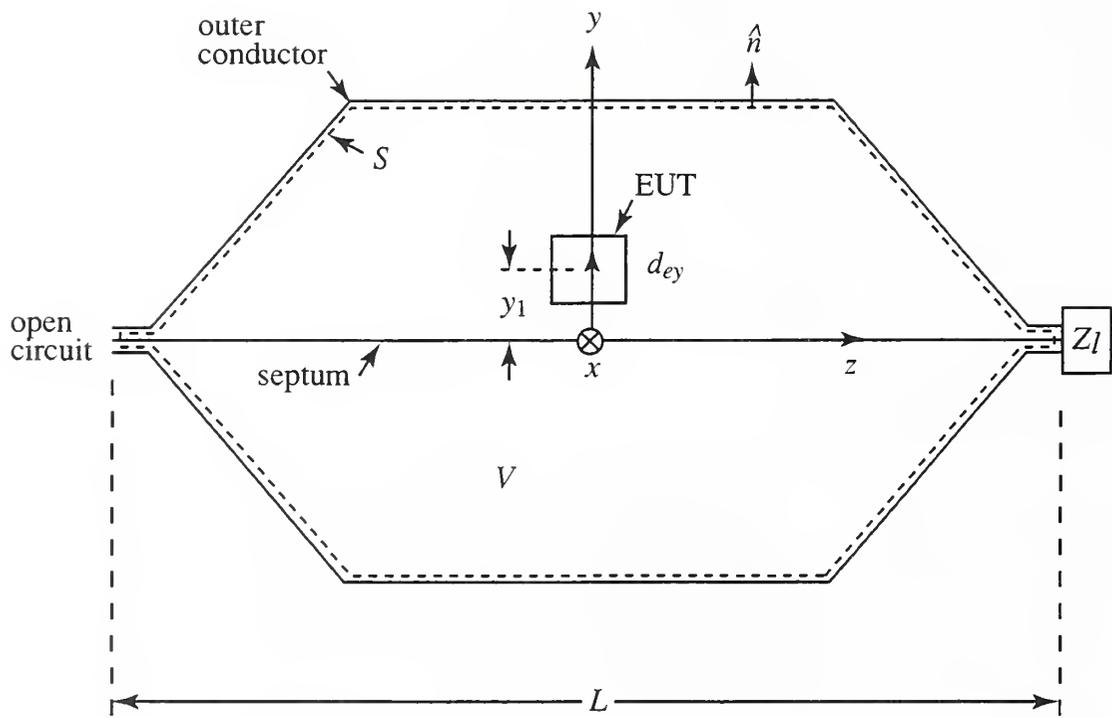
Figure 3. Side view of an EUT located above the septum in an open-circuited TEM cell.
