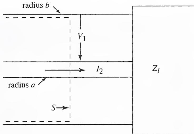
Figure 4. Impedance termination of the coaxial section of a TEM cell.
