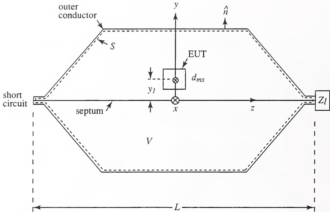
Figure 6. Side view of an EUT located above the septum in a short-circuited TEM cell.
