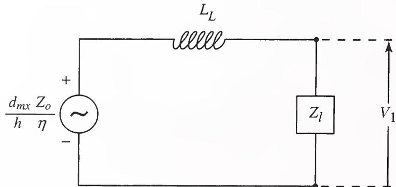
Figure 7. Equivalent circuit for a magnetic dipole source in a short-circuited TEM cell.
