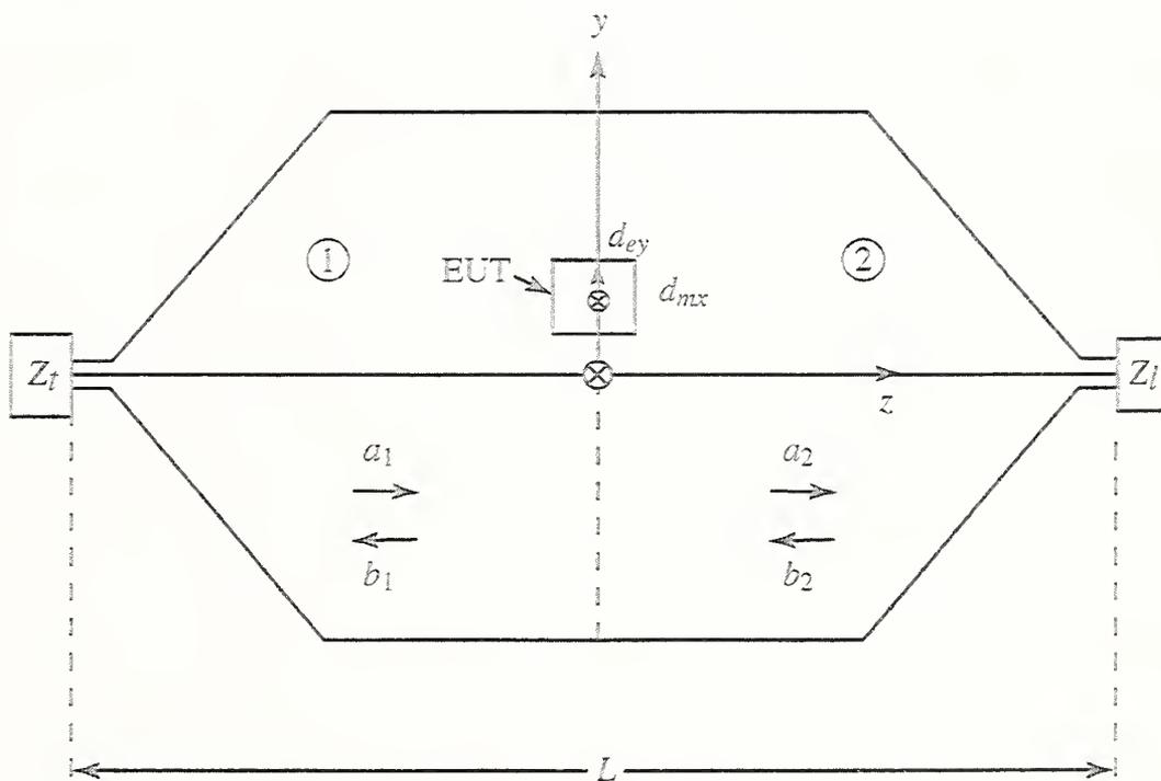
Figure 12. Side view of an EUT located in a TEM cell with arbitrary terminations.
