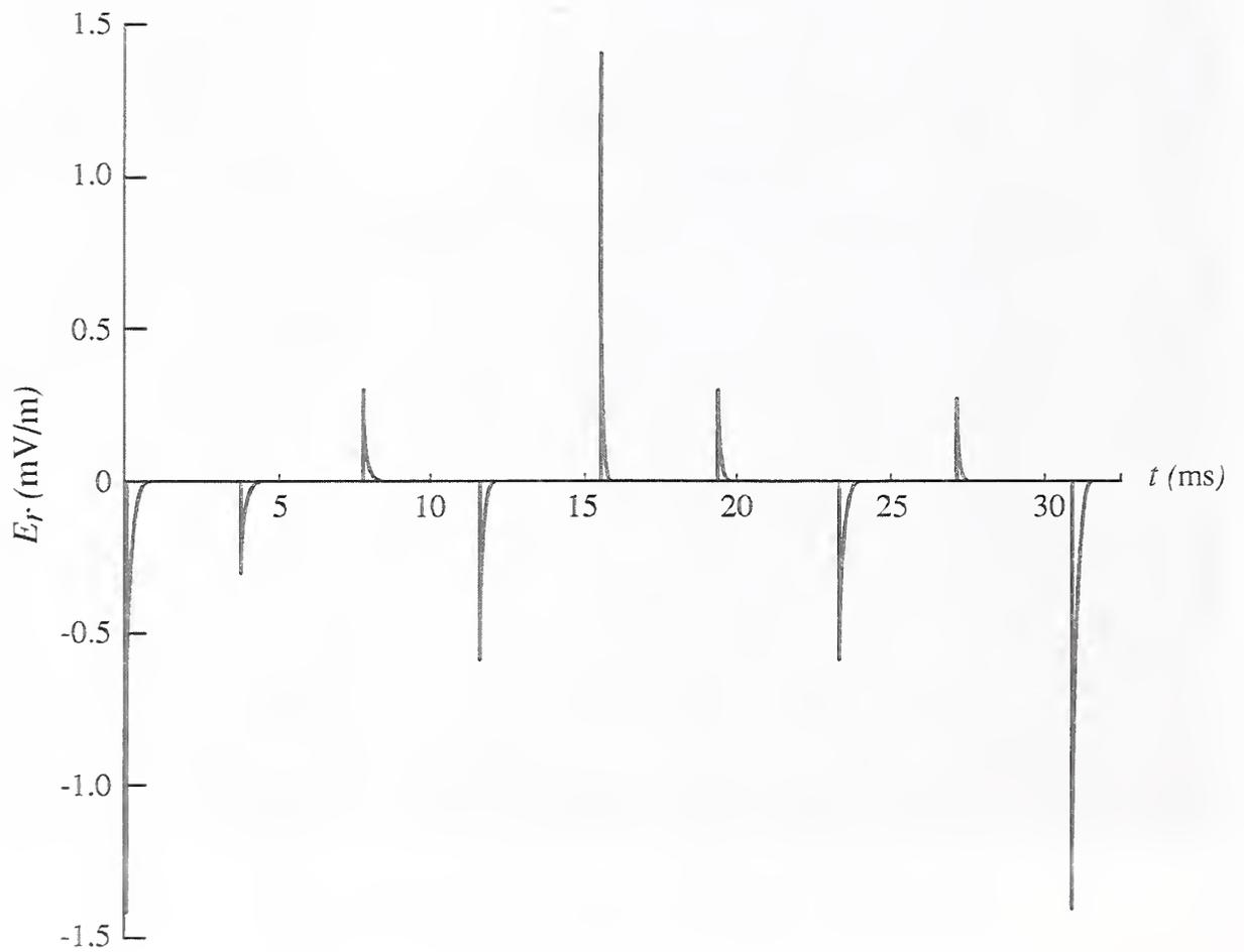
Figure 11. Time-domain waveform for the radial electric field at 1 m from an electronic timer.
