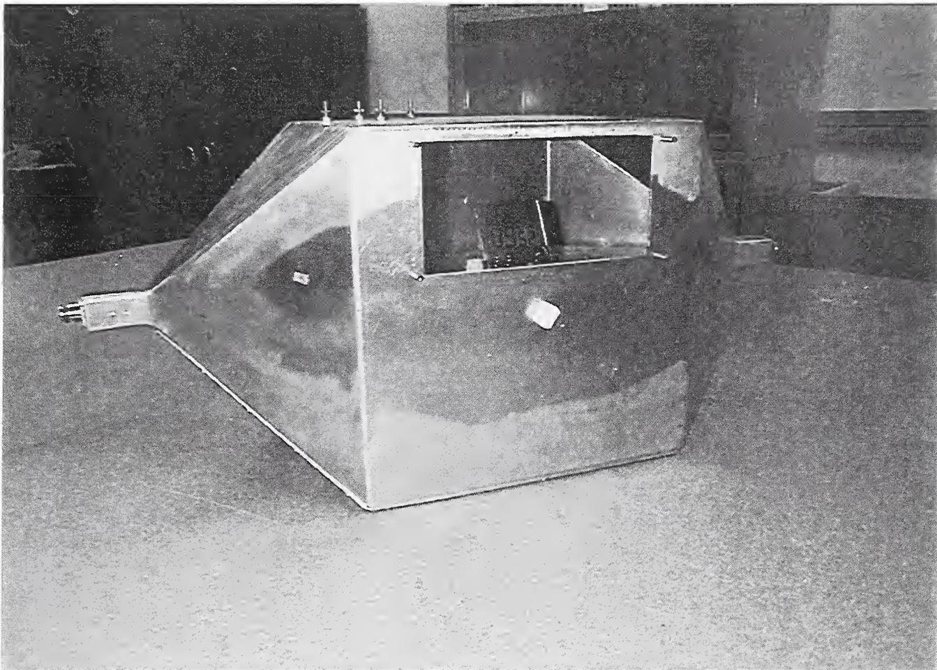
Figure 8. Photograph of an electronic timer in a TEM cell.
