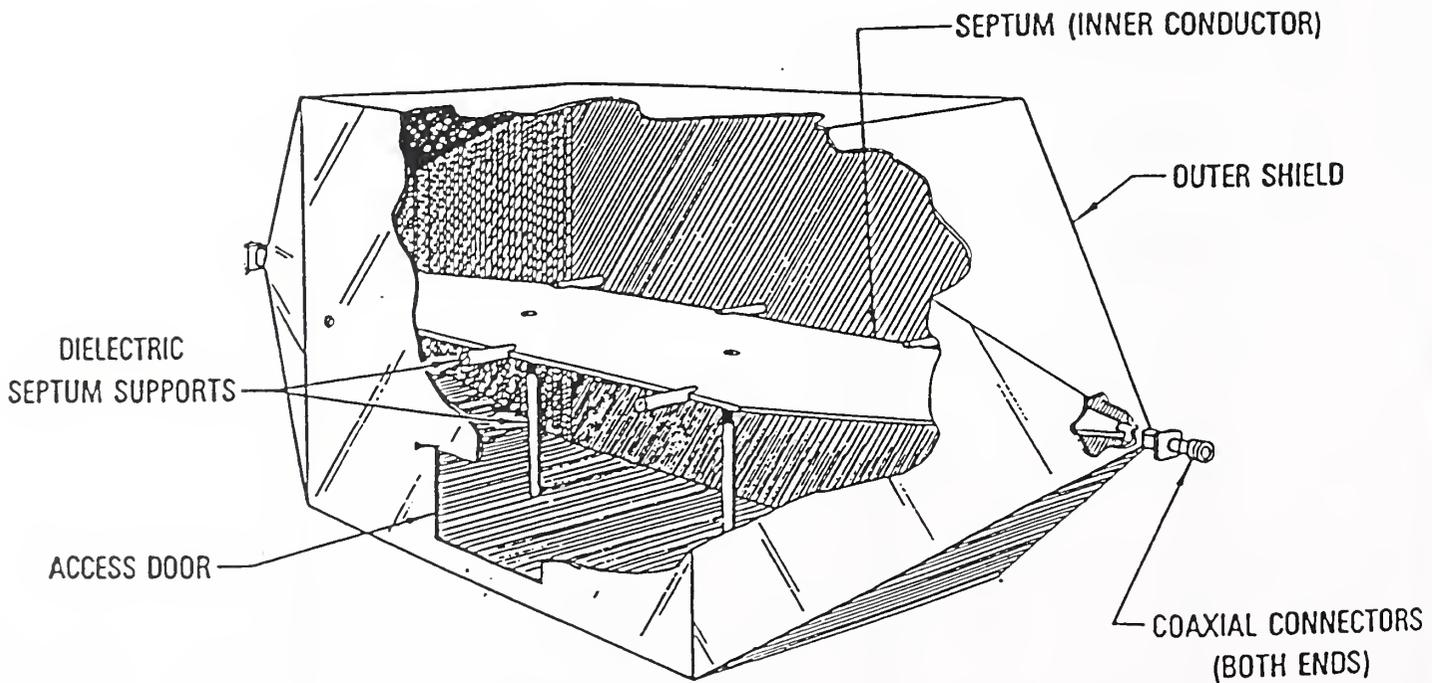
Figure 1. Geometry for a TEM cell.
