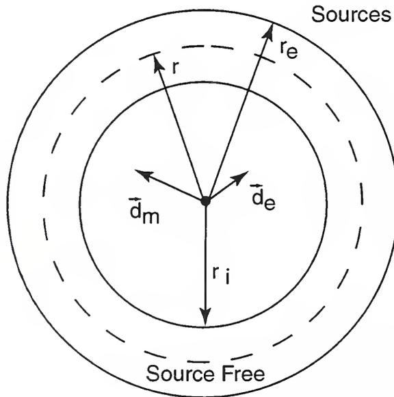
Figure 4. Geometry for a measurement sphere of radius  $r$  with equivalent electric and magnetic dipoles located inside a sphere of radius  $r_i$  and exterior sources located outside a sphere of radius  $r_e$ .
