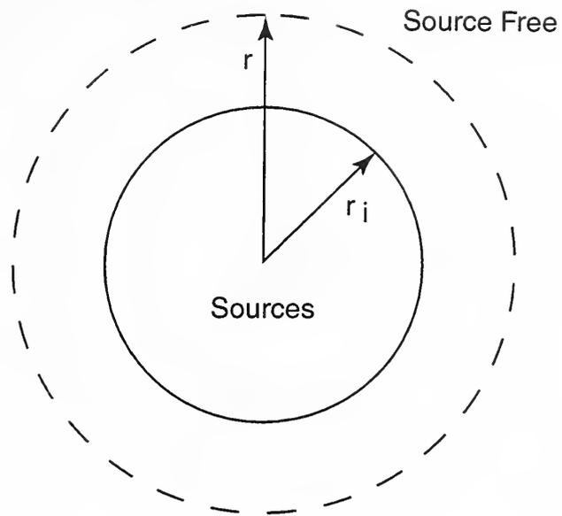
Figure 1. Geometry for a measurement sphere of radius  $r$  with sources located inside a sphere of radius  $r_i$ .
