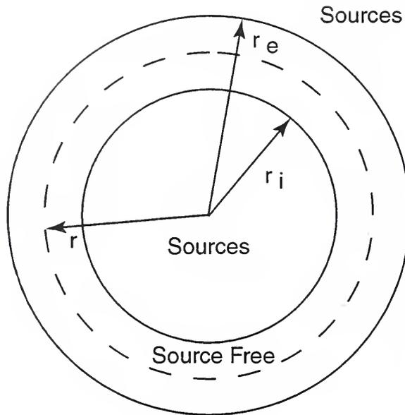
Figure 3. Geometry for a measurement sphere of radius  $r$  with sources located inside a sphere of radius  $r_i$  and outside a sphere of radius  $r_e$ .
