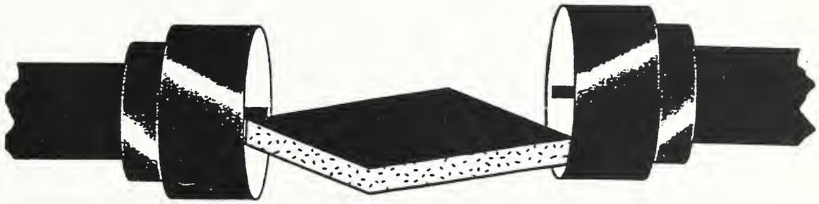
Figure 1. Coupling schematic between 7 mm coaxial connectors and a copper-clad dielectric substrate.
