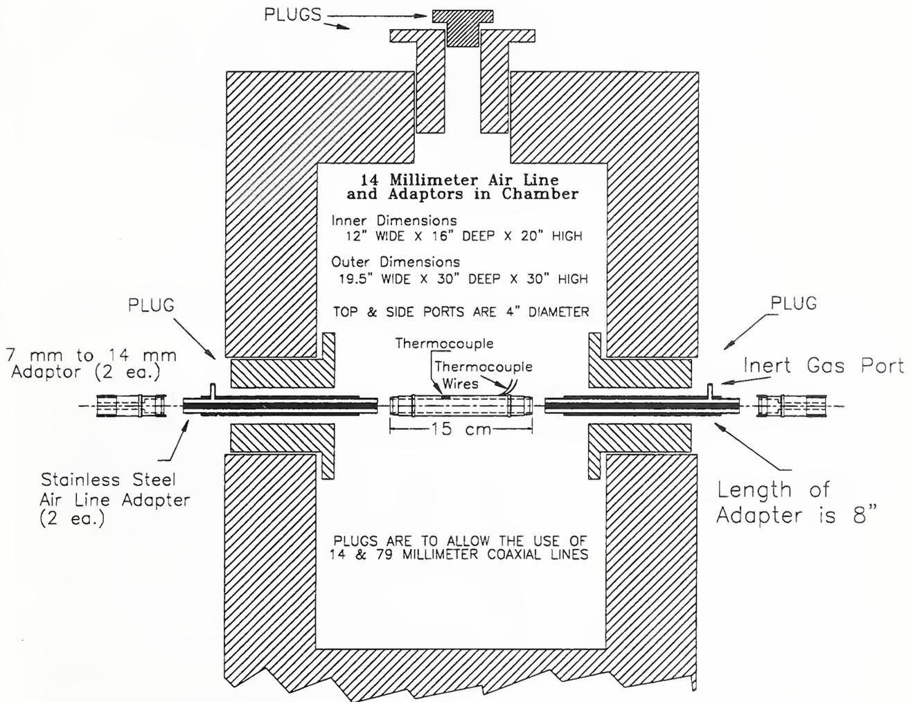
Figure 2: Two-port system with environmental chamber.
