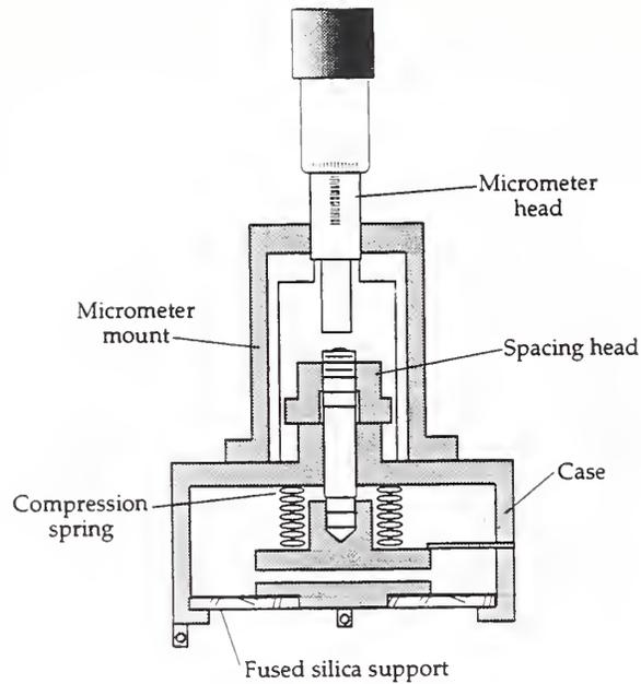
Figure 5: Capacitance dielectrometer.
