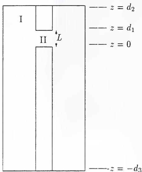
Figure 6: A doubly reentrant cavity. The sample resides between the parallel plates in region II.
