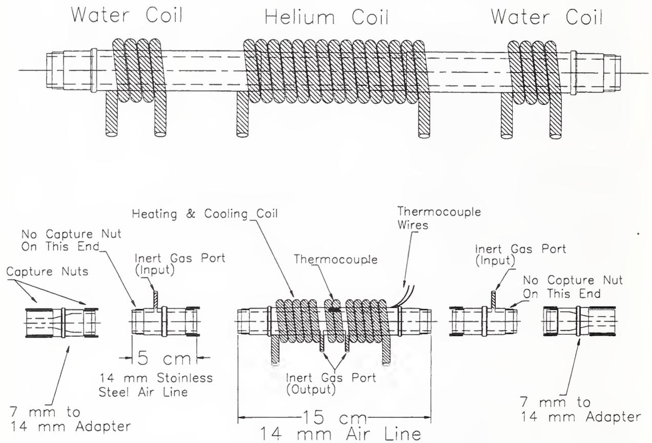
Figure 1: Two-port coaxial fixture for elevated temperatures. The fixture maintains temperature control by heating and cooling coils. Also depicted is the coaxial line setup with feedlines and connectors.
