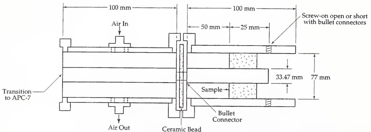
Figure 3: One-port coaxial fixture for elevated temperatures. The end of the fixture would be inserted into an access hole in an environmental chamber.
