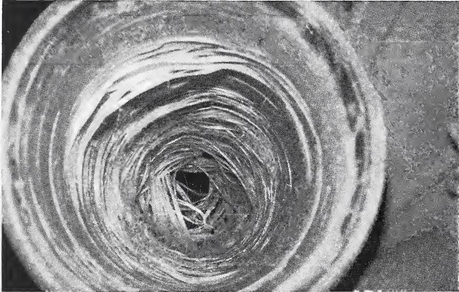
Figure B.14. Internal hoop-ply delamination (tube type 18) at 76 K.
