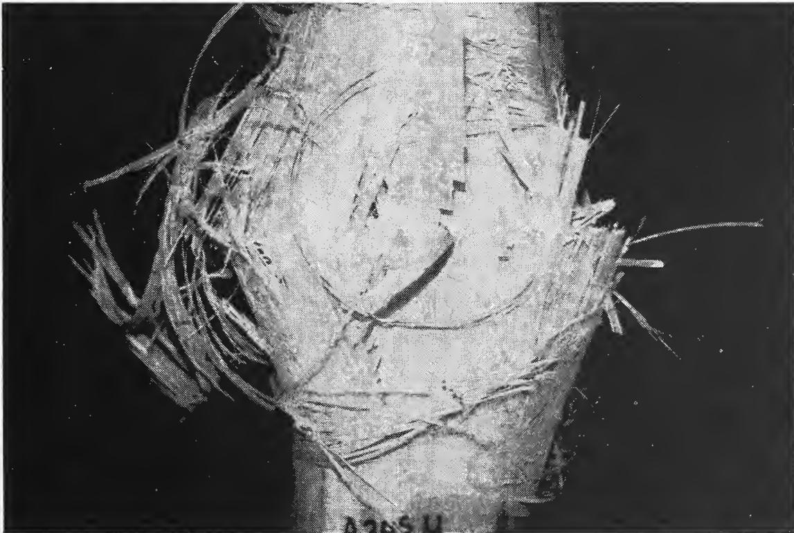
Figure B.13. Failure in tube type 5 at 4 K.
