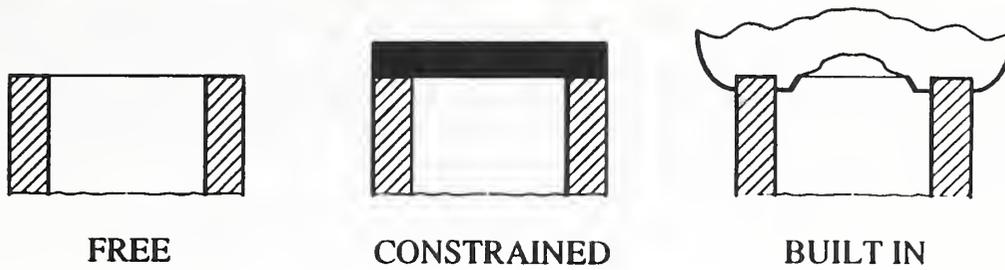
Figure 2.2. Conditions at the edges of the cylinder.
