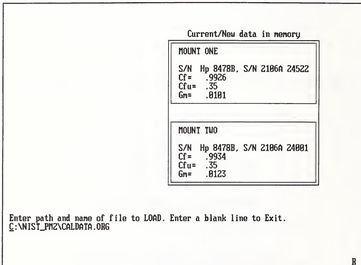
Figure 2.6. Mount selection screen when loading a CALDATA file.
