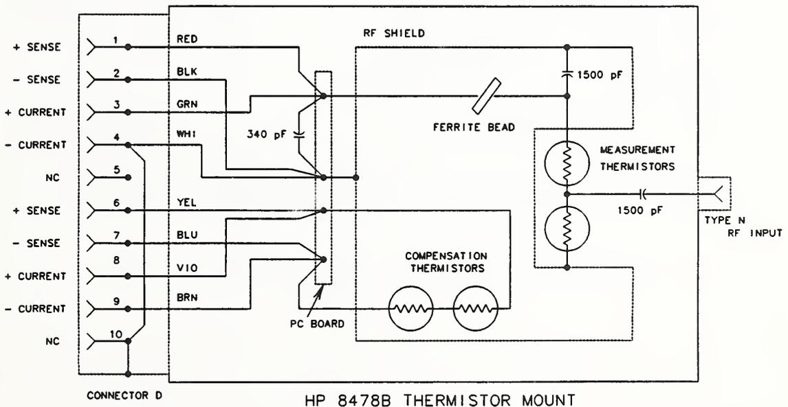
Figure 3.4. Modified mount wiring.
