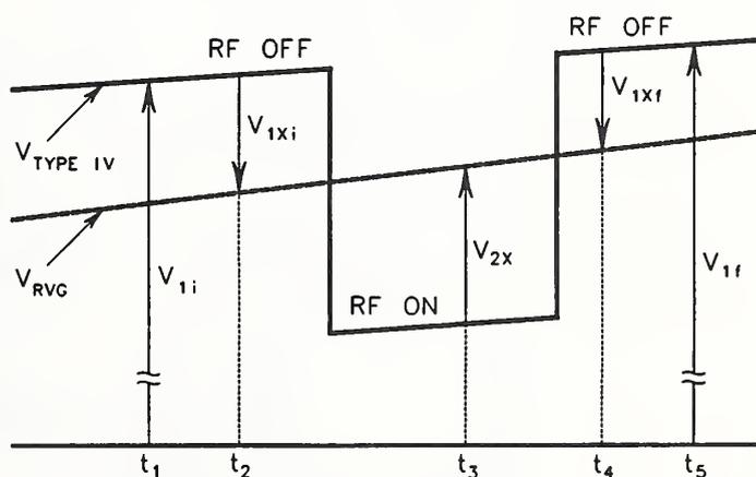
Figure 3.1. Measured power meter voltages vs time.
