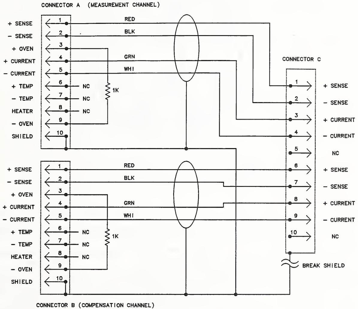
Figure 3.6. Thermistor mount connecting cable wiring diagram.
