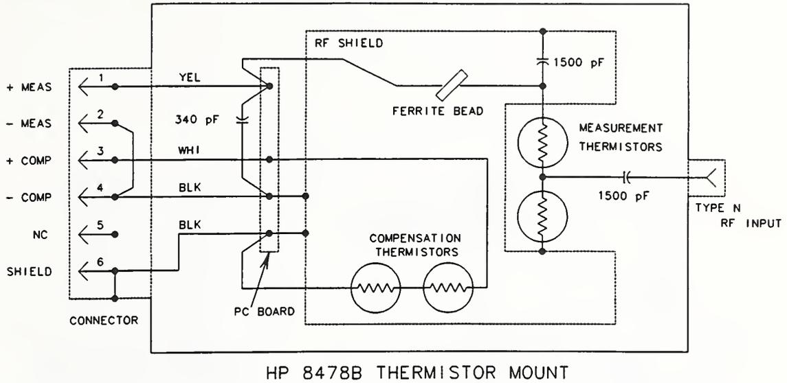
Figure 3.3. Original mount wiring.
