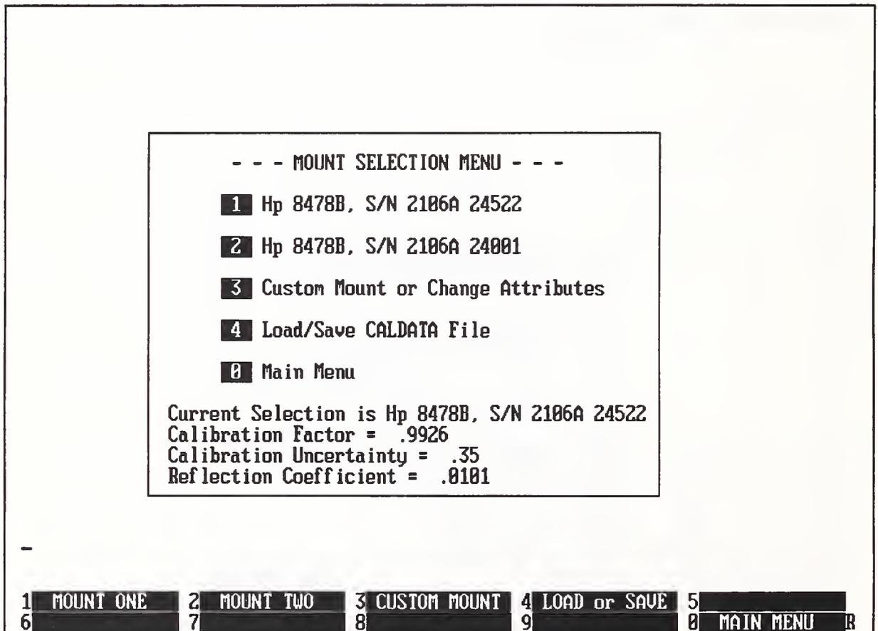
Figure 2.2. Screen display of the mount selection menu.
