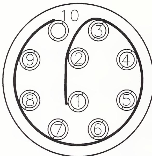
Figure 3.7. Connector pin-out (Male cable connector as seen from cable end).
