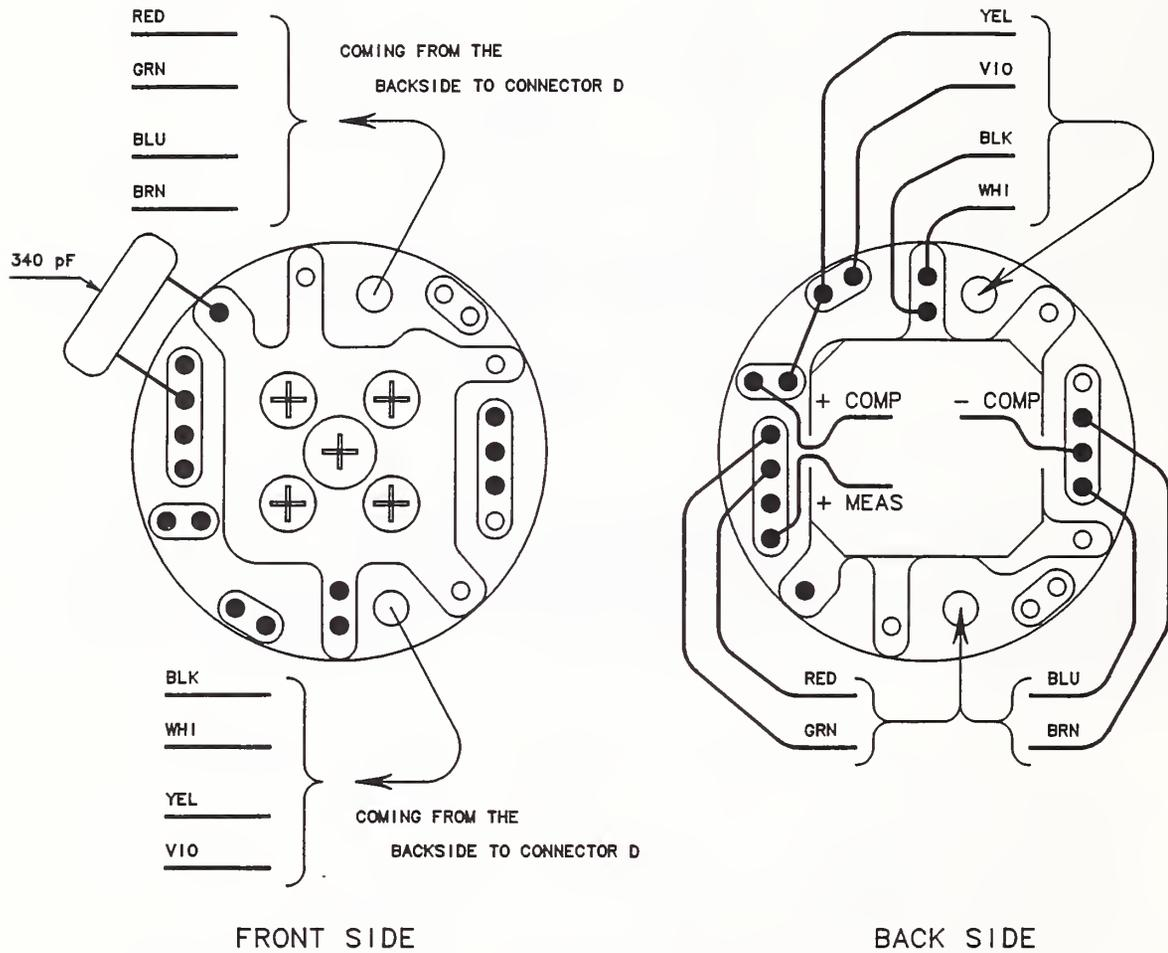
Figure 3.5. HP 8478B thermistor mount pc board layout with modified wiring.
