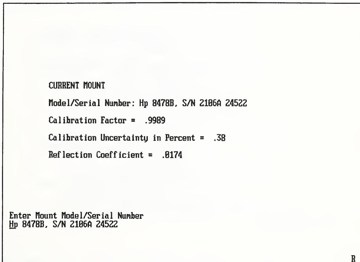
Figure 2.3. Screen display for changing stored calibration data.
