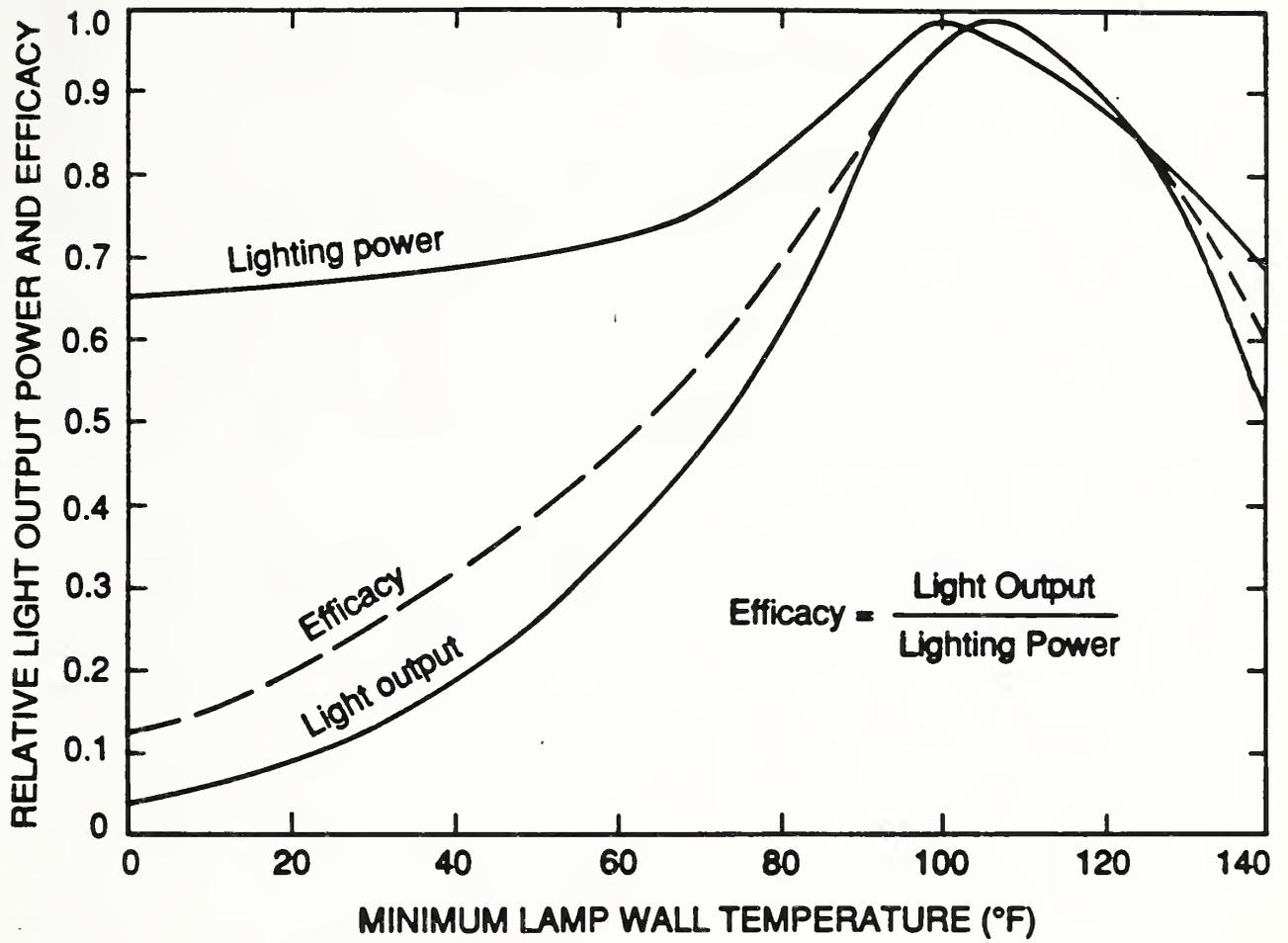
Figure 1. Dependence of Lamp Functions on Lamp Wall Temperature
