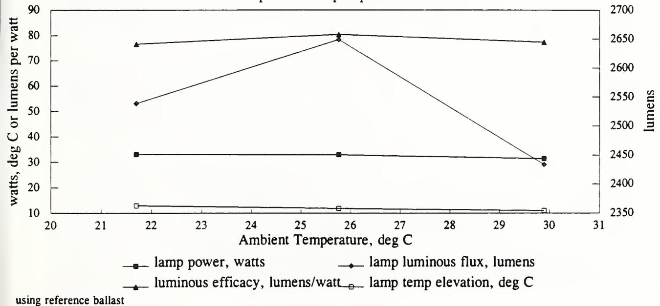
Figure 10. Measured Performance versus Ambient Temperature for Lamp #4.
