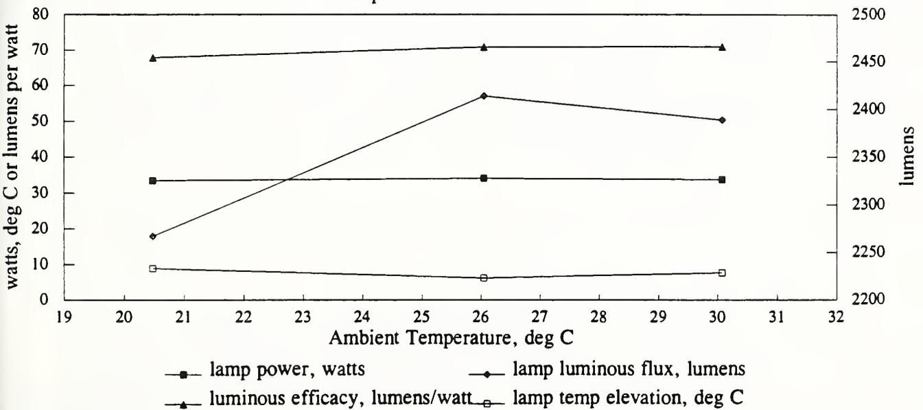
Figure 8. Measured Performance versus Ambient Temperature for Lamp #2.
