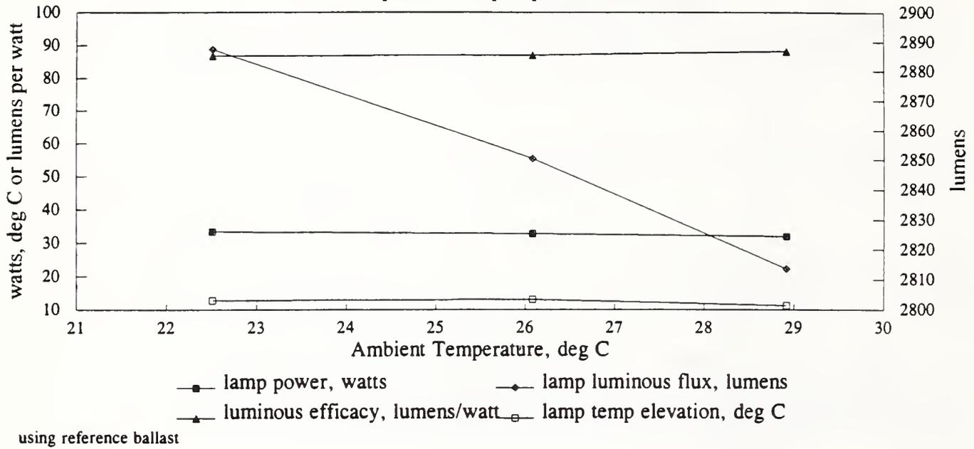
Figure 11. Measured Performance versus Ambient Temperature for Lamp #5.
