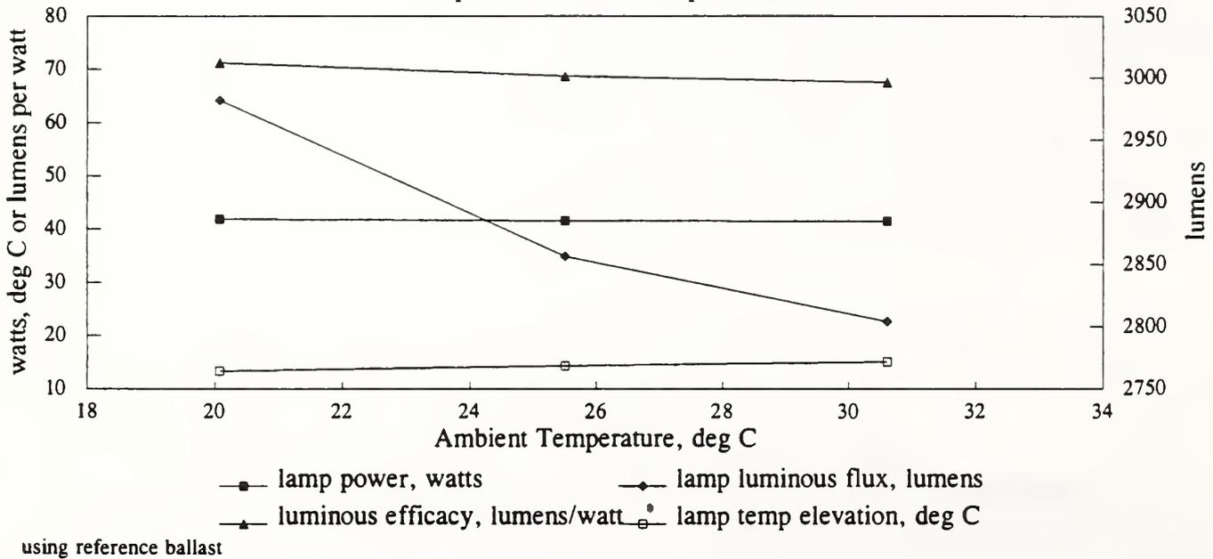
Figure 12. Measured Performance versus Ambient Temperature for Lamp #6.
