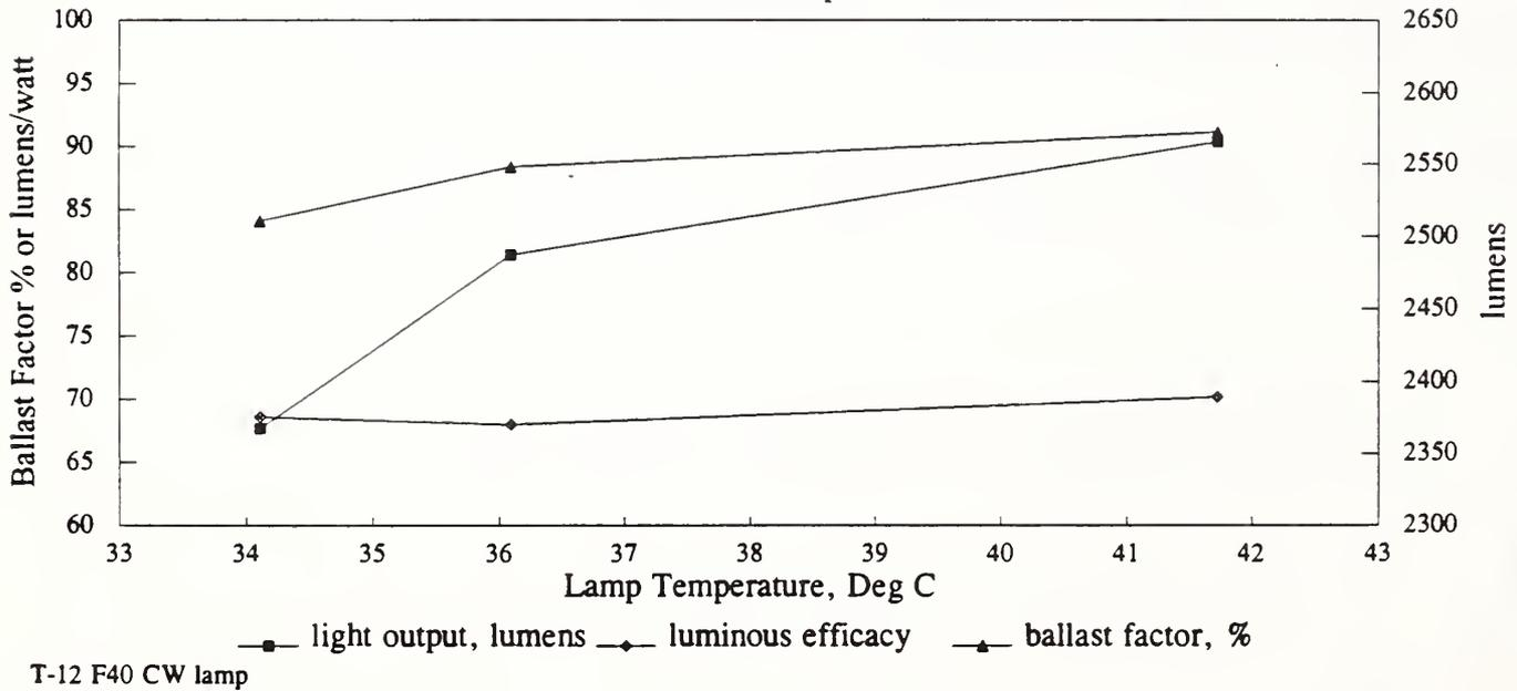
Figure 14. Measured Performance of Ballast 4 with Lamp #3.
