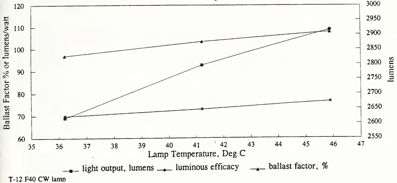
Figure 15. Measured Performance of Ballast 4 with Lamp #4.
