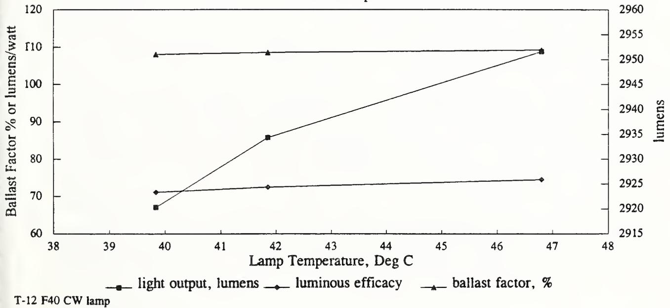
Figure 16. Measured Performance of Ballast 5 with Lamp #4.
