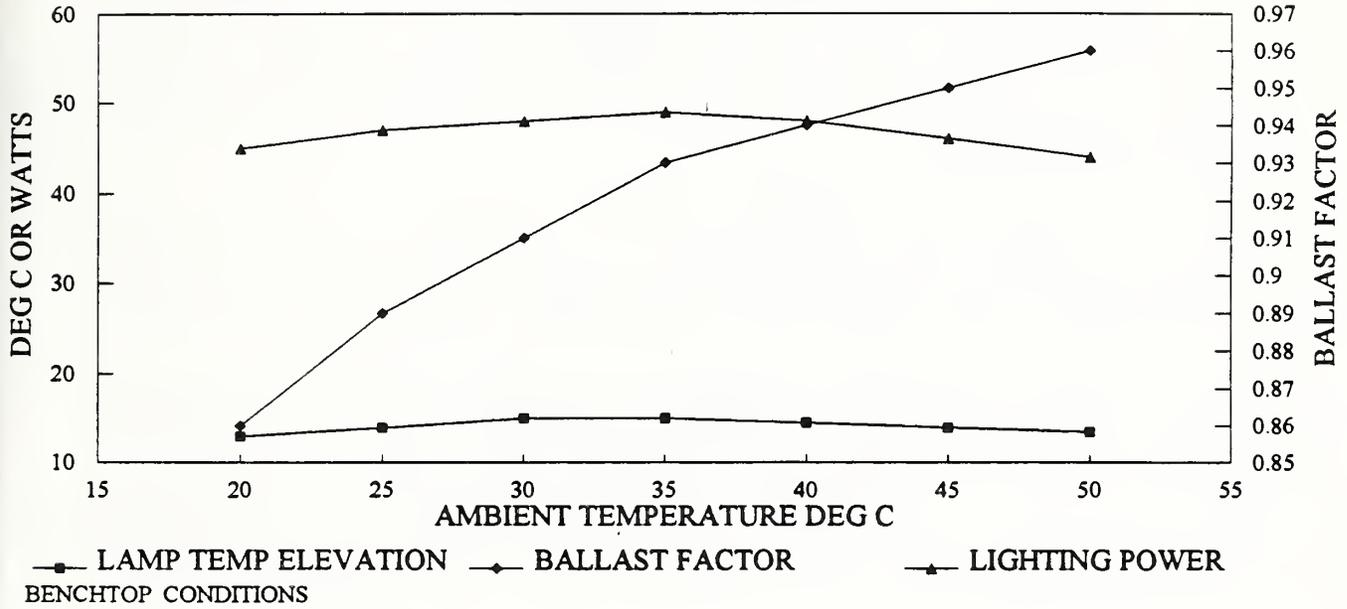
Figure 3. Typical Data for Ballast Factor, Ballast Power Ratio, and Ballast Temperature Ratio.
