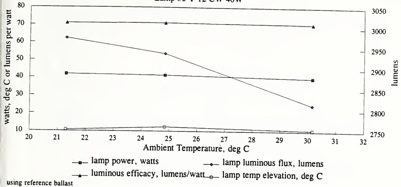
Figure 9. Measured Performance versus Ambient Temperature for Lamp #3.
