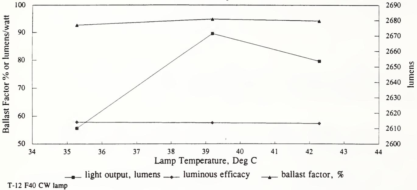
Figure 13. Measured Performance of Ballast 1 with Lamp #3.
