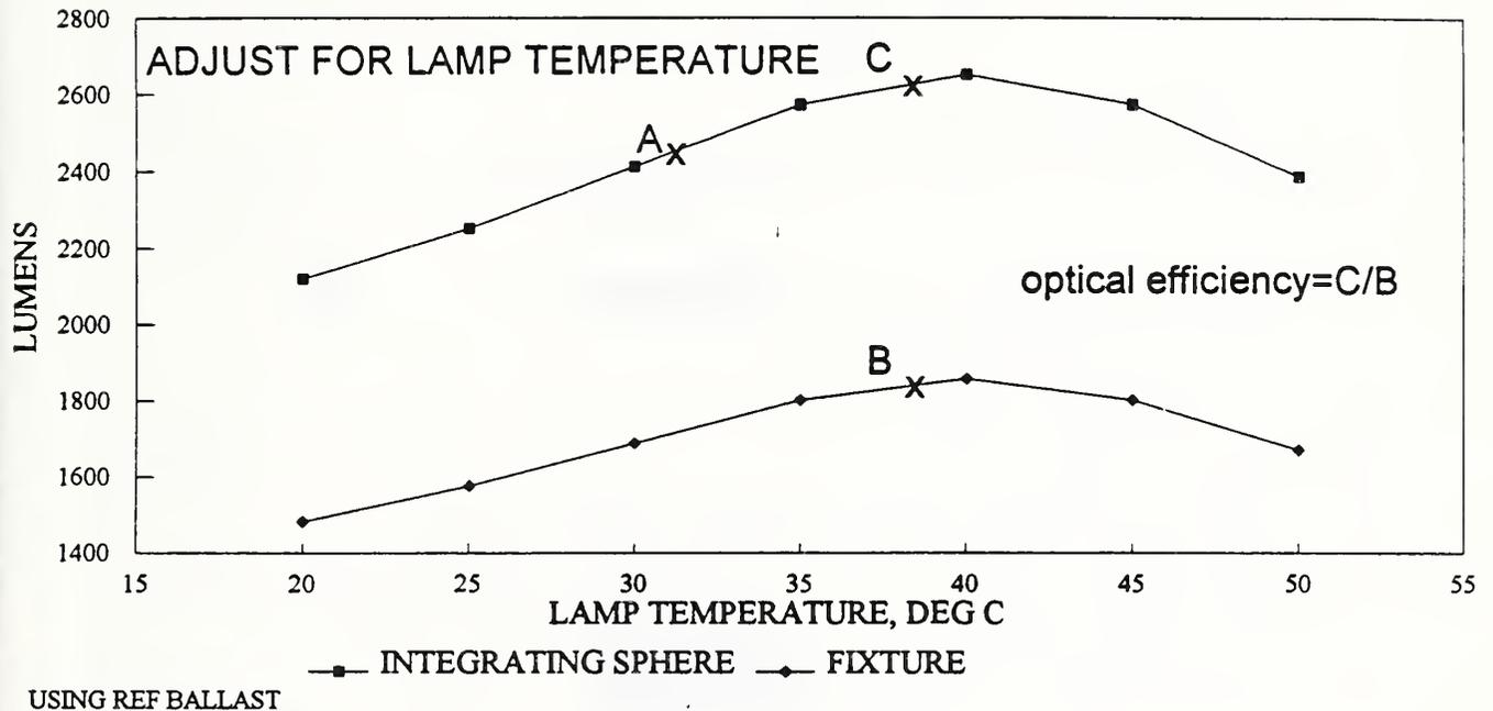
Figure 4. Procedure for Determining Fixture Optical Efficiency.
