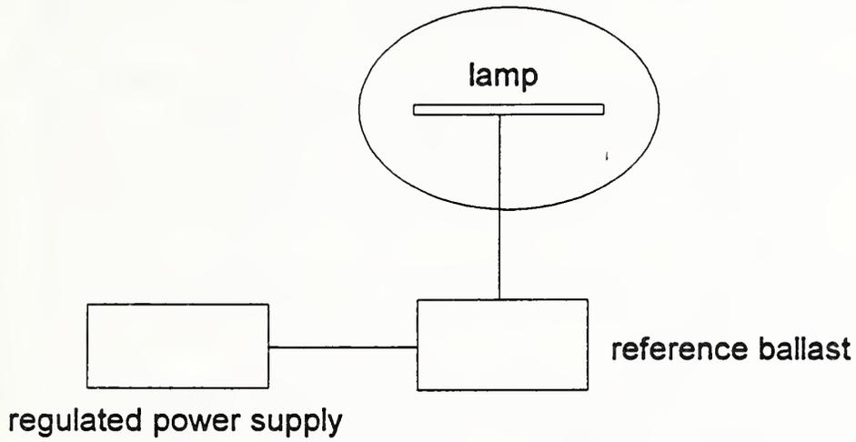
Figure 6. Schematic Approach for Measuring Lamp Output.
