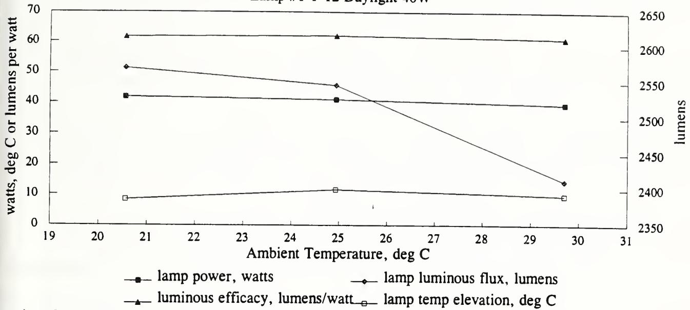
Figure 7. Measured Performance versus Ambient Temperature for Lamp #1.
