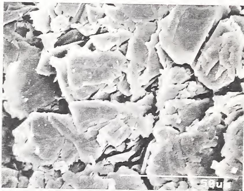
Fig. 6. SEM photograph of the morphology of the NiCl<sub>2</sub> - IG particles.
