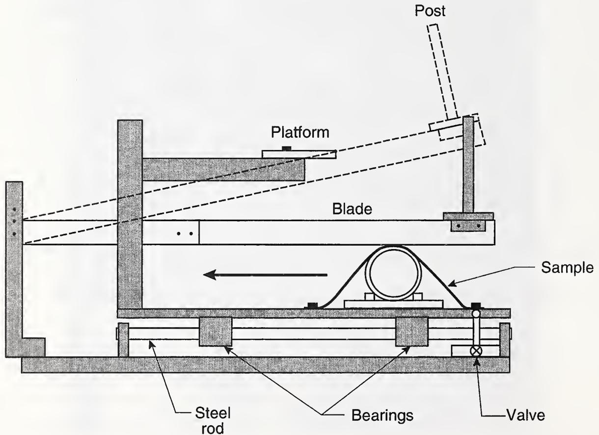
Figure 5. Sketch of slash test apparatus.
