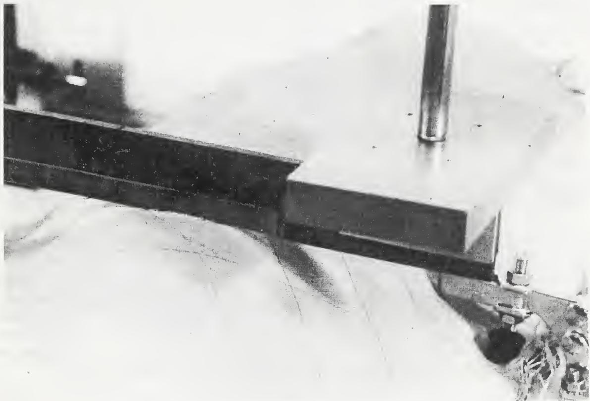
*Figure 8. Photograph of post used to add weight to slash test blade.*
