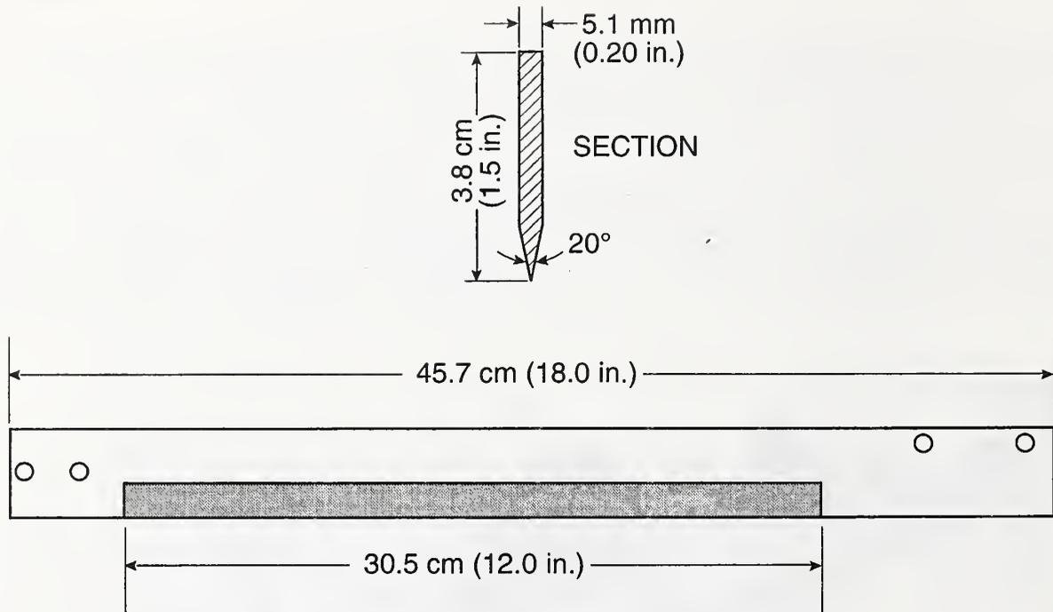
Figure 7. Sketch of slash test blade.
