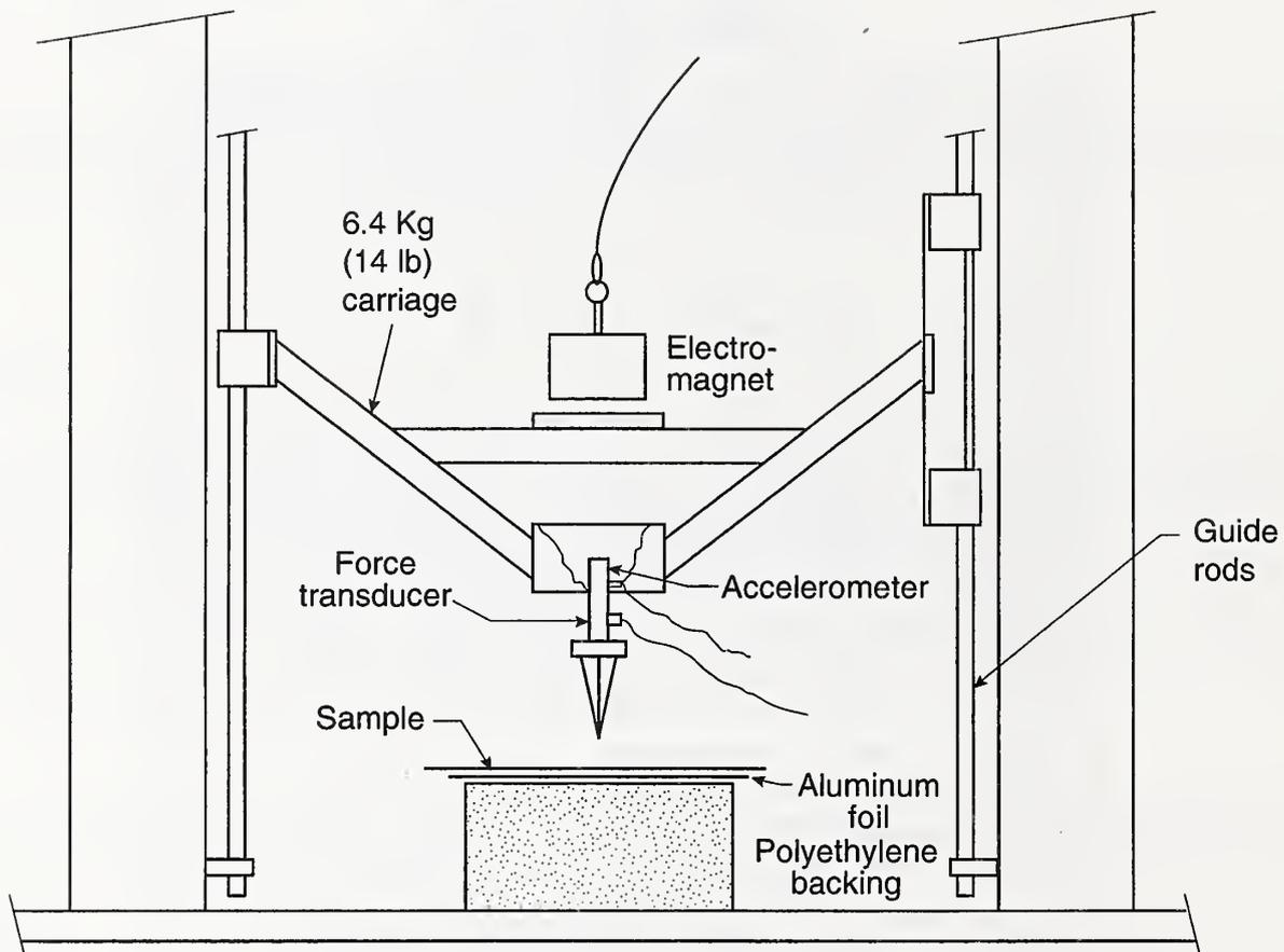
Figure 1. Sketch of free fall test apparatus
