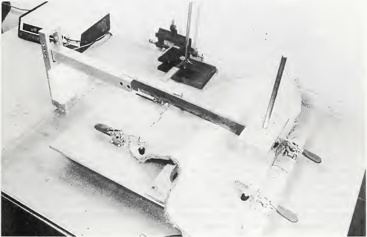
*Figure 6. Photograph of slash test apparatus.*
