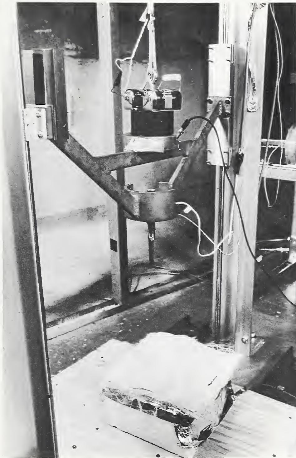
*Figure 2. Photograph of carriage suspended above sample by electromagnet.*
