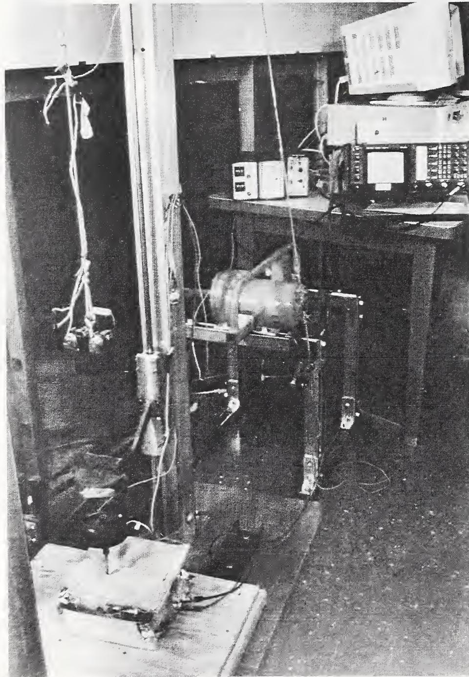
*Figure 3. Photograph of overall apparatus used for stab penetration testing.*
