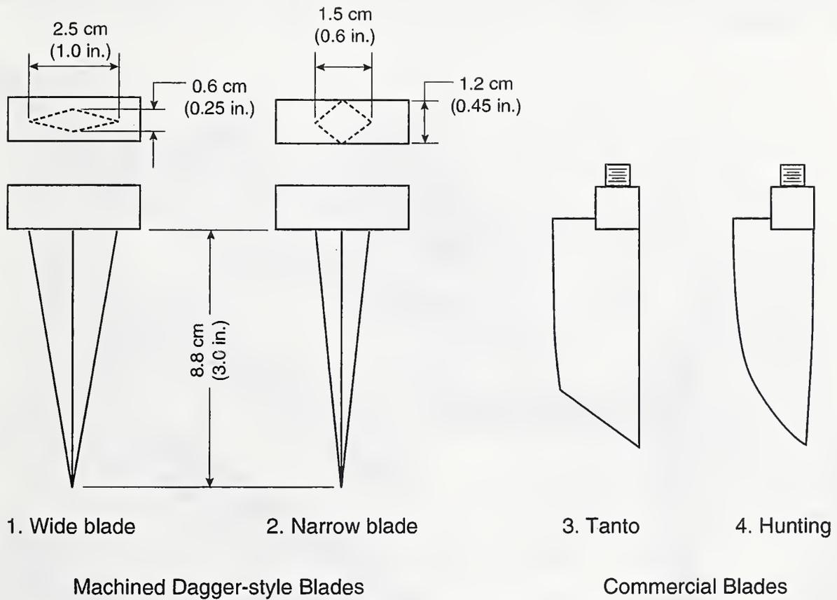
Figure 4. Test penetrators.
