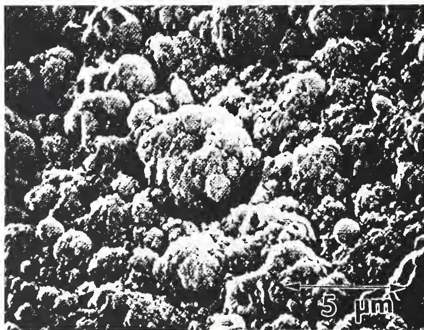
Figure 2. Microstructure of Nd/YAG-deposited PZT film (SEM).
