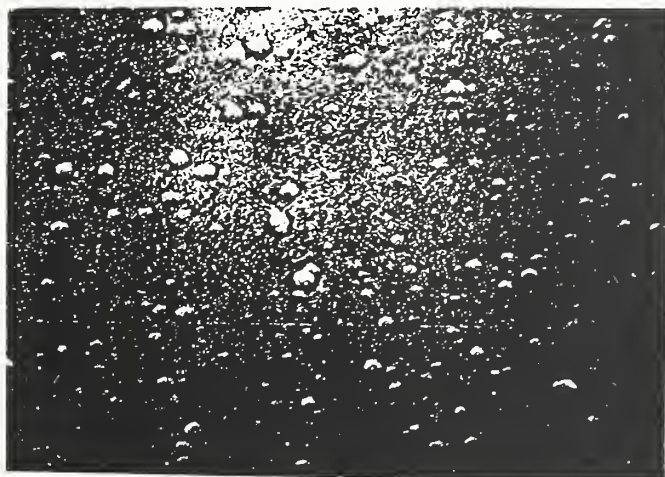
Figure 5 A SEM micrograph of a PZT film heat-treated at 550^\circ\text{C} .
