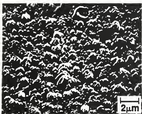
Figure 4 SEM micrograph of as-deposited line-of-sight film.
