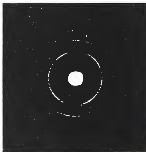
Fig. 4b Selected area electron diffraction from area in Figure 4a.
