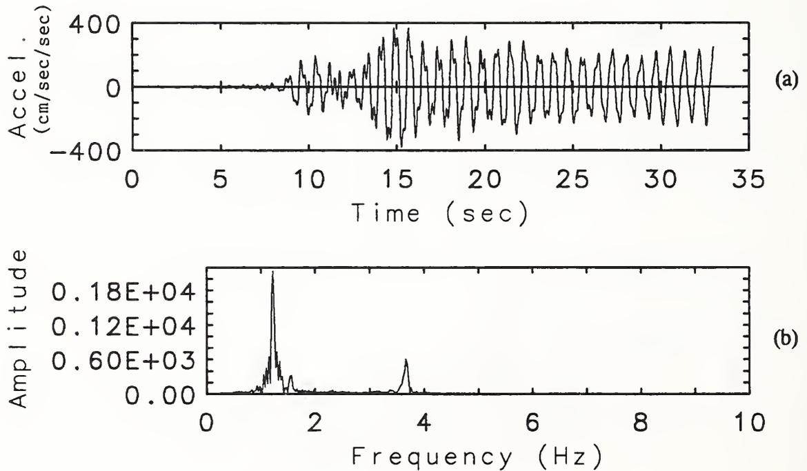
Figure 3.10 EW Acceleration-Time History at North End of Roof from the Fixed-Base Model with 0.5% Damping (a), and Corresponding Fourier Spectrum (b).
