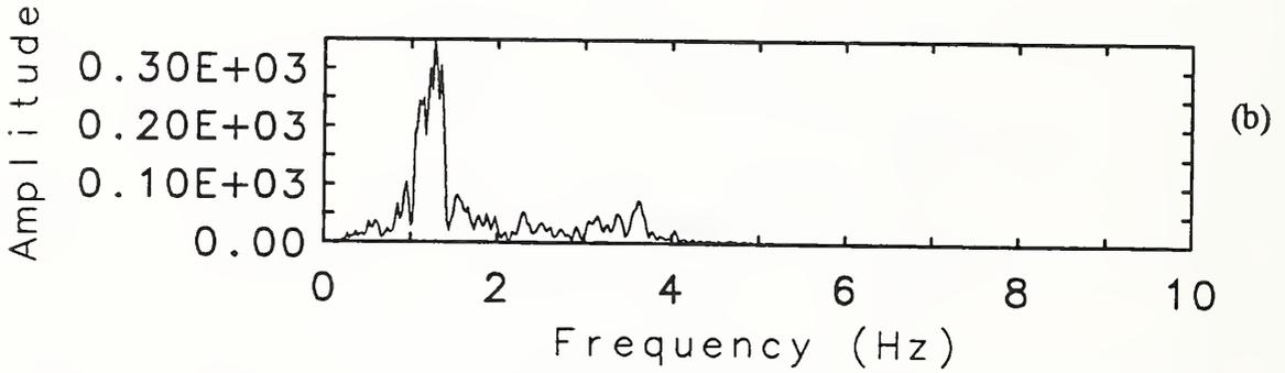
Figure 3.5 EW Acceleration-Time History at Center of Roof from the Fixed-Base Model with 7% Damping (a), and Corresponding Fourier Spectrum (b).
