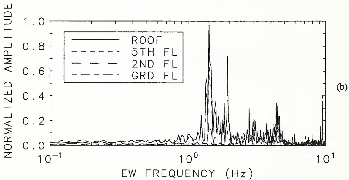
Figure 2.17 Normalized Fourier Spectra of Ambient Vibration Records at Different Elevations in NS (a) and EW (b) Directions, and First-Mode Response Mode Shape Due to Ambient Vibration (c).
