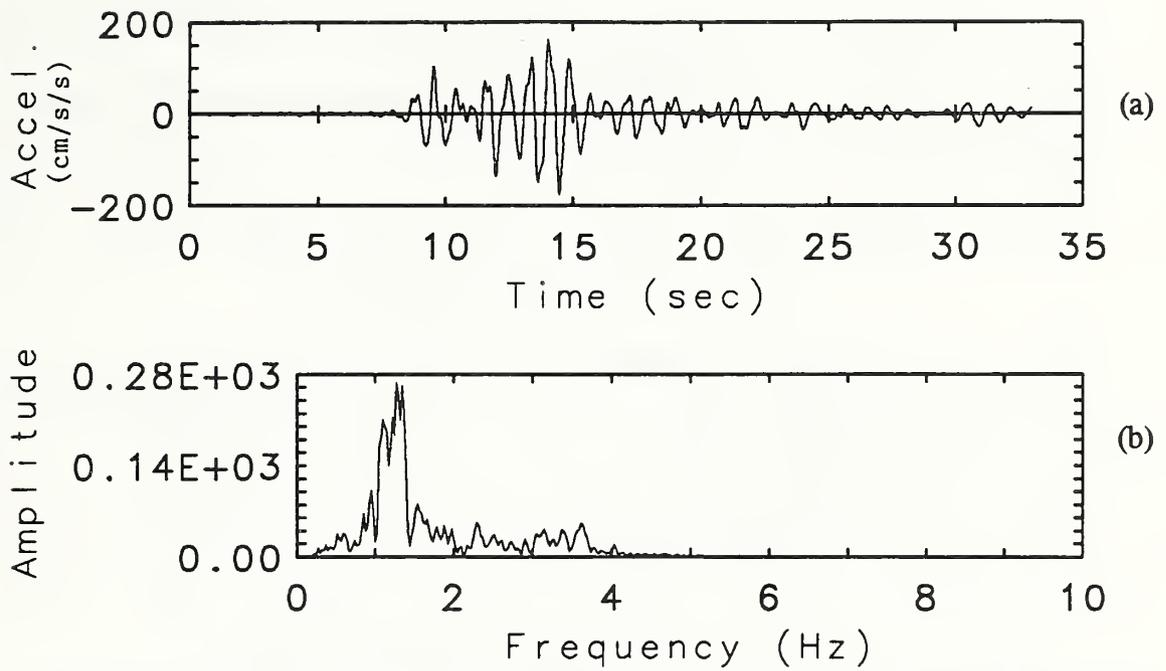
Figure 3.3 EW Acceleration-Time History at Center of Roof from the Fixed-Base Model with 10% Damping (a), and Corresponding Fourier Spectrum (b).
