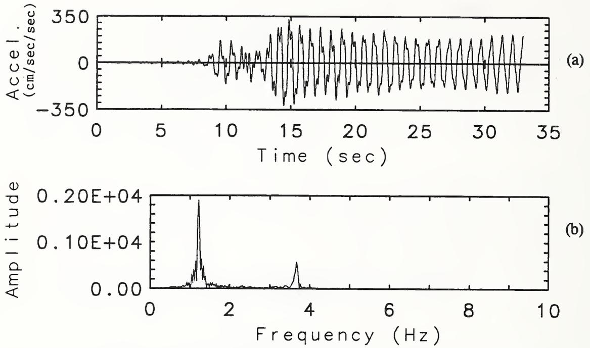
Figure 3.9 EW Acceleration-Time History at Center of Roof from the Fixed-Base Model with 0.5% Damping (a), and Corresponding Fourier Spectrum (b).
