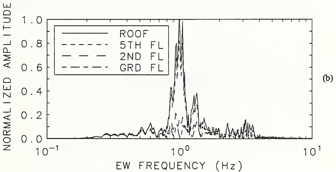
Figure 2.10 Normalized Fourier Spectra of Strong-motion Response Records at Different Elevation in NS (a), and EW (b) Directions, First-Mode Response Mode Shape due to the Loma Prieta Earthquake (c).
