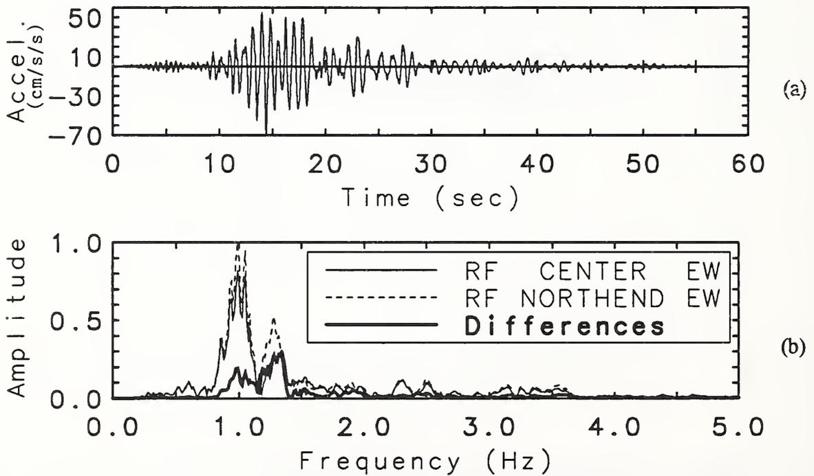
Figure 2.9 Difference of Roof-level EW Acceleration (a) and Corresponding Fourier Spectrum (b).
