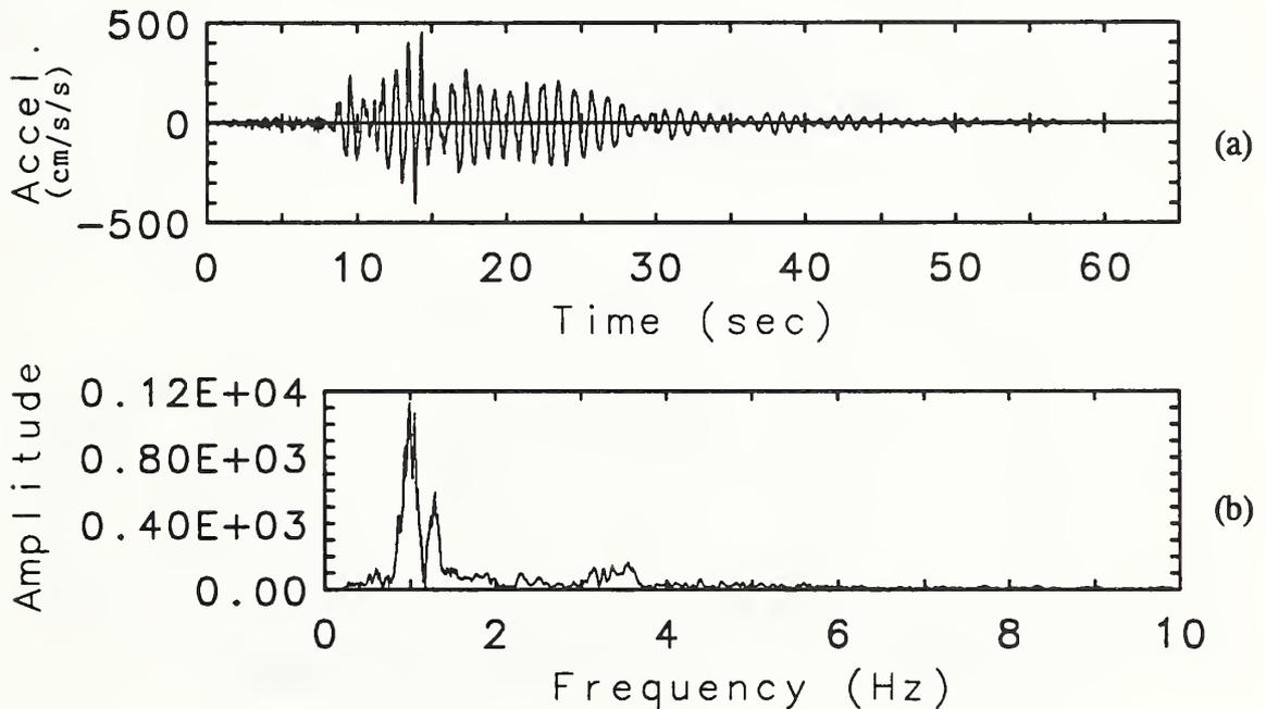
Figure 2.7 Acceleration-Time History at North end of Roof in EW Direction Due to the Loma Prieta Earthquake (a) and Corresponding Fourier Spectrum (b).
