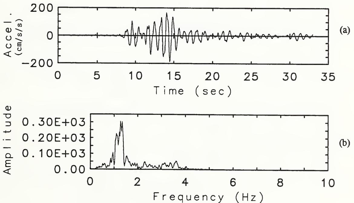
Figure 3.4 EW Acceleration-Time History at North End of Roof from the Fixed-Base Model with 10% Damping (a), and Corresponding Fourier Spectrum (b).
